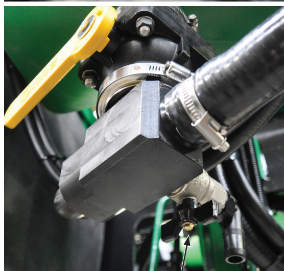
Hopper Drain Tap - Photo looking up from underneath the hopper
