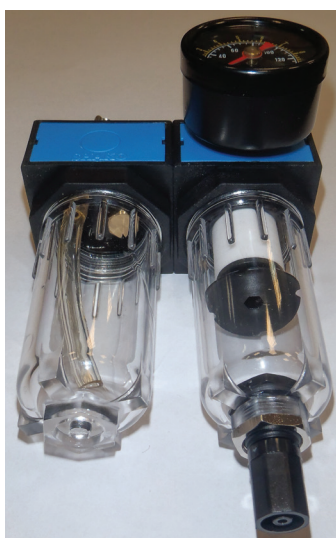
Moisture trap drain - Right chamber
