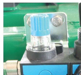
Oil flow adjustment screw - Blue
