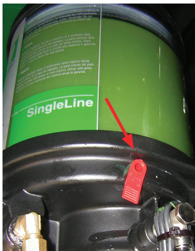
Figure 5. Red tagged bung in place.
