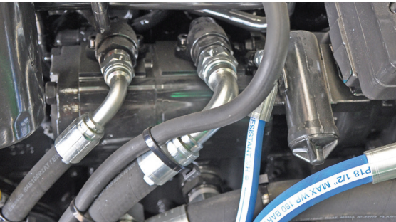
Above: Hydraulic pumps on left hand side of engine.
