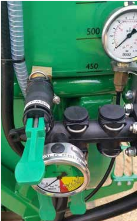
Picture 5 showing the bypass tap open for spraying.
