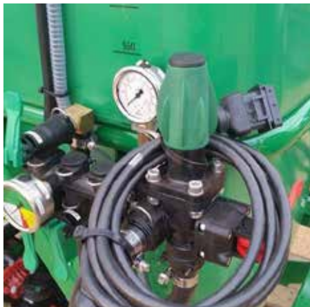
Picture 3, showing the control station. All taps are closed, and the dump valve is open providing low pressure agitation.
