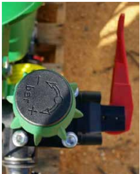
Picture 4, manual pressure regulator with directional indicators.
