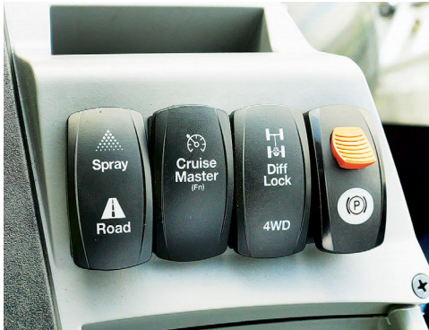
The Mode Switches panel (The Differential Lock Switch is a 4WD model option only).
