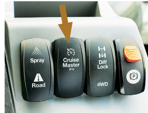
Press the top of the Cruise Master switch to activate or deactivate Cruise Control.
