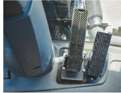
The Foot Brake (left) & Accelerator (right) located on the floor on the right hand side of the steering column.
