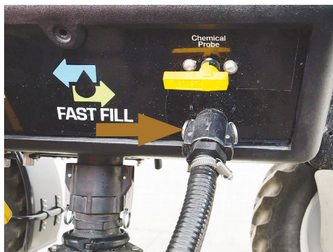
Connect a chemical probe suction hose to the Chemical Probe inlet.
