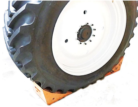
Chock opposite wheels of the Cruiser before lifting.
