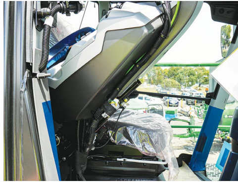
Lift & raise the front of the armrest control console to its highest position.
