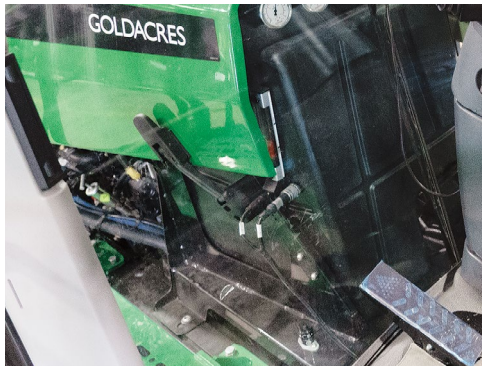
Unclip the bonnet latch located on the left hand side near the cabin.
