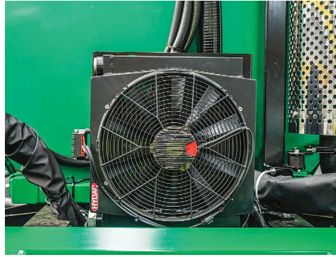
The Hydraulic Oil Cooler behind the spray tank
