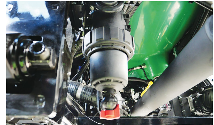
First remove the red valve at the base of the Pressure Filter, then unscrew the filter collar & remove the filter element for cleaning. After cleaning refit all components.
