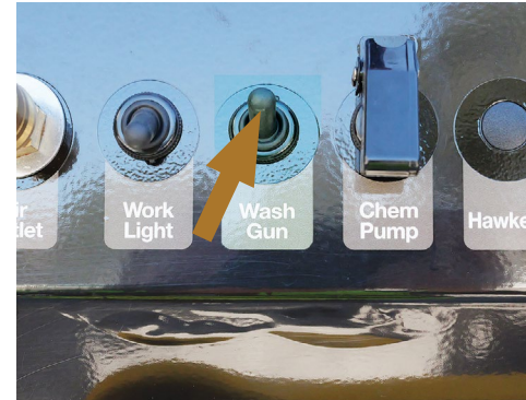
Lift up the 'Wash Gun' toggle switch On to start the pump.
