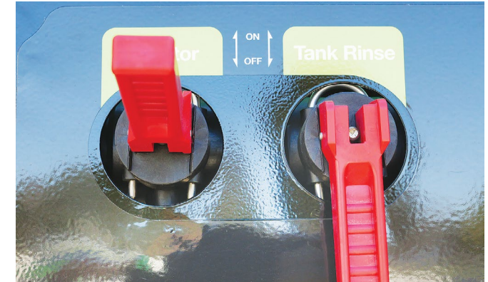
Raise the Agitator valve handle to 'On' position to rinse the tank agitator, then lower it to 'Off' position after rinsing.
