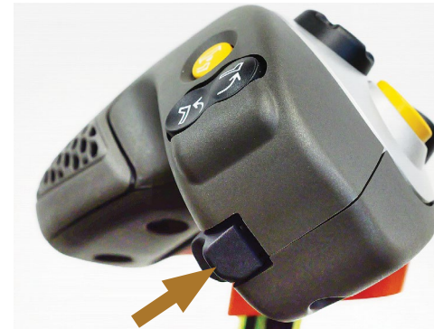
Dual Tilt rocker switch on the Joystick used to tilt boom wings up for folding.
