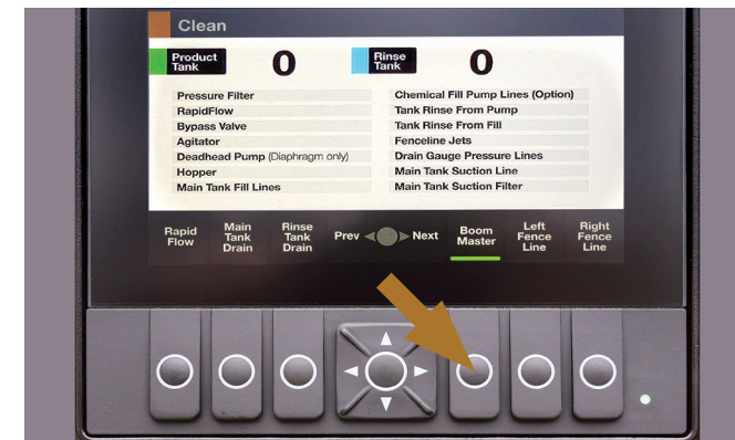
Press the 'Master Switch' push button 'On' to begin rinsing the boom nozzles.
