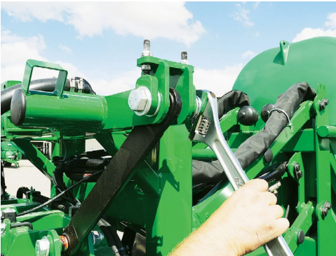
Loosen the bolt & nut clamping the top centre level support (on the centre section side the boom is low).
