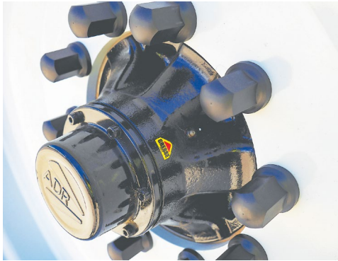
Recommended wheel nut torque tension is 320 ft/lb.
