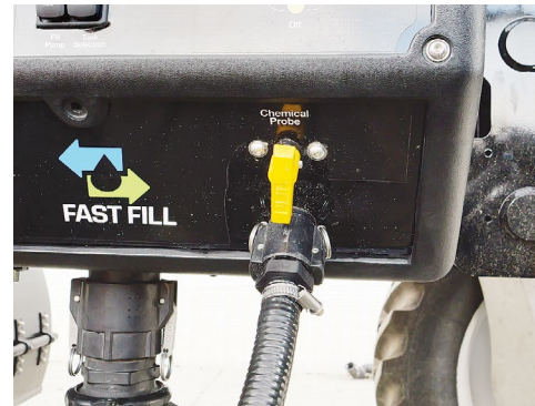
Rotate the 'Chemical Probe' valve to On position.
