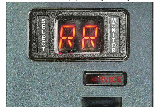
Select & Monitor displays showing Reverse gear.
