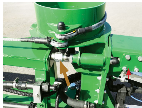
Stopper bolt used to adjust the 2nd boom section forward.
