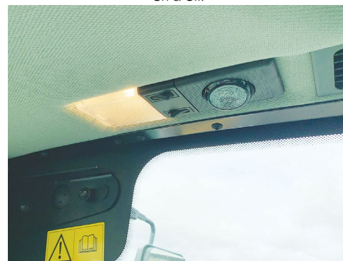
Use the Outer rocker switch to switch the front map light On & Off.
