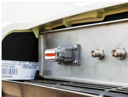
The cover removed showing the antenna connectors.
