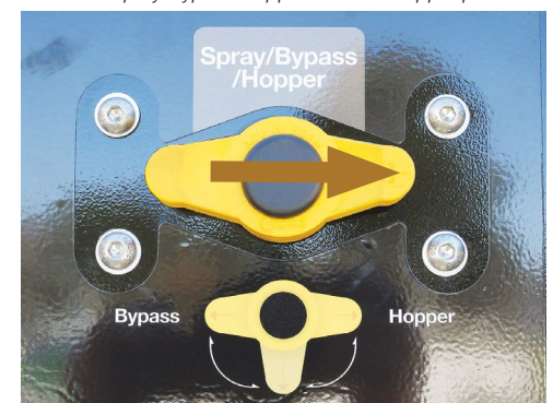
Turn the 'Spray/Bypass/Hopper' valve to Hopper position.
