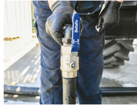
Place the Chemical Probe into the chemical & open the Probe Valve to rinse the hoses.
