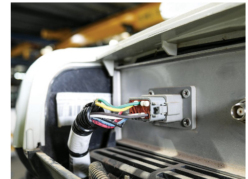
The Starfire adaptor cable fitted to the front connector.
