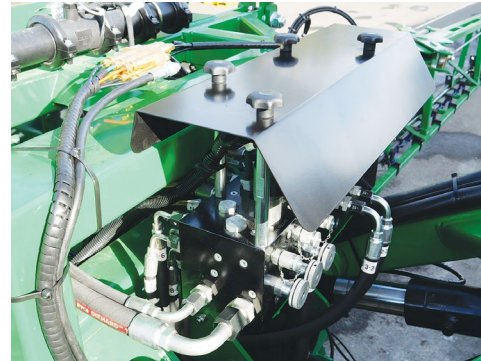
Remove the hydraulic manifold cover to access the Yaw reducing valve.
