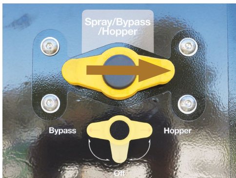
Turn the 'Spray/Bypass/Hopper' valve to Hopper position.
