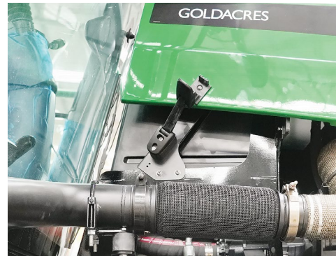
Unclip the bonnet latch located on the right hand side near the cabin.
