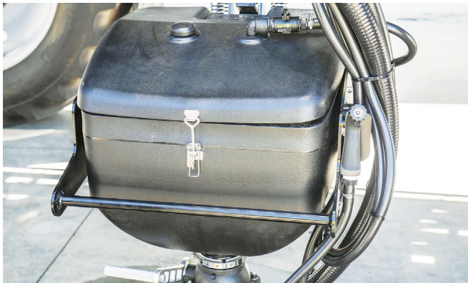
Lower the Chemical Induction Hopper keeping the hopper lid closed.
