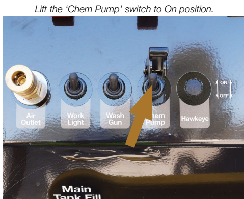
Lift the 'Chem Pump' switch to On position.
