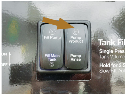
Press-in the 'Product Pump' switch to start the pump sourcing from the a Product tank.
