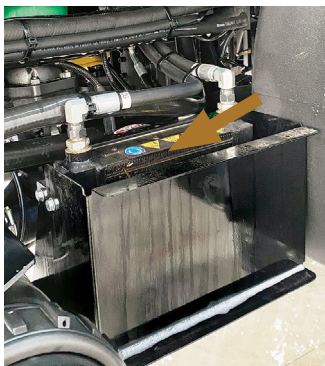
The transfer case oil cooler located on the RHS next to the suction filter.
