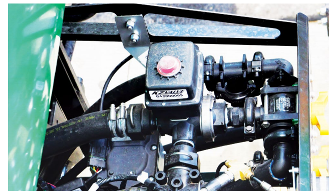
The Regulator Valve, located behind the Quick Fill panel, should regularly checked & calibrated.
