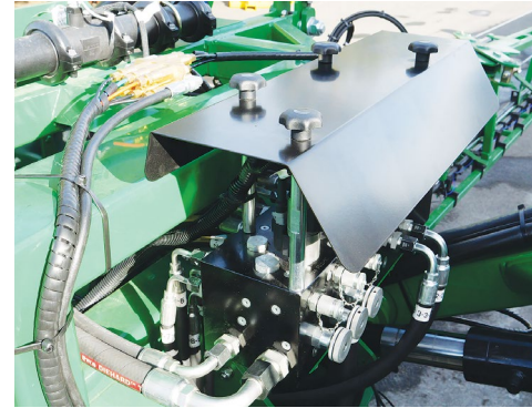
Rear Manifold at the front of the boom centre section.
