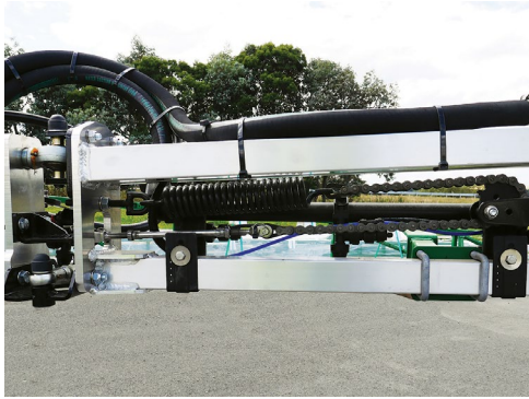
Regularly lubricate the Three Way Tip Breakaway mechanisms.
