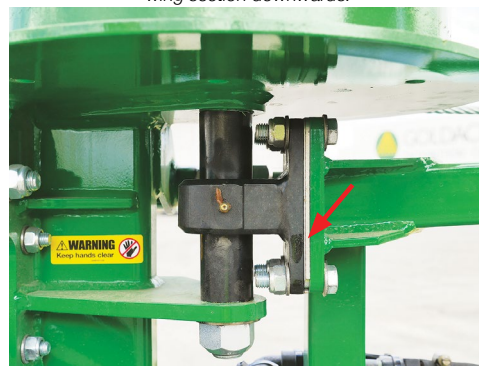
Add shims to the upper joint bracket to tilt the end of 2nd wing section downwards.
