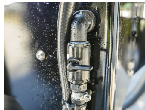
On completion of mixing, Close the Mixing Jet valve.
