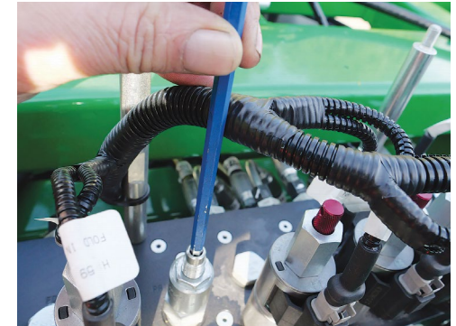
Set the Yaw Pressure with the Pressure Reducing Valve, then re-tighten the locknut.
