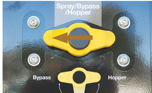
Rotate the 'Spray/Bypass/Hopper' valve to 'Bypass (Spray)' position for rinsing boom, tank and pump functions.
