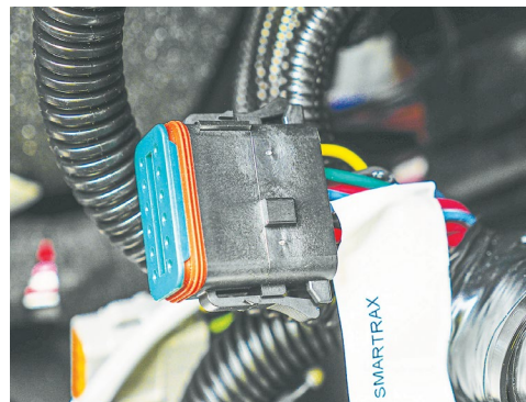
SMARTRAX connector - ISO BUS connection point.
