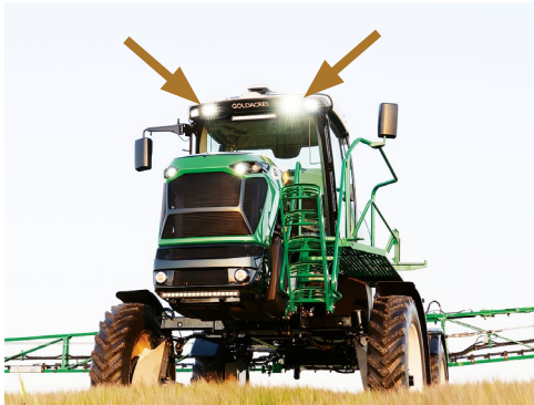
Two Egress lights on the front corners of the cabin provide exit safety in dark conditions.
