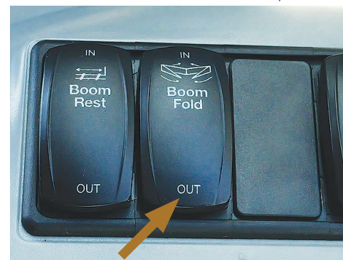
Press the 'Boom Fold OUT' button to build pressure.
