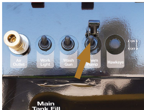
Lift the 'Chem Pump' switch to On position.
