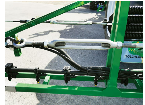
Eyebolt Cable Adjusters to tension the boom cables.
