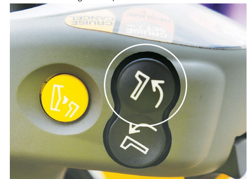
The upper Cruise Set/Increase push button used to resume current ground speed for Cruise Control.
