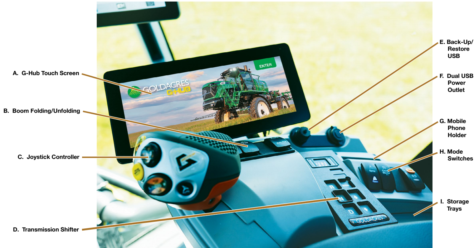
Armrest Control Console photo - information on each item (shown above) is given on the following pages using the item letter & title).
