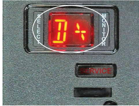
When the transmission shifter displays 'D-\' (loss of J1939), press 'D' and/or consult a qualified technician.
