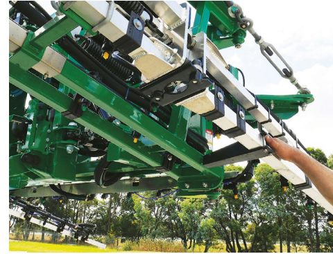
Check tension on the left hand folded outer boom section by pulling the end outwards.
