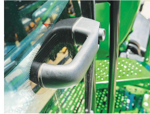
Use the cabin's external lockable door handle to open the cabin door.
