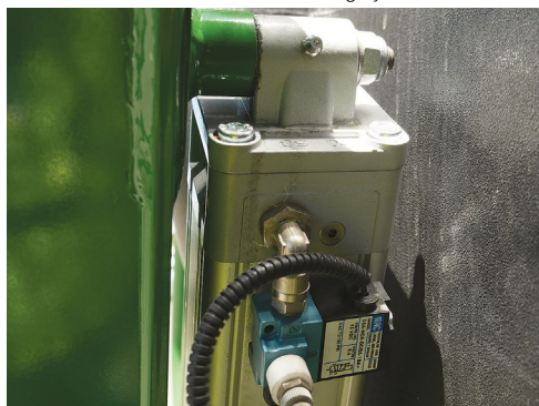
Air inlet of the ladder folding cylinder.
