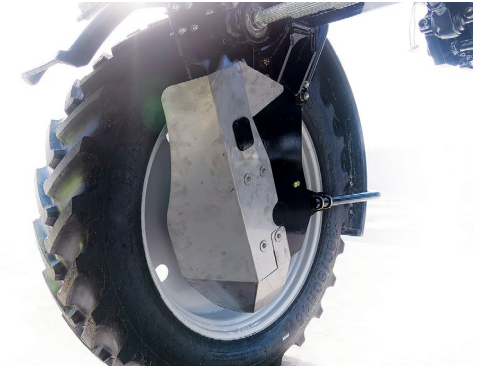
Check dropleg oil level.
