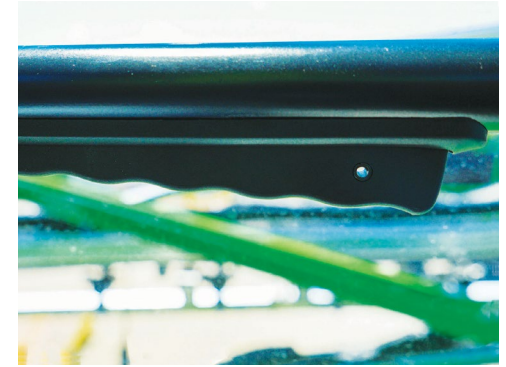
Squeeze the door handle lever to open the cabin door latch, then push the door handle to open the door.
