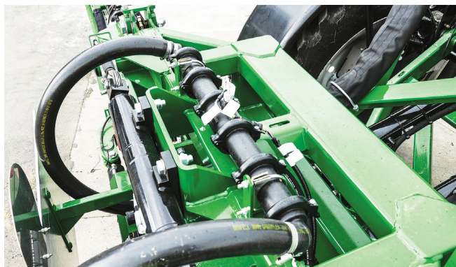
The Flow Meter, located on top of the boom centre section, should regularly inspected & cleaned.
