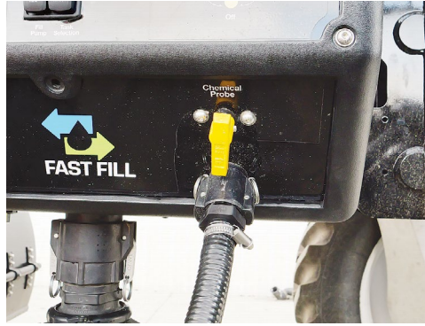
Connect the chemical probe suction hose to the Chemical Probe inlet & rotate the 'Chemical Probe' valve to On.
