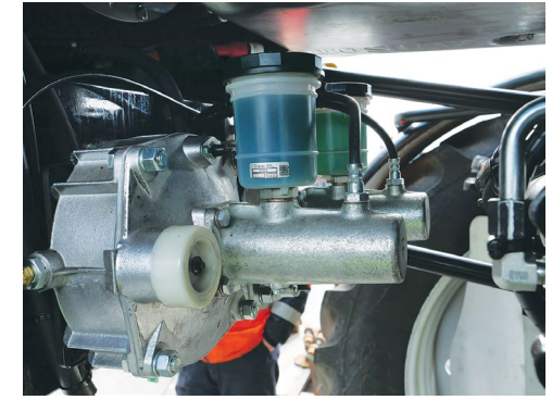
Brake fluid reservoirs located at the rear of the engine.
