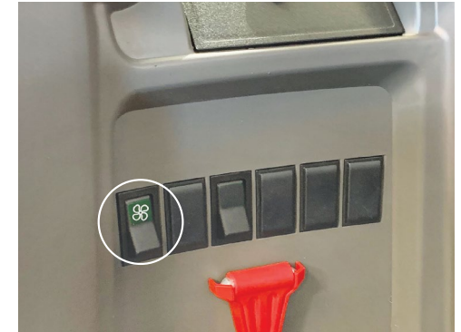
Press the Carbon Filtration Fan Rocker Switch to activate the Carbon Filtration System Fan before spraying.
