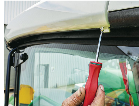
Remove the screws from the antenna connectors cover.
