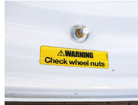
Check tyre inflation and wheel nuts.
