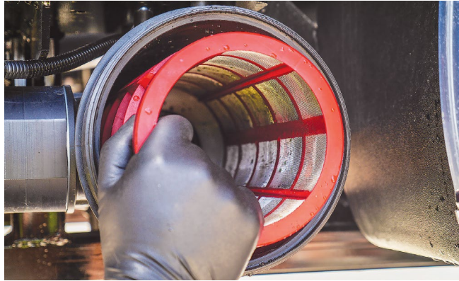
Remove the Suction Filter screen.
