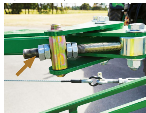
Adjuster bolt used to adjust the 1st boom section forward.
