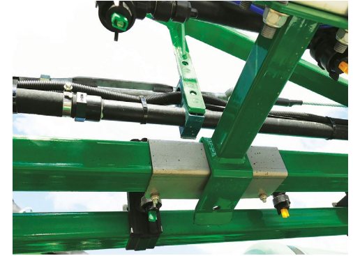
The outer boom rest protection plate must be correctly positioned on each side.
