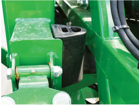
Check rubber bumpers for wear. Replace if worn.
