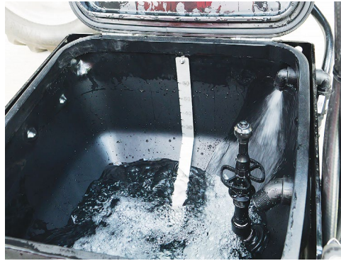
Add the chemical granules or powder to the flowing liquid.
