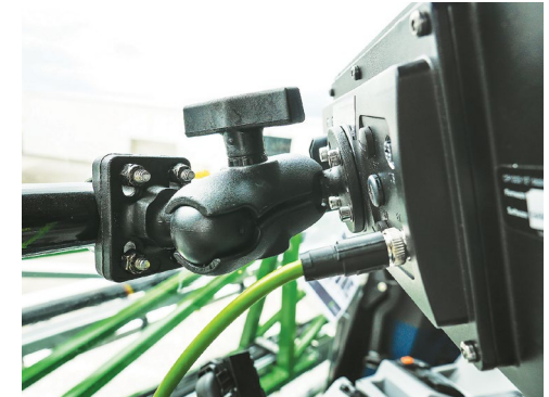
Position the ball mount on the cabin rail & fit the G-Hub Console & cables.
