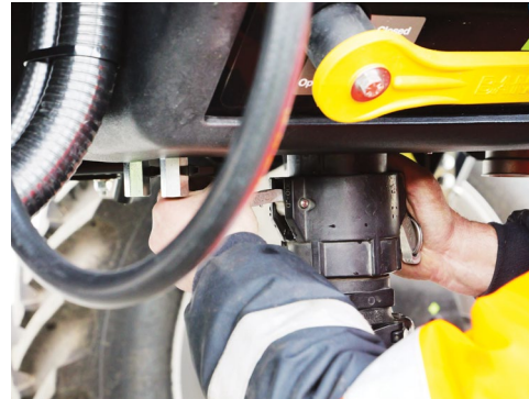
Connect a 3" fill hose to the 'Clean Fill' inlet & Open the 'Fill' ball valve(s).
