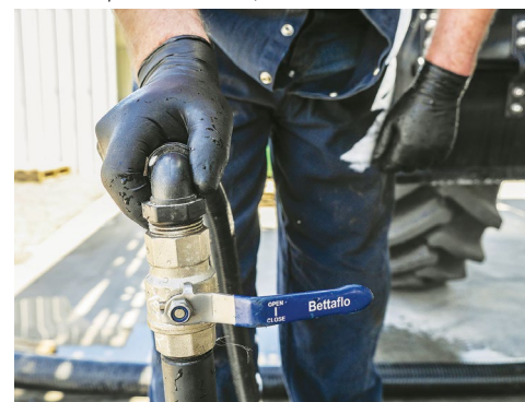
After the required amount of chemical has been transferred lift the probe to suck air, then close the Probe Valve.
