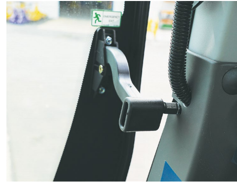
The right hand door latch opened with the holding pin & latch holding the door ajar.
