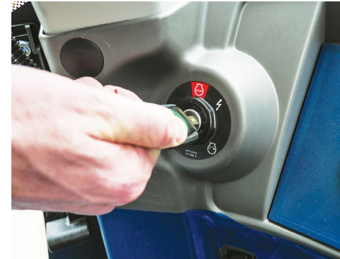
Turn the Ignition key to crank & start the engine.
