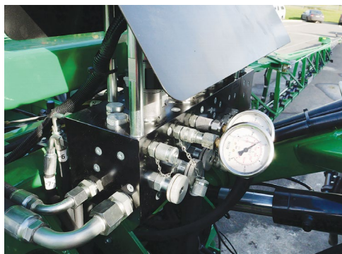
Relocate pressure gauges from the hydraulic cylinder circuit to the hydraulic control block
