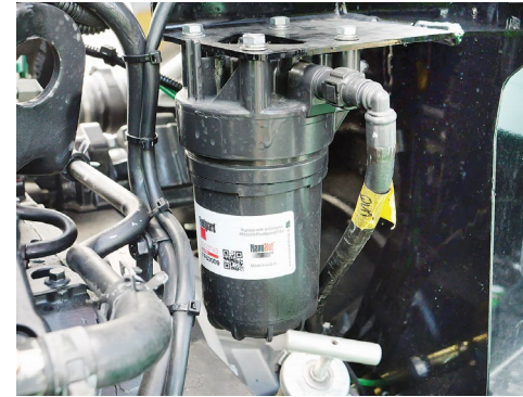
The secondary fuel filter located on the left hand side of the engine.
