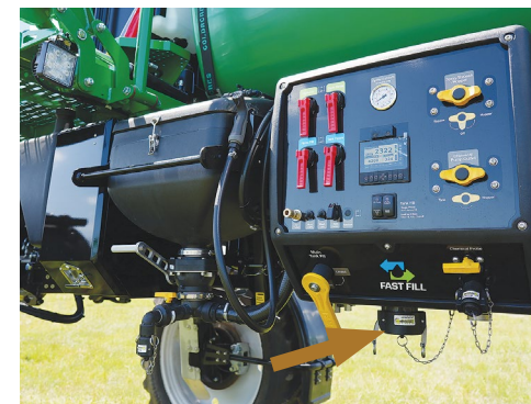
The 3" Clean Fill inlet located underneath the filling pod with camlock cap fitted.
