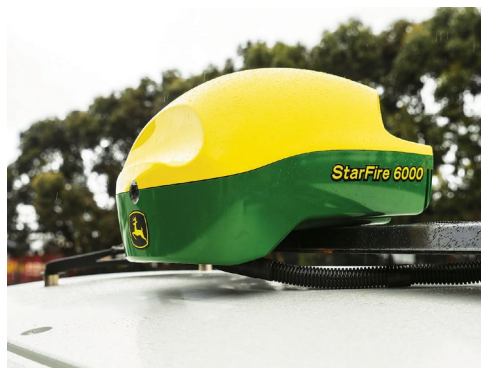
Fit & connect the Starfire Receiver onto the roof mounting.
