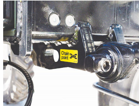
Front right tie-down attachment & towing point.
