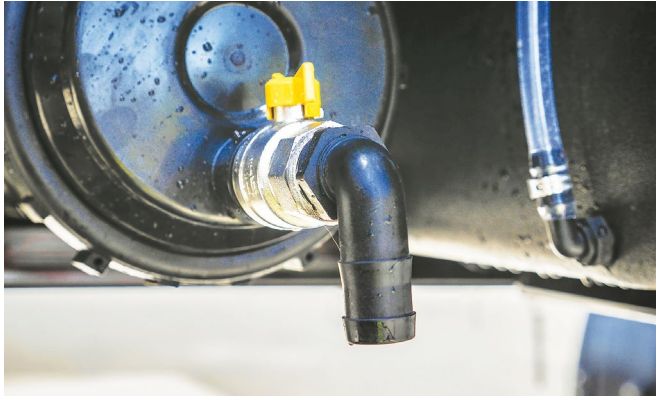
Open the drain valve to drain the Suction Filter.
