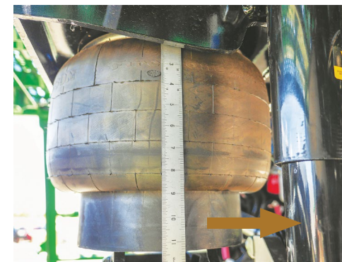
Air bag ride height measurement & shock absorber (right).
