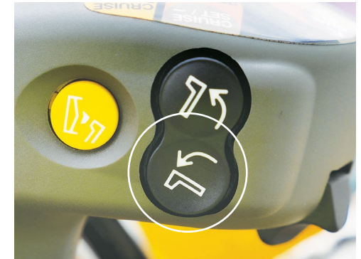
The lower Cruise Set/Decrease push button used to set the current ground speed for Cruise Control.
