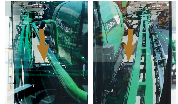
Rear vision mirror views of rear axles fully closed.
