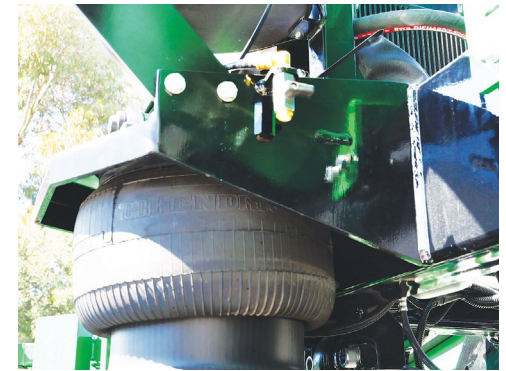
Airbag component of the 5 point suspension system.
