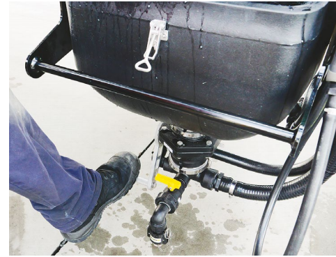
Open the foot operated ball valve at the base of the Hopper to transfer mixed product into the Main Tank.
