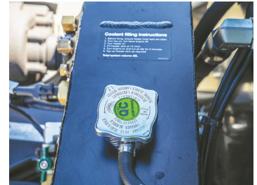
The engine radiator & radiator cap.
