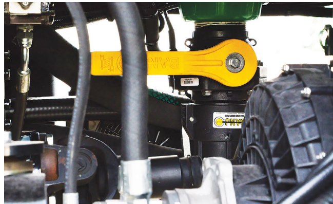
Open the Product Tank drain valve by rotating down the yellow handle down & completely drain the tank. Close the drain valve when emptied.
