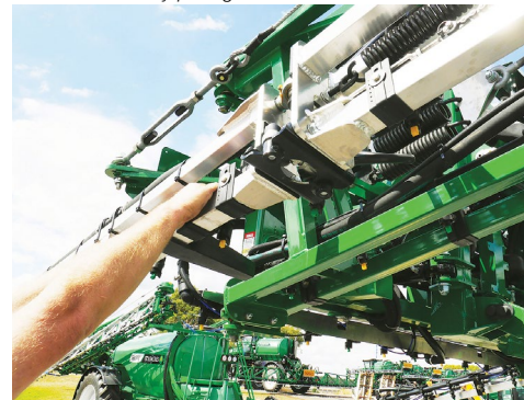
Check tension on the right hand folded outer boom section by pulling the end outwards.
