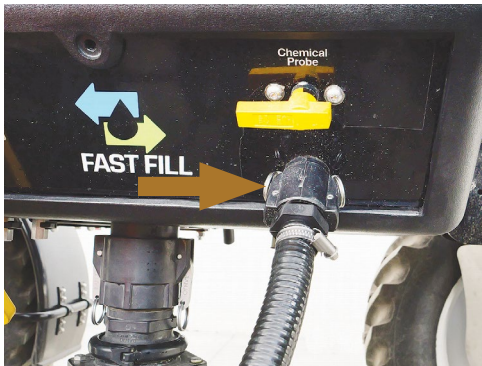
Connect a Micromatic suction hose to the Chemical Probe inlet.
