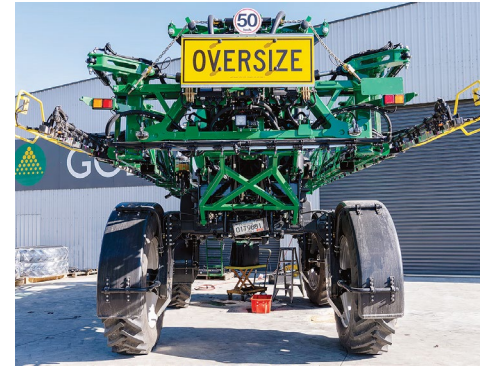
From behind the sprayer, watch if one side of the boom tilts excessively downwards when folding.
