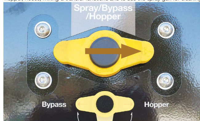
Rotate the 'Spray/Bypass/Hopper' valve to 'Hopper' position for rinsing the hopper, hoses, mixing & transfer functions and to use the spray gun for cleaning.
