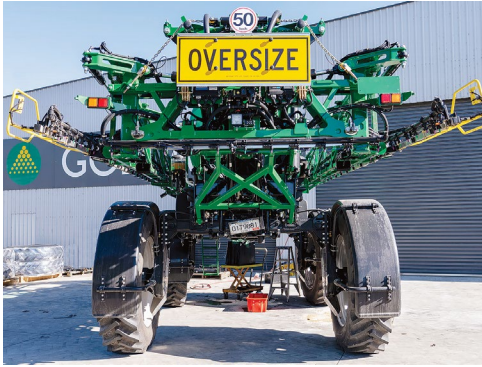
Fold the boom to re-check boom alignment in the folded position.
