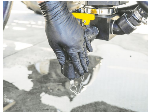
On completionm disconnect the micromatic hose & refit the camlock coupling plug.
