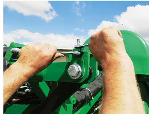
Undo the adjuster locknuts and adjust the support to raise & level the boom. After adjustment retighten the locknuts.
