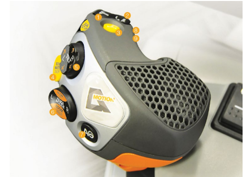
Check all joystick boom switch functions.
