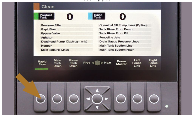
Press the 'Rapid Flow' push button On (illuminates green when On) to rinse the boom pipes.
