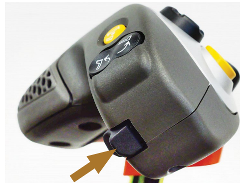
Press & hold IN the outer end of the Dual Tilt rocker switch on the Joystick to raise the boom wing ends.
