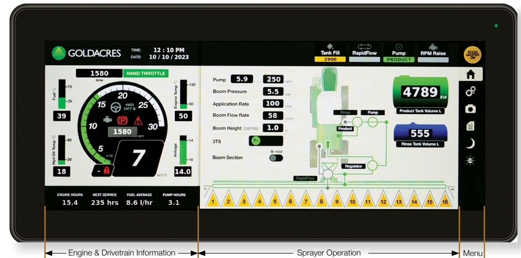
Goldacres G-Hub Touch Screen illustrating three sections of touch control & data information.
