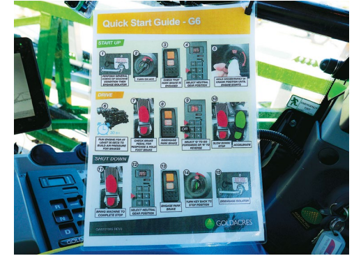
The plastic coated Quick Start Guide attached to the right hand safety door rail of the cabin
