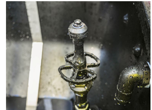
Open the hopper lid to access the Drum Rinse Nozzle.
