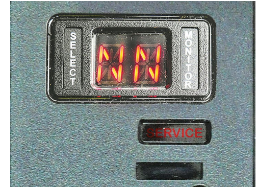
Select & Monitor displays showing Neutral.
