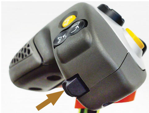
Press & hold IN the inner end of the Dual Tilt rocker switch on the Joystick to lower the boom wing ends.
