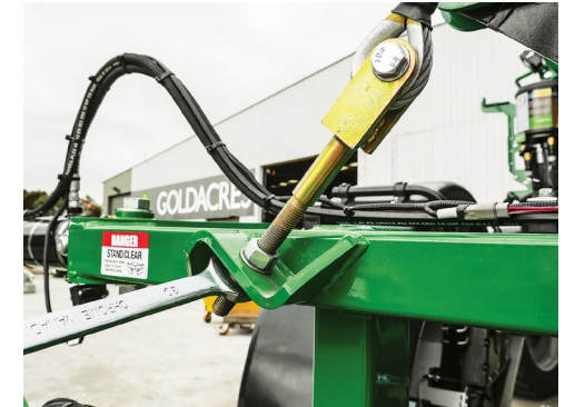
Make adjustment to the Boom Centre Level cable adjusters as required.
