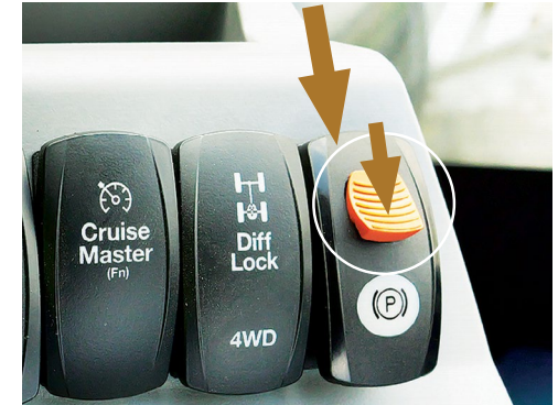
To engage the Park Brake (On), slide the orange lock rearward & press the top of the switch.
