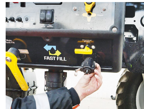
Rotate the Chemical Probe valve to Off. Disconnect the hose from the Probe Inlet & replace the camlock cap.
