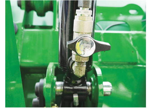
Close the ball valve on each lift cylinder (2) for safety.
