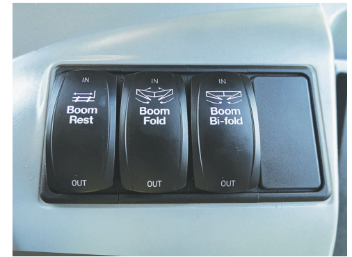
Boom Rest, Boom Fold & Boom Bi-fold rocker switches used for folding & unfolding the boom.
