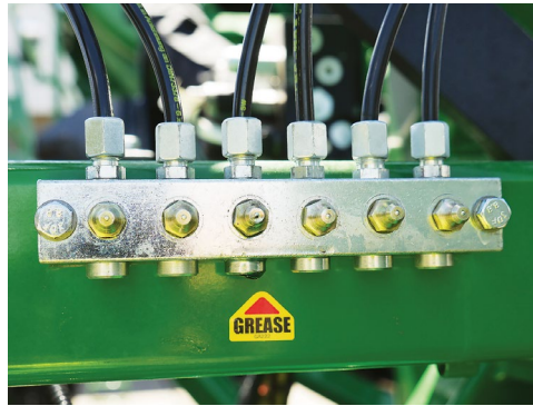
'Remote Grease Bank' with a 'Grease Decal' are used to simplify greasing access.
