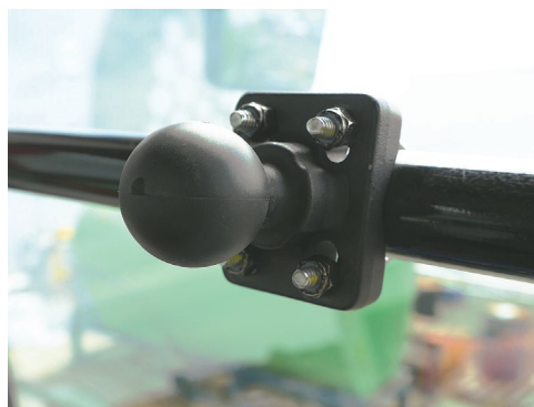
Ball mount fitted on the rail ready for the Autosteering Console.
