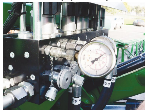
Use the Yaw Pressure gauge when setting Yaw pressure.
