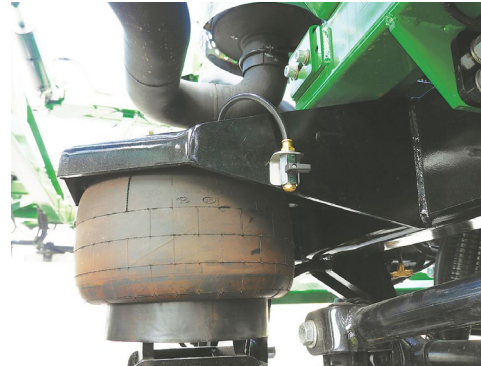
Open the dump valve air bag for trailer transport.
