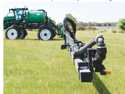
Move the boom end by hand to adjust the Yaw Alignment.
