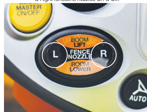
The Fenceline Nozzle push button is used to switch the Left & Right fenceline nozzles On & Off.
