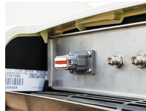
The cover removed showing the antenna connectors.
