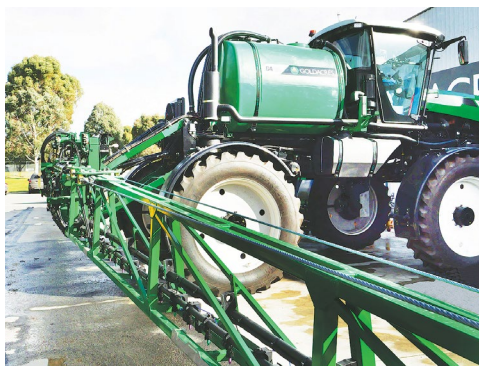
On level ground, engage the park brake, chock wheels & have the boom in working position before making adjustments.
