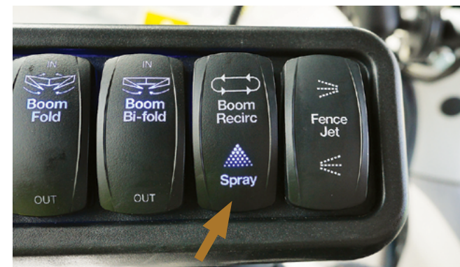
Start the 'Product Pump', then press 'Spray' to start the nozzles spraying.
