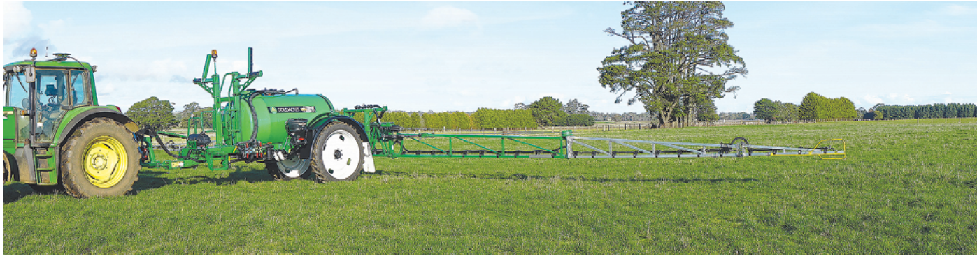
3000 litre Prairie Special fitted with 24m Delta boom & Rowcrop 3 point linkage hitch option.
