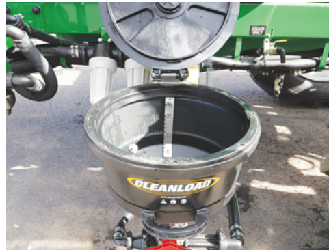
Lower Chemical Mixing Hopper & open the lid to add an appropriate amount of decontaminating agent.
