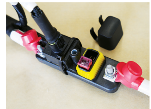
The main fuse of the electrical system with cover removed.
