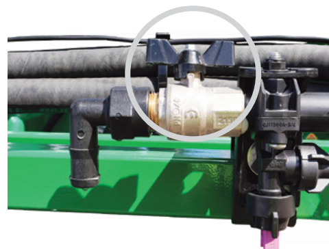
Open each boom section valve to quickly flush chemical from the boom line.
