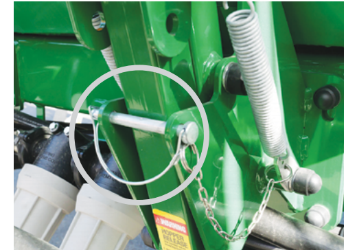
To lower the Chemical Induction Hopper, first remove the hopper safety pin & locking pin.
