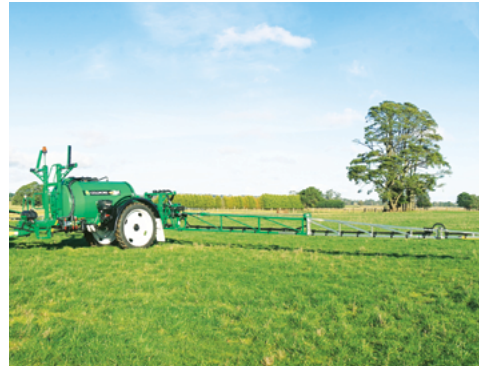
On level ground, engage tractor park brake, chock wheels & place boom in working position before making adjustments.
