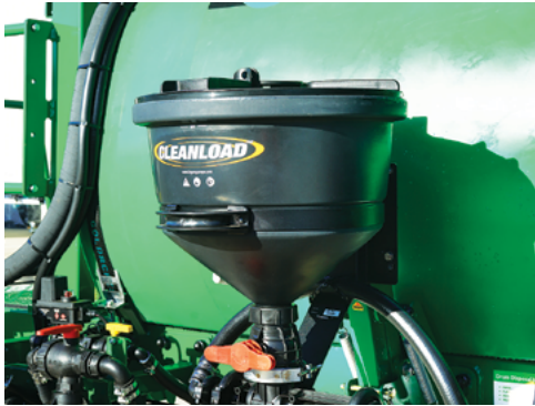
Raise the Chemical Induction Hopper to transport position.
