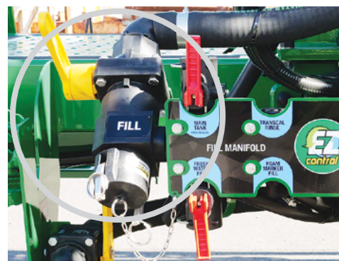
The 2" Clean Fill inlet with camlock cap fitted.
