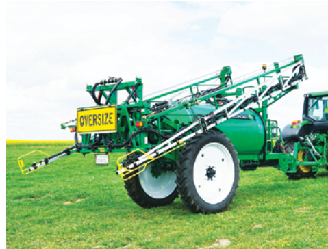
3000 litre Prairie special with 3 point linkage hitch & 24m boom
