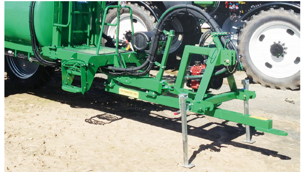
A detachable drawbar is bolted to the base optional Rowcrop Hitch to enable vehicle transport without 3 point linkage arms. The detachable drawbar must be removed before connecting the sprayer to the tractor 3 point linkage arms.
