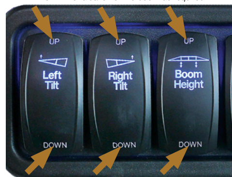
Press 'Left Tilt UP DOWN' & 'Right Tilt UP' switches to raise lower boom ends as needed & press 'Boom Height UP/DOWN' to raise/lower the boom as required.
