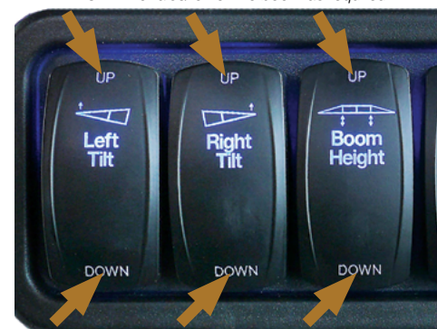
Press 'Left Tilt UP DOWN' & 'Right Tilt UP' switches to raise lower boom ends as needed & press 'Boom Height UP/ DOWN' to raise/lower the boom as required.
