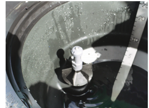
Hopper Drum Rinse Nozzle.
