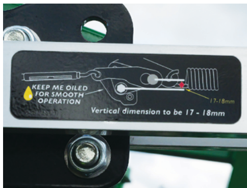
End boom section lubrication points.
