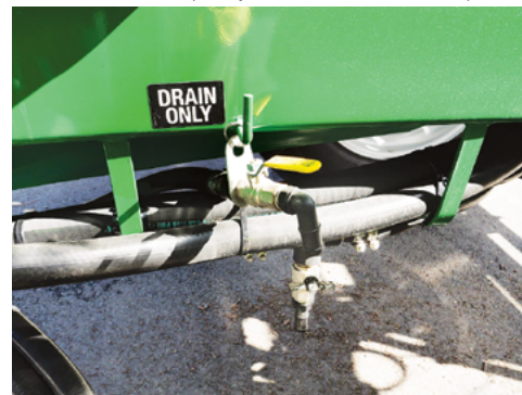
Unhook the 'Sump Hose Drain Valve', open the valve & lower it, to completely drain the Main Tank sump.
