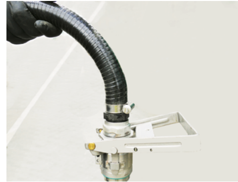
Disconnect the Micromatic coupler from the chemical source.
