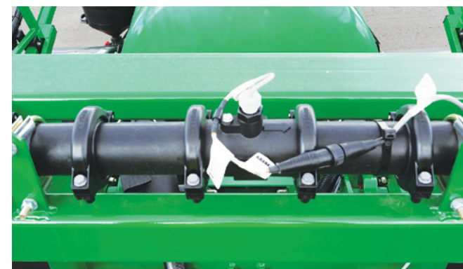
The Flow Meter, located on top of the boom centre section, should regularly checked & cleaned.
