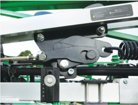
Regularly lubricate the 3-Way Breakaway mechanism.
