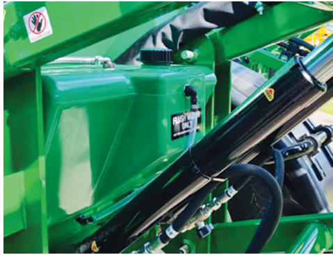
The Rinse Tank (200 litres) must be filled with clean water to do the Quick Boom Rinse.
