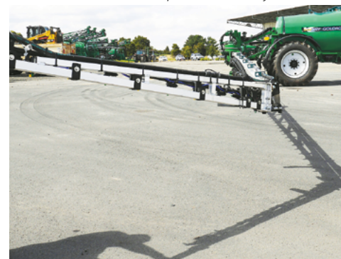
Rearward & Upward Breakaway.
