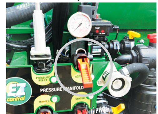
Open the 'Agitator' valve (located on the Pressure Manifold) to ensure chemical agitation in the Main tank.
