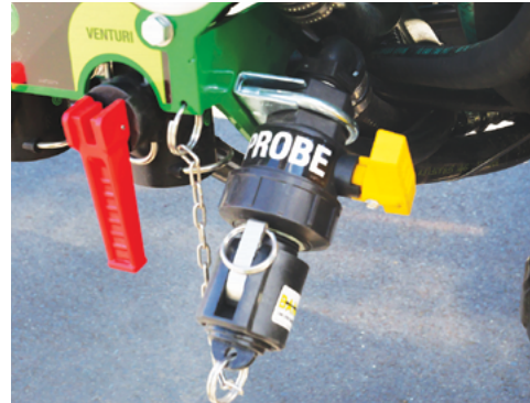
Chemical Probe Inlet with Camlock cap fitted on the right hand side of the Pressure Manifold.
