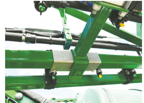
Ensure outside boom saddles slide over inside boom protection plates for support in folded position.
