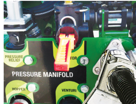
Connect the Micromatic coupler to the Micromatic Rinse Coupling on the Pressure Manifold of the sprayer.
