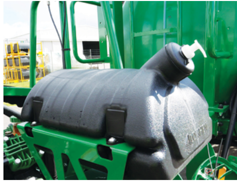
Hand Rinse Tank (20 litres) located at the front of the sprayer - clean water only cleansing.
