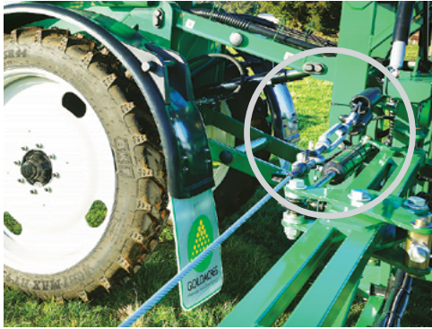
Turnbuckle cable adjuster used to tension each boom cable.
