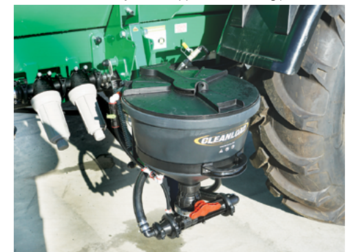
Use the hopper handle to support the hopper, unlock the latch lever, then carefully lower hopper to its working position.
