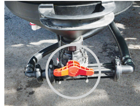
Open the 'Transfer' valve (at the base of the hopper) to transfer chemical mixture to the Main tank.
