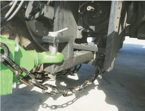
Ensure the drawbar pin & safety chains are fitted and locked in position.
