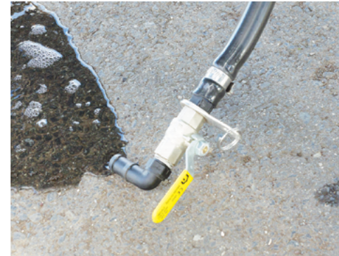
Open the 'Sump Hose Drain Valve', & lower it to completely drain the Main Tank sump.
