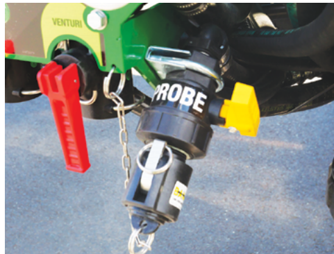
Close the Venturi valve and Chemical Probe Inlet valve, then disconnect the Probe 1" hose & refit Camlock cap.
