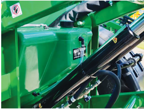
Rinse Tank (200 litres) located at the rear of the sprayer - clean water only for flushing the sprayer.
