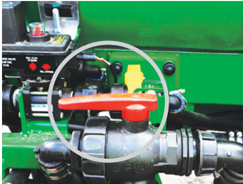
Turn the Three-way Red Handle ball valve (top of the suction filter) to draw liquid from the Main tank (arrow pointing forwards).
