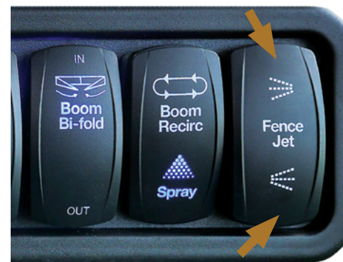
Press the 'Fence Jet' switch to start & stop fenceline nozzle spraying as required.
