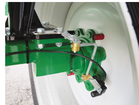
Wheel speed sensor & magnets are fitted to the right hand side sprayer wheel.
