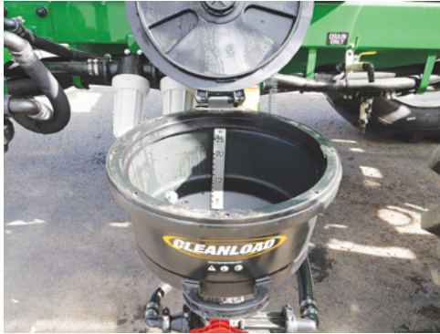
Release the hopper lid latch & open the lid.
