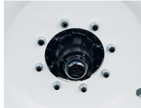
Recommended wheel nut torque tension is 320 ft/lb.
