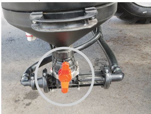
Close the 'Transfer' valve (at the base of the hopper) on completion of transfer to the Main tank.
