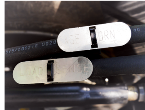
Each hydraulic hose is tagged for easy recognition - CASE DRN & LOAD SENSE hose tags shown above.
