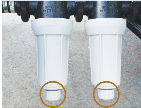
Unscrew and remove the end caps from each filter and allow liquid to drain out.
