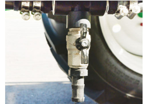
To empty the Rinse Tank, open the drain valve on the LHS of the sprayer and allow the water to drain out.
