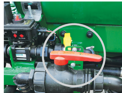
Turn 'Bypass' valve to Off & the Three-way Red Handle ball valve to draw from the Rinse tank
