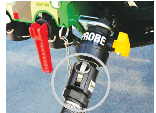
Remove the Camlock cap and connect a Chemical Probe hose to the 1" Chemical Probe Inlet.
