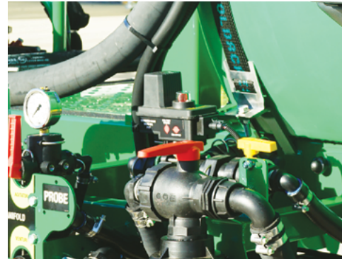
Rotate the 'Three-way Red Handle' ball valve (top of filter)' to Off position to close-off any liquid from the Main Tank.
