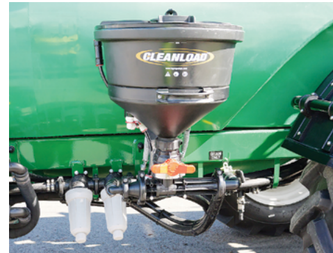
Chemical Induction Hopper in raised/transport position.
