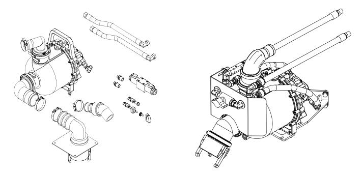
Description: This kit includes a hydraulic drive centrifuge pump with a 3" inlet and a hydraulic spool valve to assist with the filling of the main tank on a machine without having the need to transport a separate pumping unit. Flow of unit is approximately 350 - 400LT/Min.
