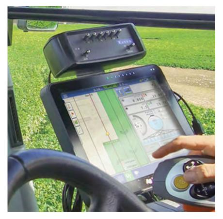
Description: ISOBUS Product Control and ISOBUS CAN System, The Raven ISOBUS single product control node is designed to add liquid speed compensated product control capabilities to ISOBUS virtual terminals.
