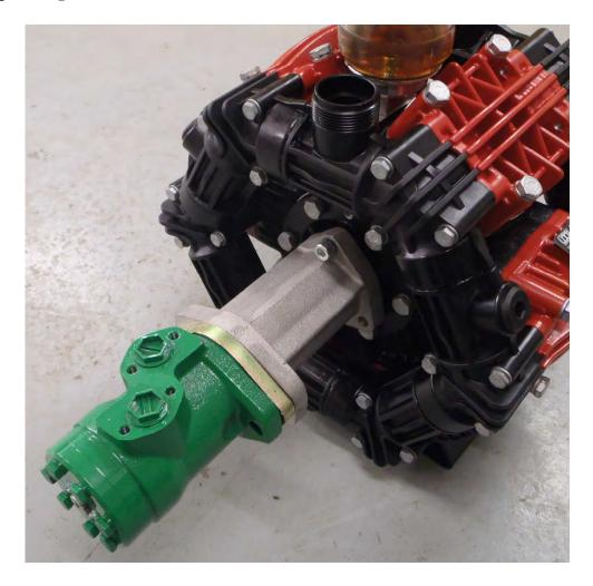
Description: This kit has been produced to remove the PTO shaft from the tractor and use the hydraulics from the tractor to drive the PTO Pump.
