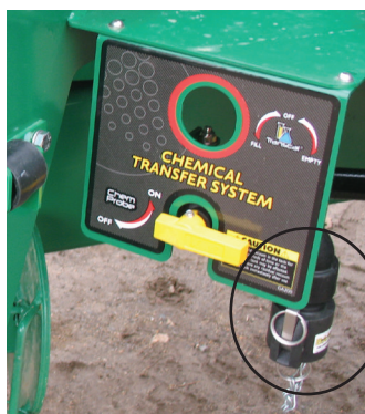
Chemical Probe connection point
