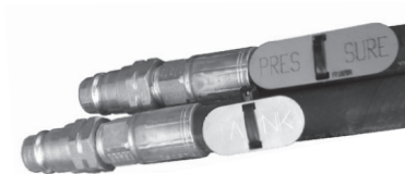
Hydraulic hose connections
