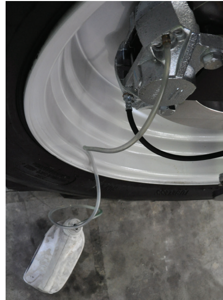
Left: Front brake caliper bleeding setup
