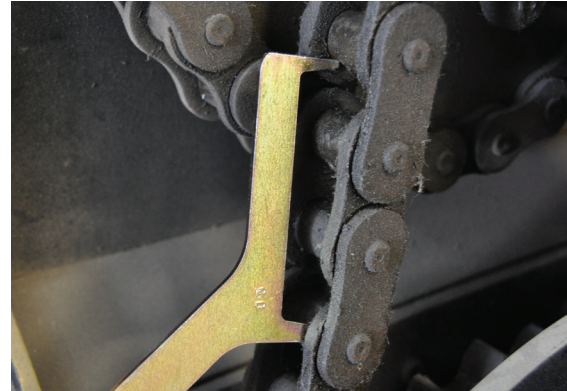
Above: Chain gauge being used to assess chain stretch percentage.
