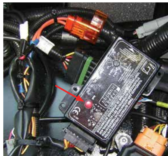
Figure 10. Electronic timer in main fuse compartment
