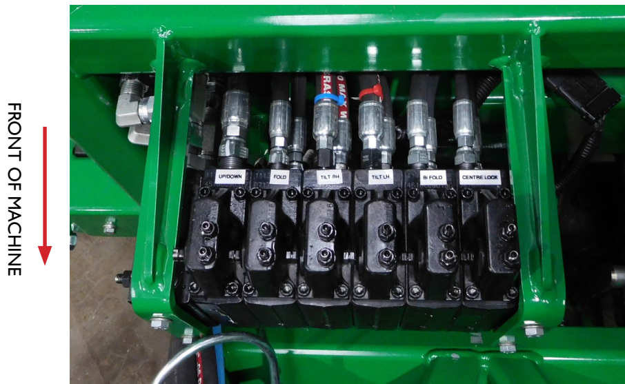
Above: The hydraulic boom functions are controlled by an electric over hydraulic solenoid valve block mounted to the paralift rear of the centre section.
