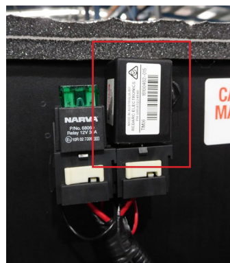
Above: Egress lighting timer relay located in rear left hand side roof area of cabin.
