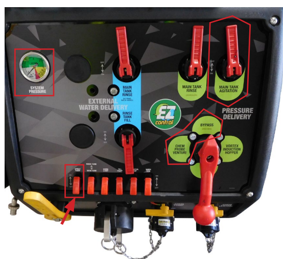
Above: EZ control pod functions used when transferring chemical via the venturi method.
