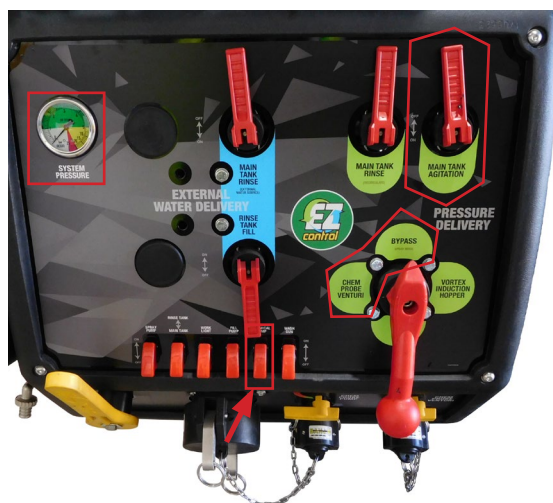
Above: EZ control pod functions used when transferring chemical via the electric pump method.
