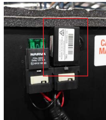
Above: Egress lighting timer relay located in rear left hand side roof area of cabin.
