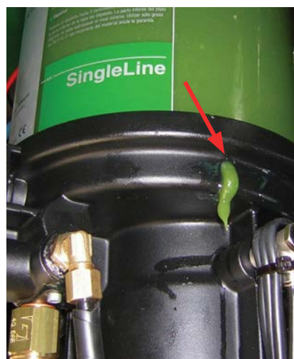
Unplugged overflow hole
