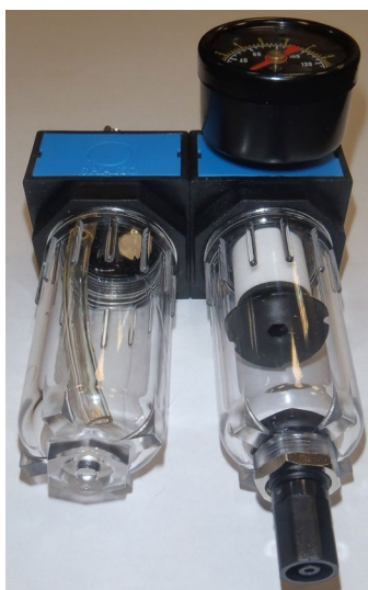
Moisture trap drain - Right chamber
