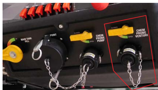
Above: Chemical probe venturi cam lock fitting and isolating ball valve.
