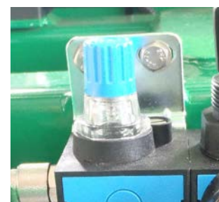
Oil flow adjustment screw - Blue
