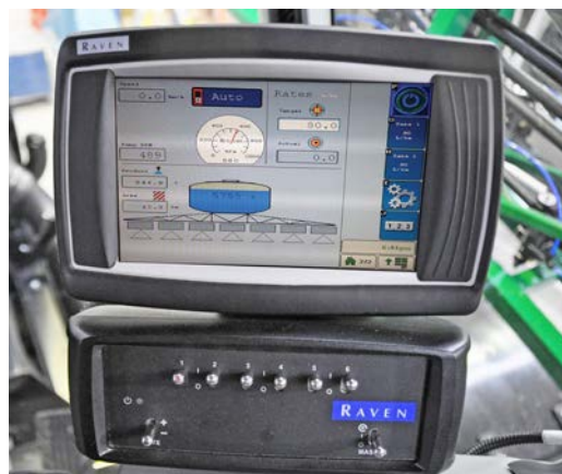
Above: ISOBUS system with Raven virtual terminal (VT) screen and 6 section switch box.
