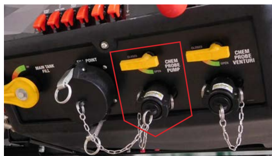
Above: Chemical probe pump cam lock fitting and isolating ball valve.
