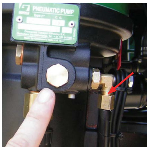
Above: Second grease outlet
