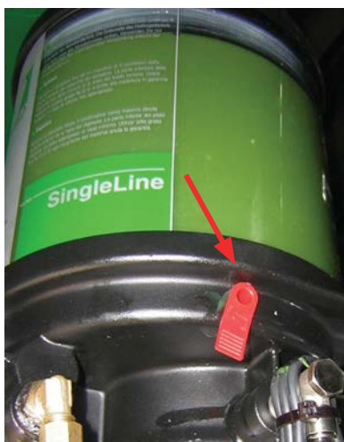
Red tag bung must be removed
