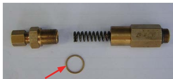
Meter components showing shim
