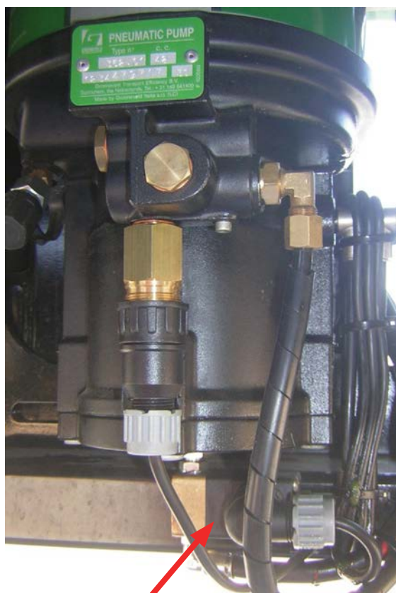
Solenoid located at bottom of pump unit
