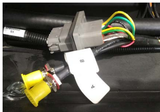
Above: GPS receiver connection points inside the cabin roof near the front, on the left hand side.
