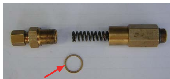
Meter components showing shim
