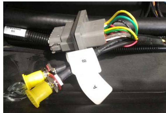
Above: GPS receiver connection points inside the cabin roof near the front, on the left hand side.
