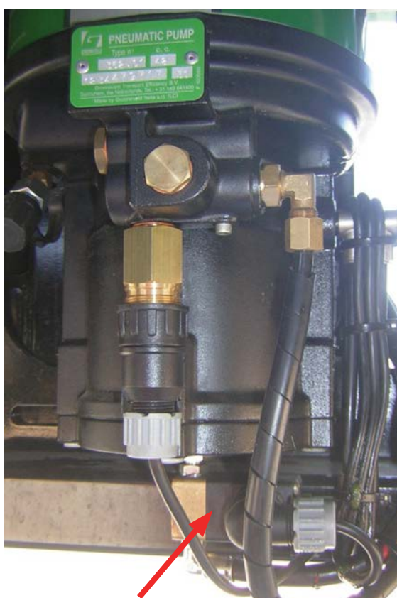
Solenoid located at bottom of pump unit
