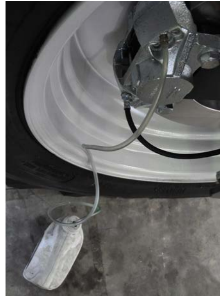
Left: Front brake caliper bleeding setup
