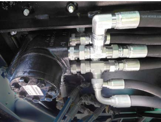
Above: Steering orbital mounted under cabin.
