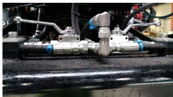
Above: Adjustable axle isolating taps on top of axle.
