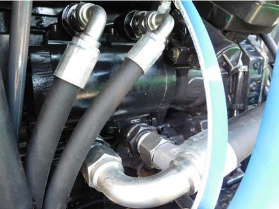
Above: Hydraulic pumps on left hand side of engine.
