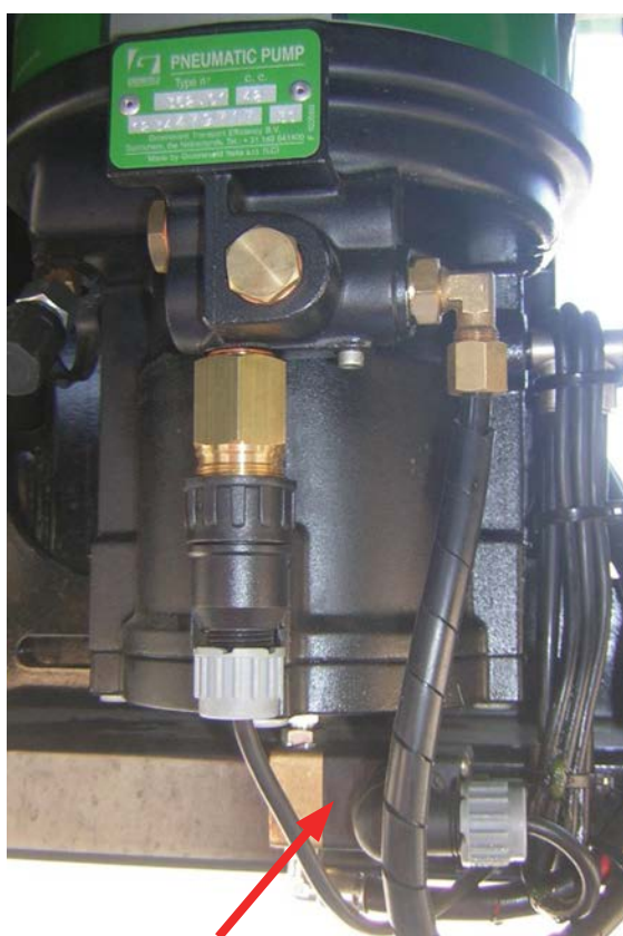
Solenoid located at bottom of pump unit
