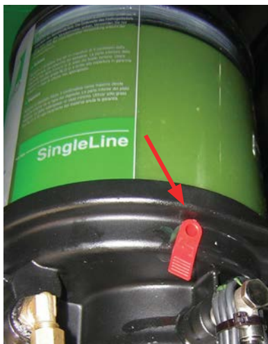
Red tag bung must be removed
