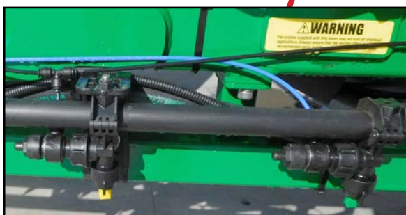
Air check nozzle bodies arranged along centre section and booms
