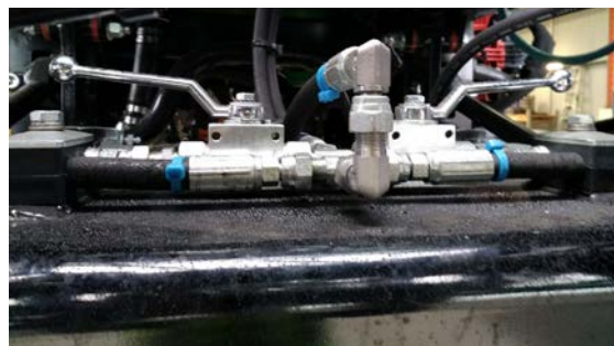
Above: Adjustable axle isolating taps on top of axle.
