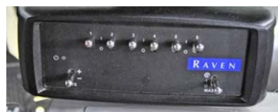
Above: An optional Raven 6 section control box can be programmed to control the 16 sections in any combination of groups or individually. Note that Raven RCM and Rapidfire must be optioned for 16 section booms.
