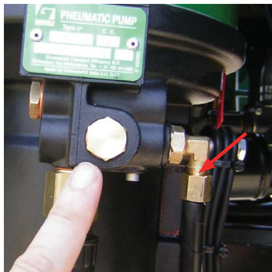
Above: Second grease outlet
