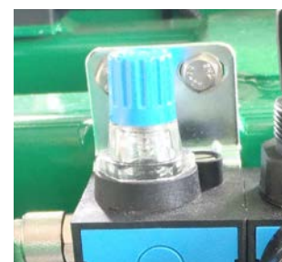
Oil flow adjustment screw - Blue
