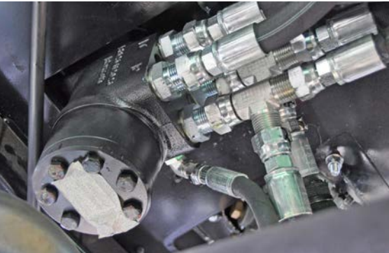
Above: Steering orbital mounted under cabin.
