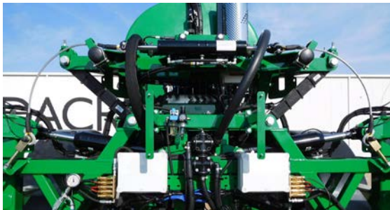
Above: Centre levelling system - holds booms level when folding.
