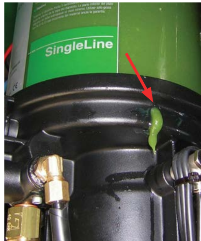
Figure 6. Unplugged overflow hole
