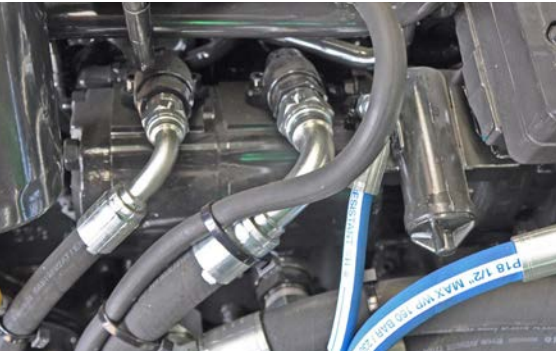
Above: Hydraulic pumps on left hand side of engine.
