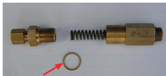
Figure 32. Meter components showing shim
