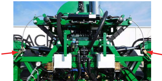
Above: Centre level cable adjusters.
