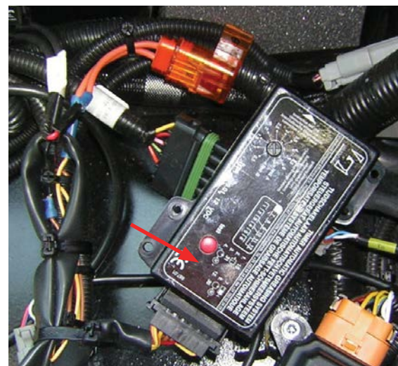
Figure 10. Electronic timer in main fuse compartment
