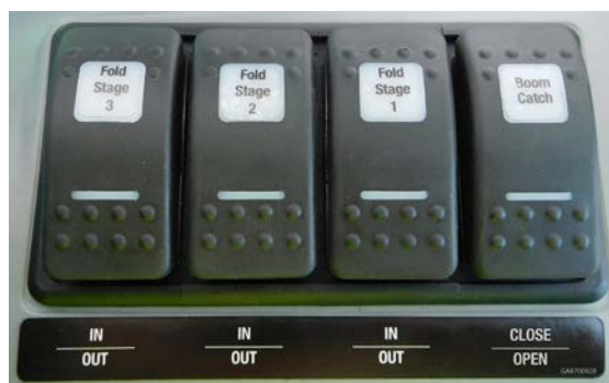
Above: Boom fold controls located on side console.
