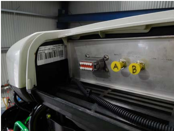
Above: GPS receiver connection points inside the cabin roof on the left hand side.
