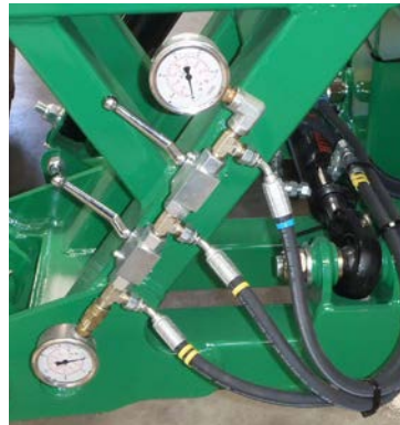
Left: Yaw charge ball valves in the OPEN position.
