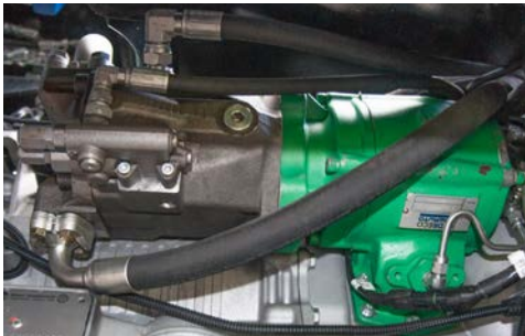
Above: Hydraulic pump on left hand side of gearbox.
