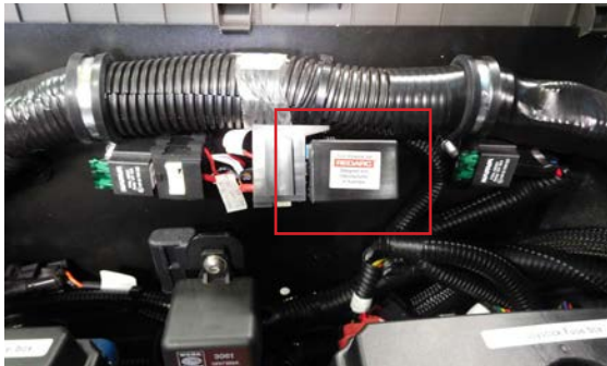
Above: Egress lighting timer relay location in main fuse box area.
