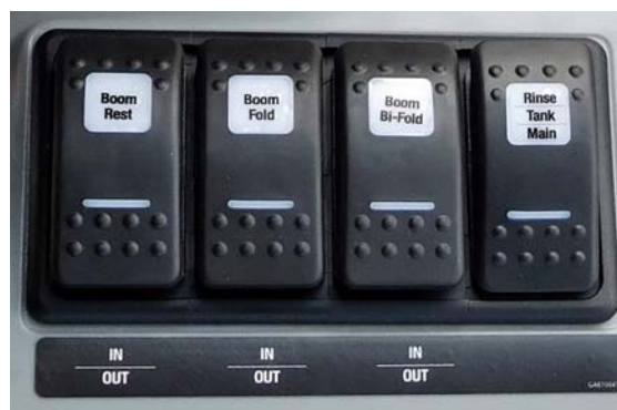
Above: Boom fold controls located on side console.
