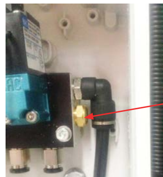
Exhaust port; one located on each end of the manifold.
