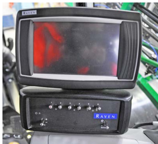
Above: ISOBUS fitted with optional Raven virtual terminal (VT) screen and further optional 6 section switch box.
