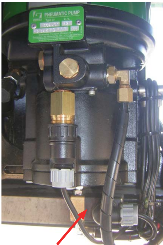
Solenoid located at bottom of pump unit
