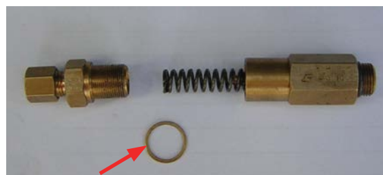
Meter components showing shim
