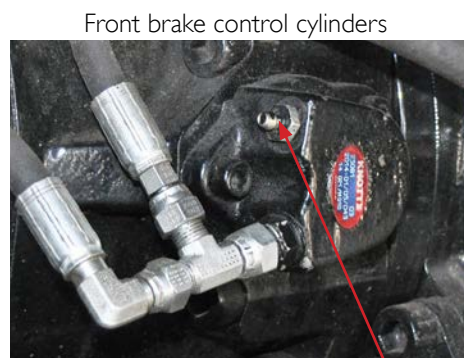
Bleed screw for Service brakes
