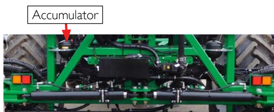
Above: Third stage fold damper accumulator.
