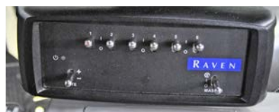
Above: An optional Raven 6 section control box can be programmed to control the 16 sections in any combination of groups or individually.
