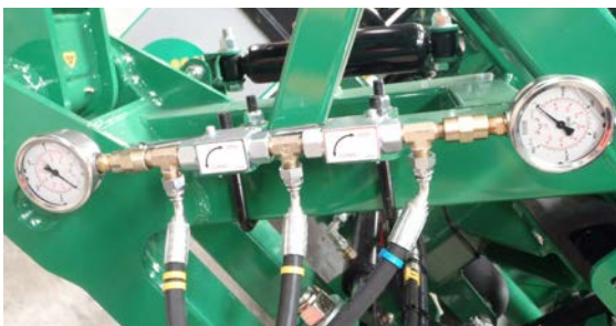
Above: Hydraulic yaw circuit pressure gauges & valves.
