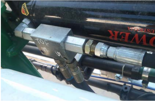
Above: Double pilot operated check valves are mounted to the bi-fold cylinders.
