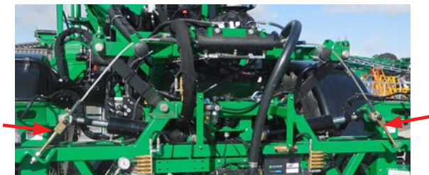
Above: Centre level cable adjusters (36-42m Boom)
