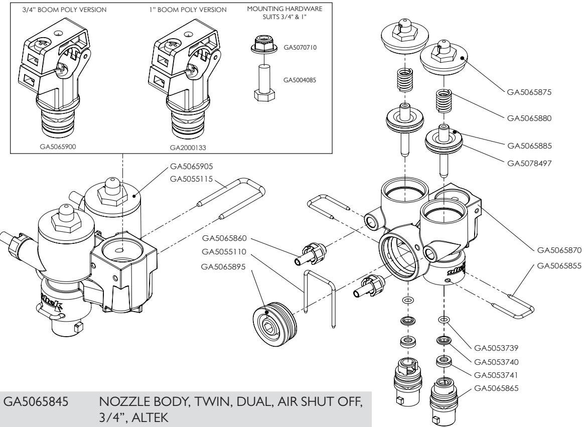
**GA5065845** NOZZLE BODY, TWIN, DUAL, AIR SHUT OFF,
