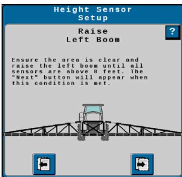
FIGURE 15. Height Sensor Setup - Raise Left Boom
