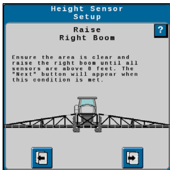
FIGURE 24. Height Sensor Setup - Raise Right Boom
