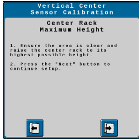
FIGURE 6. Vertical Center Sensor Calibration - Maximum Height
