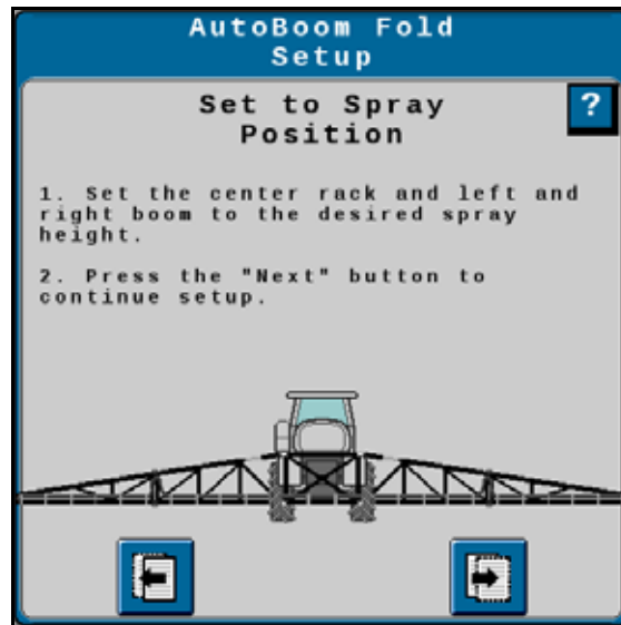
FIGURE 29. Vertical Center Sensor Calibration - Set to Spray Position
