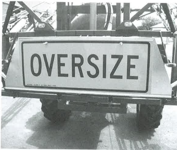
Oversize sign fitted without tail lights.
