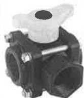
3-WAY POLY BALL VALVE - Directional flow either right or left. - Valve cannot be turned off. V-075-SL 3/4" 3-way poly valve V-100-SL 1" 3-way poly valve
