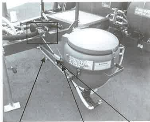
Hopper adjustment arm HOPADJARM Nylon insert RIR-5980 Hopper frame height adjustable CHEMIND-FHA
