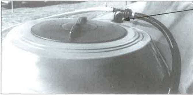
Venturi mounted in top of tank. (Need to drill 1 1/4" hole in top of tank).
