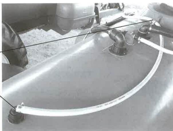
Tank rinsing nozzle assembly TRNA
