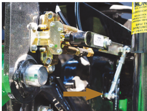
Loosen the bolt on the adjuster plate & move the rod up or down to adjust the ride height, then retighten the bolt.
