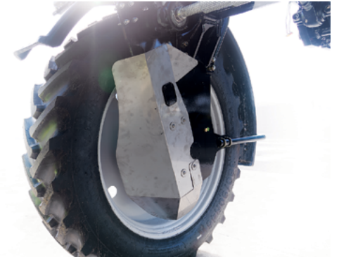
Check dropleg oil level.
