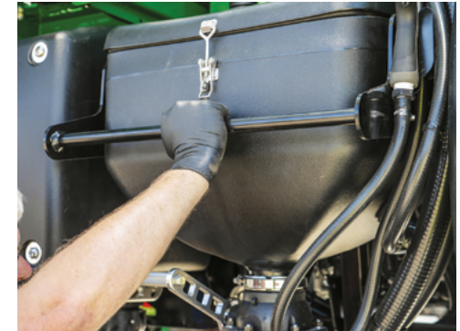
Pull the hopper down into its working position.
