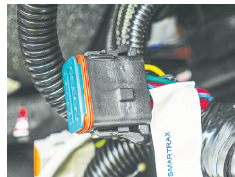
SMARTRAX connector - ISO BUS connection point.
