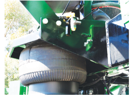
Airbag component of the 5 point suspension system.
