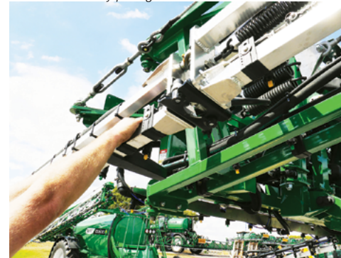
Check tension on the right hand folded outer boom section by pulling the end outwards.
