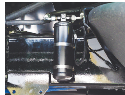
The air conditioner Receiver Dryer.
