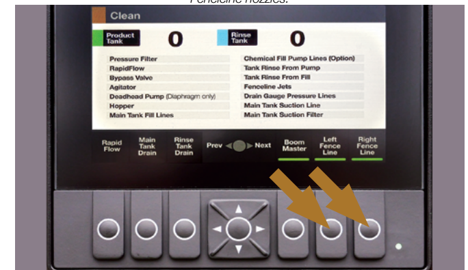
Press the 'Left & Right' Fence Line push buttons 'ON' to begin rinsing the Fence line nozzles.
