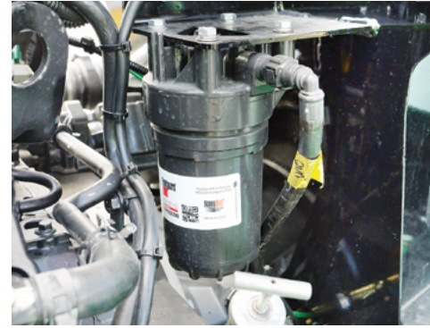
The secondary fuel filter located on the left hand side of the engine.
