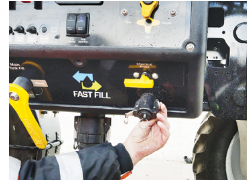
Rotate the Chemical Probe valve to Off. Disconnect the hose from the Probe Inlet & replace the camlock cap.
