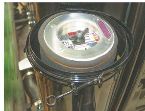
Unscrew the carbon filter retaining nut & remove the filter element from the filter housing.
