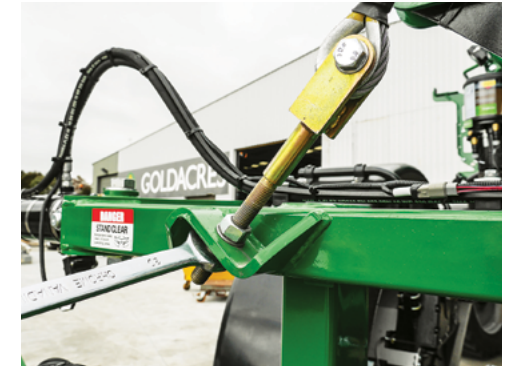
Make adjustment to the Boom Centre Level cable adjusters as required.
