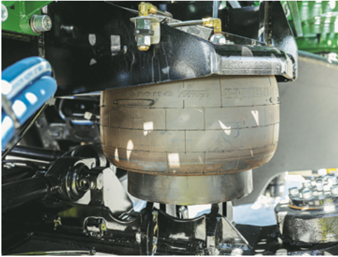
Deflate the air-bag suspension system for more load stability when loading & transporting the sprayer.
