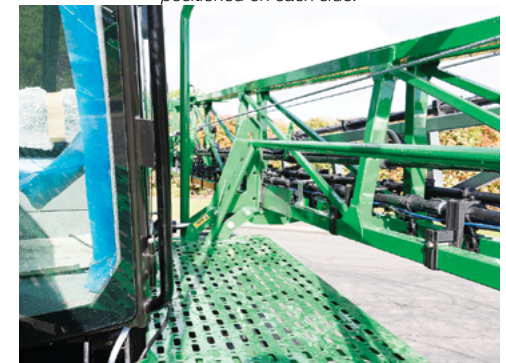
Inner boom rest protection plates must be correctly positioned on each side.
