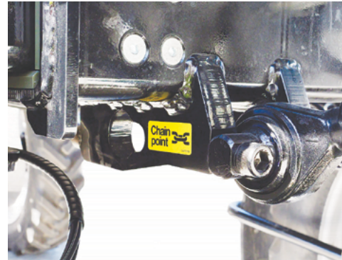
Front right tie-down attachment & towing point.
