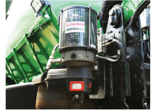
An Alemlube Auto-Greasing System centre (option).
