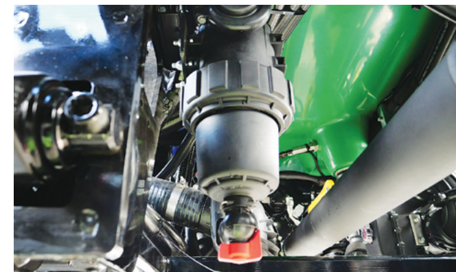
First remove the red valve at the base of the Pressure Filter, then unscrew the filter collar & remove the filter element for cleaning. After cleaning refit all components.
