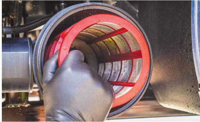
Remove the Suction Filter screen.
