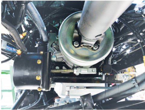
The Park Brake (a drum brake) is located at the rear of the gearbox.
