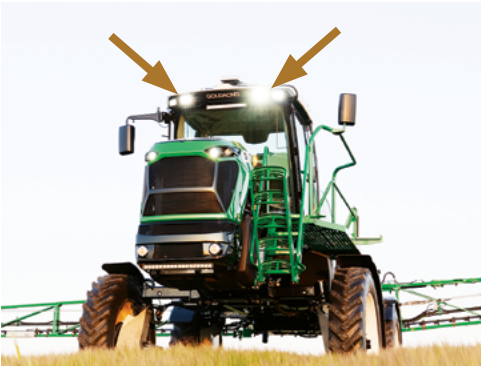
Two Egress lights on the front corners of the cabin provide exit safety in dark conditions.
