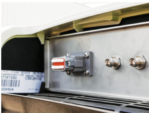
The cover removed showing the antenna connectors.
