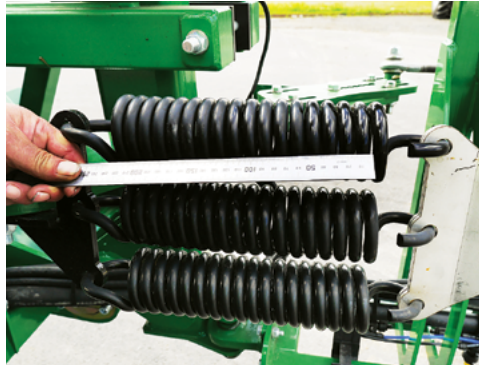
Check there is a 3 mm gap in the spring coils and adjust if required.
