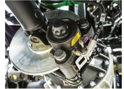
The Park Brake (a disc brake) is mounted on the rear differential.
