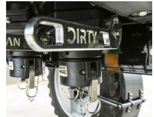
The 3" Dirty Fill inlet with camlock cap fitted.
