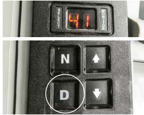
Press the D push button to engage reverse gear for reversing the sprayer.
