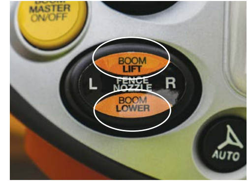
The Boom Lift & Boom Lower push button used to raise & lower the boom height as required.
