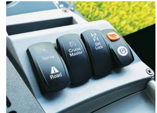
The Mode Switch panel (The Differential Lock Switch is optional for 4WD models only).
