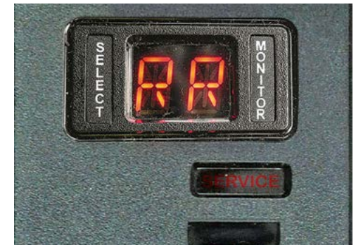
Select & Monitor displays showing Reverse gear.
