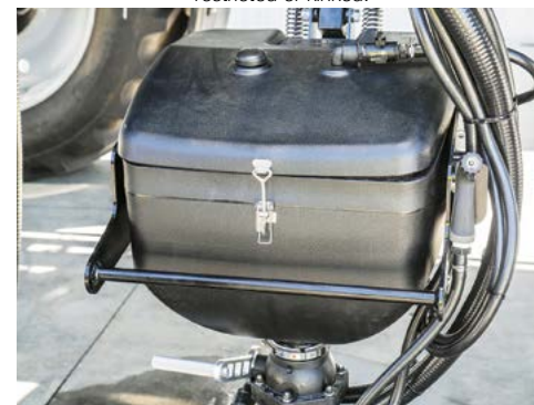
With hopper in working position, check hoses are not restricted or kinked.
