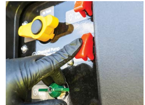
Switch On the Wash Down Gun pump.
