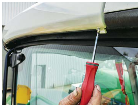
Remove the screws from the antenna connectors cover.
