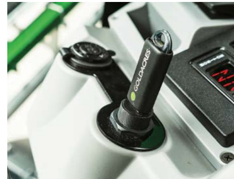
The Back-Up/Restore USB is provided to back-up & restore system settings & data.
