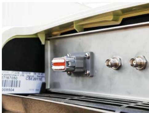
The cover removed showing the antenna connectors.
