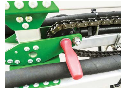
With the boom tip pulled back, place a pin through the holes to hold the sprocket to adjust the turnbuckle.
