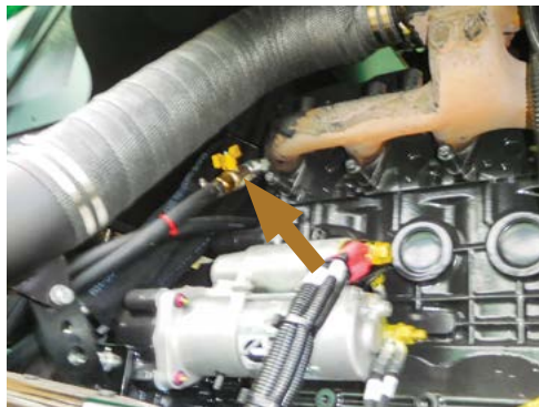
The 1st heating core Isolating Tap located on the right hand side of the engine at the rear of the exhaust manifold.
