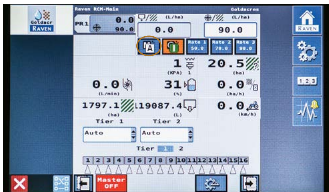
The Raven Control Module (RCM) home screen showing 'Automatic' mode.
