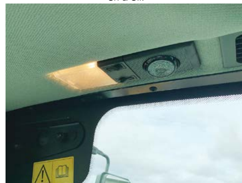
Use the Outer rocker switch to switch the front map light On & Off.
