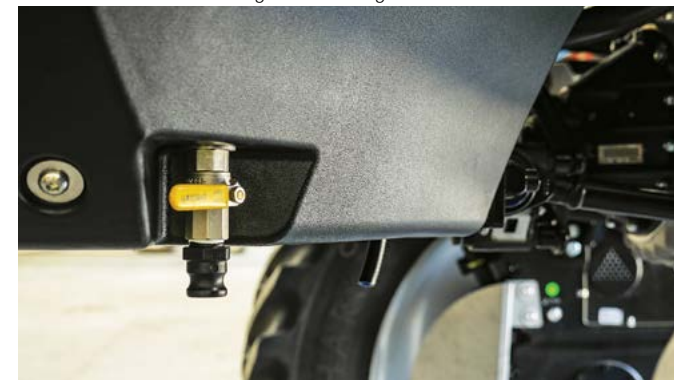
Fresh water tap for personal washing & safety, located at the base of the Quick Filling Station Storage Cabinet.
