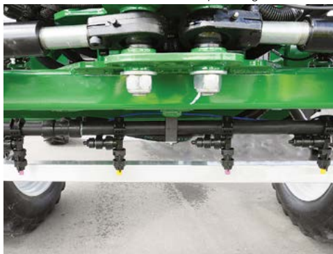
Two nozzles plumbed either side of the centre of the boom - referred to as broadacre plumbing.
