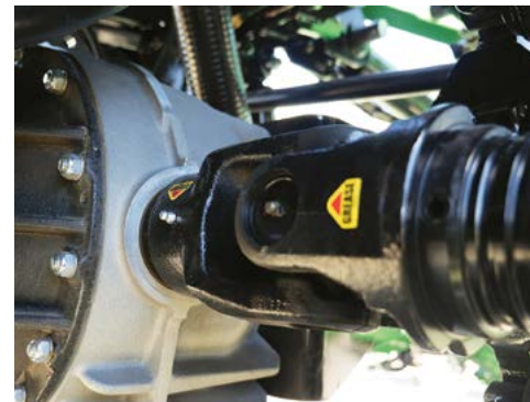
Driveshaft 'Manual Grease Points'.
