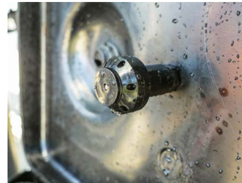
The Hopper Rinse Nozzle located under the hopper lid.
