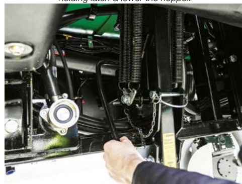
Support the hopper weight & lift the lever to unlock the holding latch & lower the hopper.
