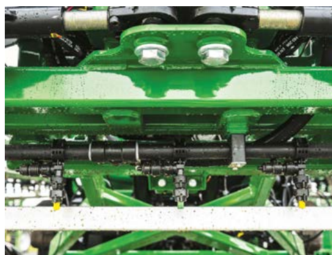
Centreline plumbed boom with optional 3TS single nozzles at 250mm spacing.
