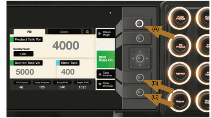
Press the Screen Selector push button (A) to select the Fill screen, then press the 'Tank Increase' (B) or 'Tank Decrease' (C) push buttons to set the required fill volume.
