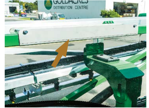
Ensure boom Protection Brackets are positioned correctly.
