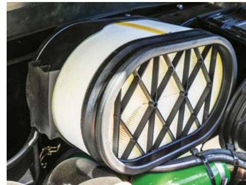
Fit a new primary air filter.
