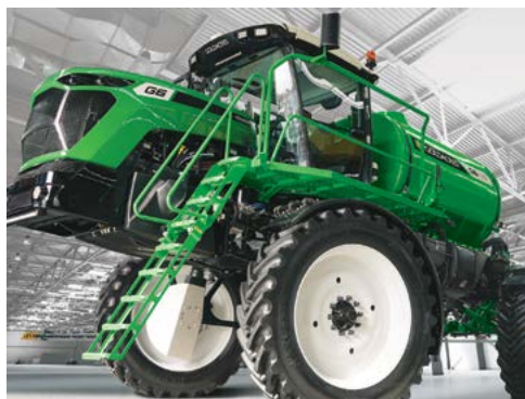
The folding stairway & walkway platform provide cabin access.
