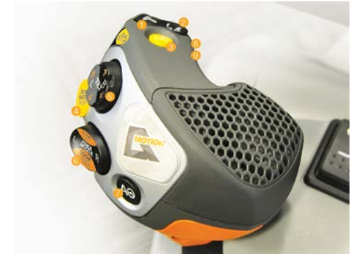
Check all joystick boom switch functions.
