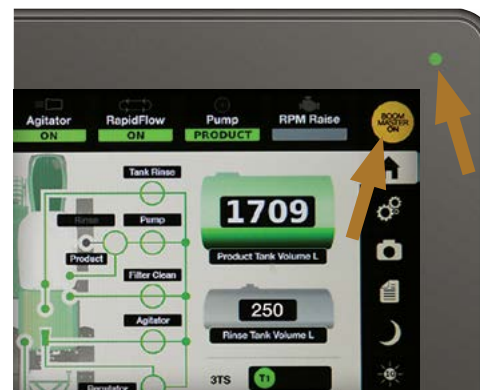
Green light indicator functional change & the Boom Master switch is now a touch button
