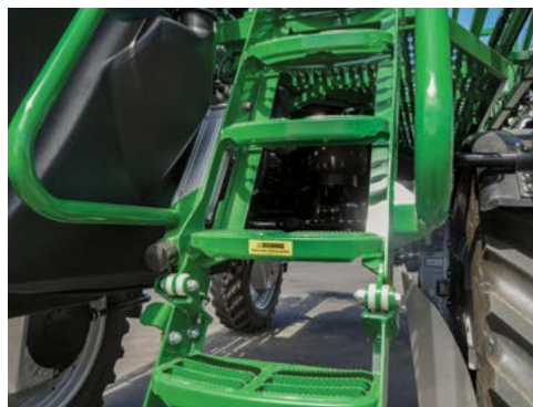
Use the stairway & walkway platform to enter the cabin. Understand its Warning decal before operating.
