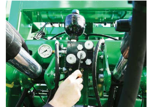
Loosen the locknut and adjust the Breakaway Bleed Valve (8).
