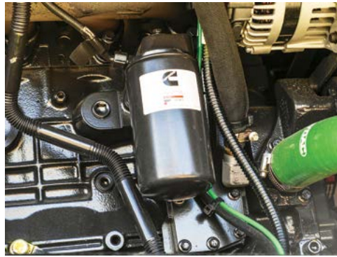
Engine oil filter located on the right hand side of the engine.
