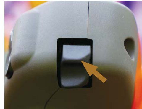
Dual Tilt rocker switch on the Joystick used to tilt boom wings up for folding.
