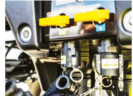
Disconnect the Chemical Probe hose & refit the camlock cap.
