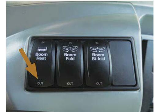
Press & hold down the Boom Rest OUT rocker switch to unlock the LHS boom rest
