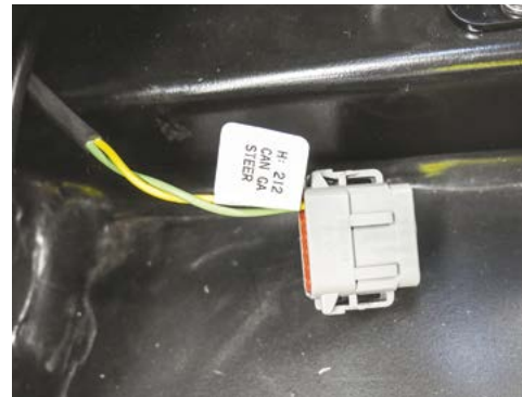
Steering CAN connector in the electrical compartment.
