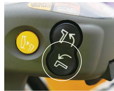
Press the lower Cruise Set/Decrease push button to set the current ground speed for Cruise Control. Once set, press the push button again to decrease set ground speed.
