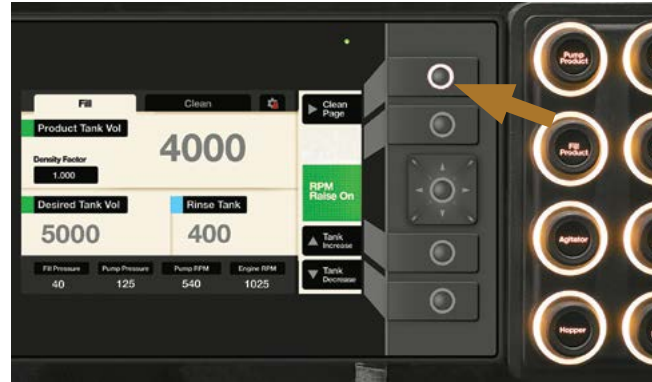
Press the Screen Selector push button to select the Fill screen.
