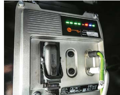
The ISOBus Module (also known as the Chassis Controller or Main Control Module) located in the storage box of Quick Filling Station.
