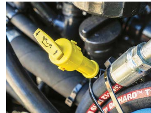
Engine oil dip stick (shown left [yellow]) & engine oil filler cap (shown behind the dipstick).
