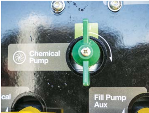
Turn the Chemical Pump valve ON.
