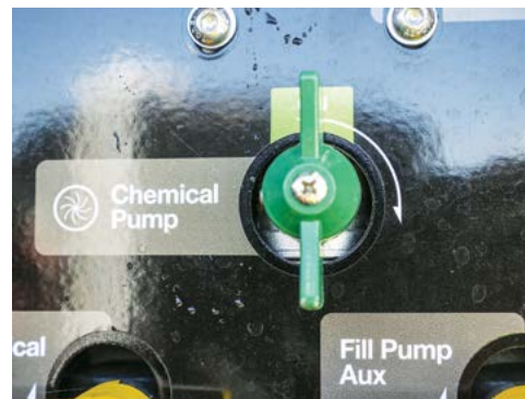
Turn the Chemical Pump valve ON.
