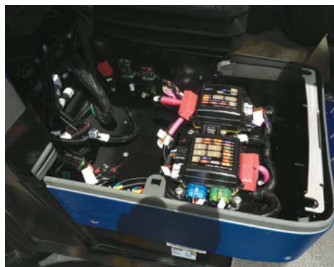
Electrical compartment located below the Armrest Control Console.
