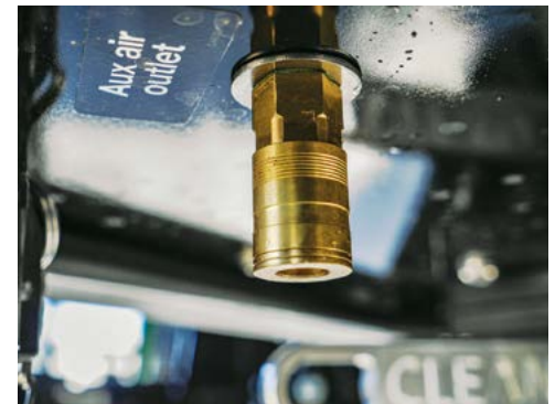
Auxiliary Air Outlet located in the left hand side fill area .
