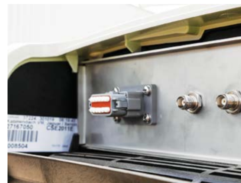
The cover removed showing the antenna connectors.
