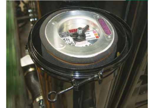
Unscrew the carbon filter retaining nut & remove the filter element from the filter housing.
