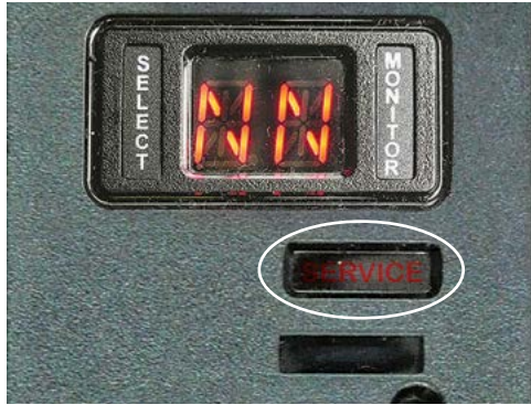
If the SERVICE indicator is illuminated, then a fault in the shift by wire system has occurred.
