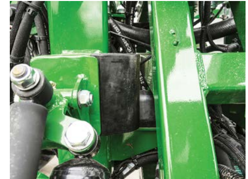
Check rubber bumpers for wear. Replace if worn.
