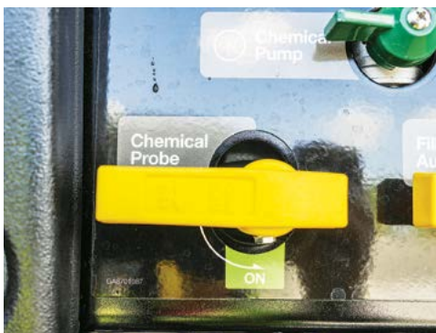
Rotate the Chemical Probe valve to Off position.
