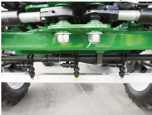
A single nozzle plumbing to the centre of the boom- referred to as centreline or row crop plumbing.
