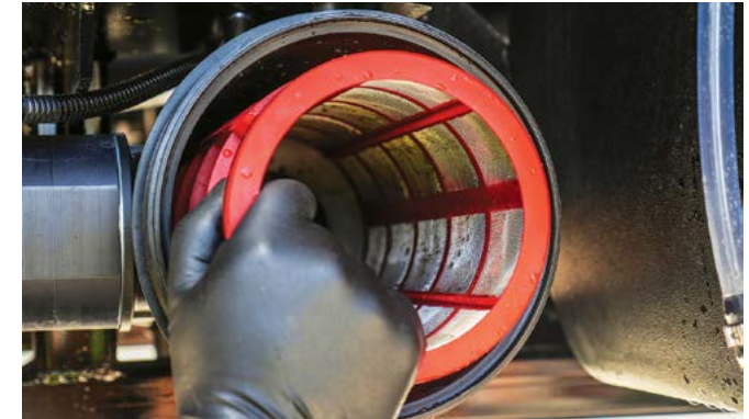
Remove the Suction Filter screen.
