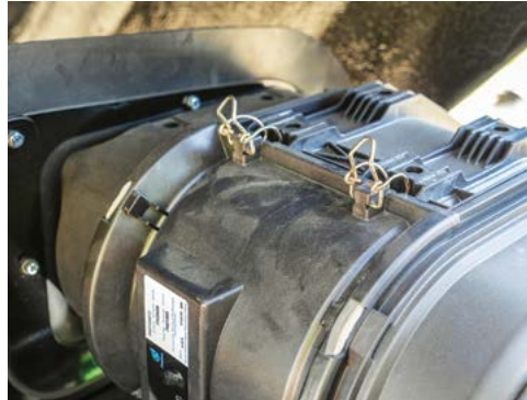
Release the cover clips on top of the air cleaner.
