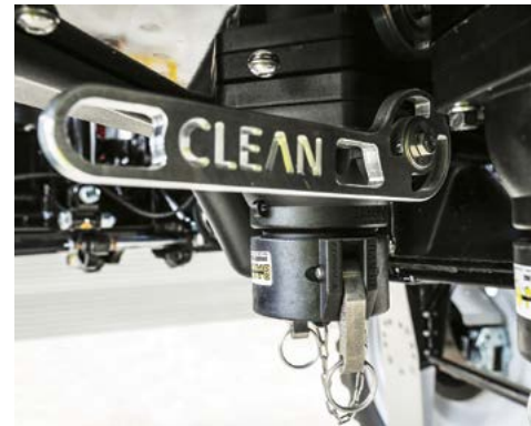
The 3" Clean Fill inlet with camlock cap fitted.
