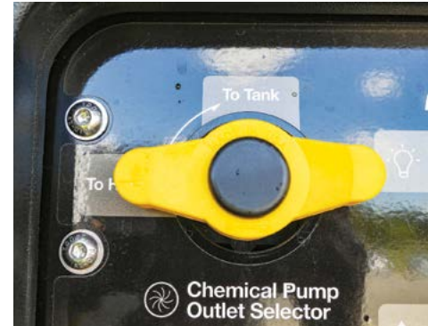
Rotate the Chemical Pump Output to Hopper position.
