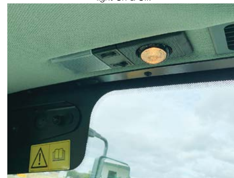
Use the Inner rocker switch to switch the directional map light On & Off.
