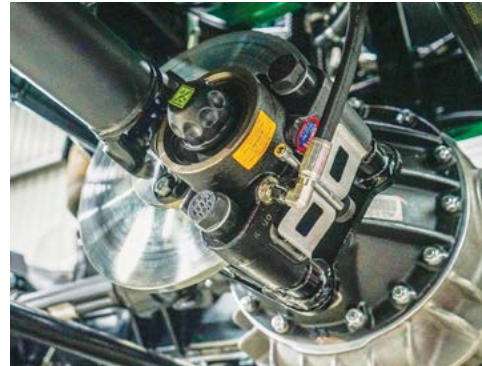
The Park Brake on the rear driveshaft.
