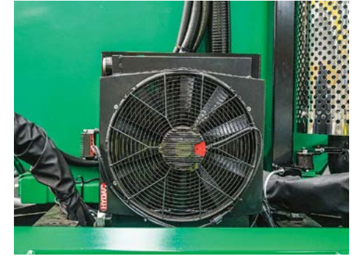
The Hydraulic Oil Cooler behind the spray tank
