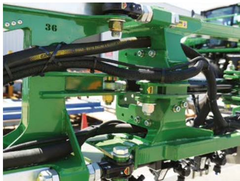
Boom wing fold 'Manual Grease Points'.
