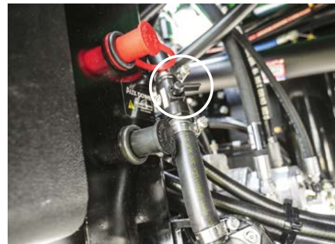
Close the Rinse Coupling Valve, then disconnect the hose from the Micromatic coupling on the Cruiser.
