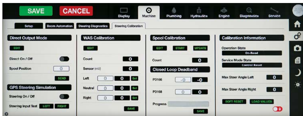
The 'Steering Calibration' screen showing menus & touch button functions.
