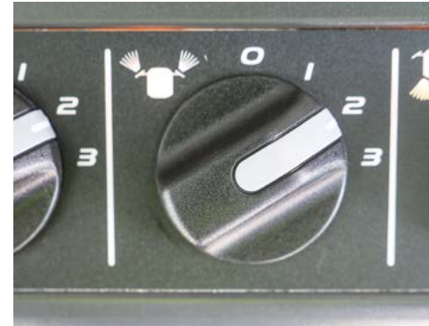
The Outer Front Work Lights Switch.
