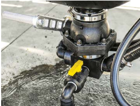
Open the Bottom Ball Valve to transfer chemical to the main tank.
