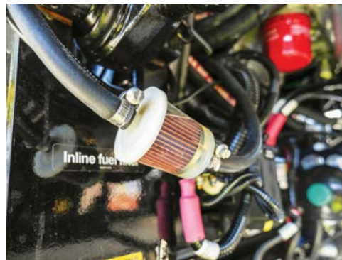
The Inline fuel filter located on the left hand side of the engine.
