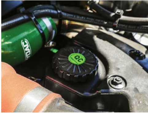
Engine oil filler cap in the rocker cover on top of the engine.
