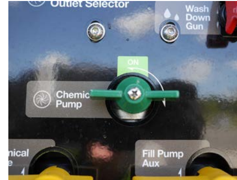
Rotate the Chemical Pump valve to Off position.
