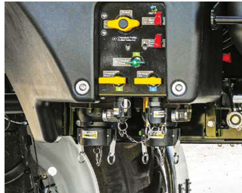
The 3" Clean Fill (left) & Dirty Fill (right) inlets with camlock caps fitted.
