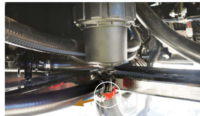
The red valve at the base of the pressure filter must be open for back-flush cleaning to function.
