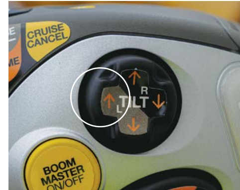
Press & hold the L Arrow Up part of the Boom Tilt push button to tilt up the left hand boom end.
