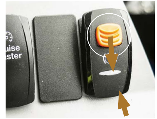
Disengage the Park Brake - slide back the orange lock, then press the switch rearward (Off position).
