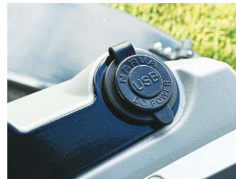
The dual USB outlet enables charging of phones or other USB devices.
