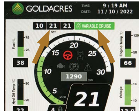
'Variable Cruise Control' with Set Speed shown centre left & Low Speed (left of centre) & High Speed (right of centre).
