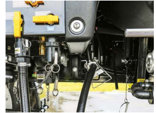
Connect a hose for Micromatic filling to the Chemical Probe inlet.
