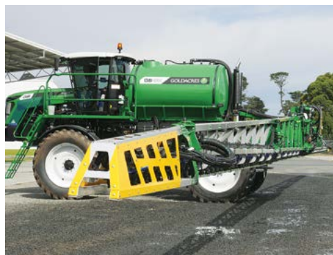
On level ground, engage the Park Brake, chock wheels & have the boom in its working position before making adjustments.
