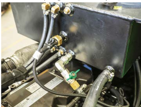
Open the heater ball valve (on the top rear of the engine) when replacing coolant to bleed any air.
