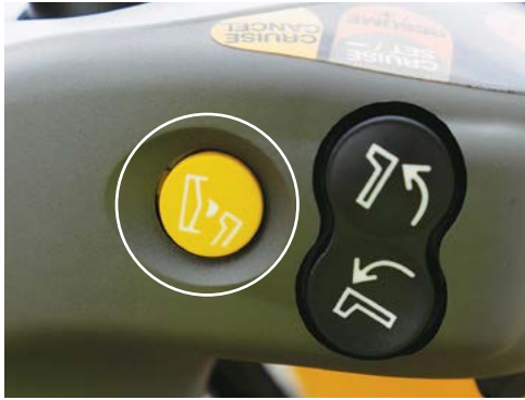
The Cruise Cancel push button on the side of the Joystick used to cancel the cruise control function.
