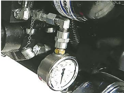
Attach a pressure gauge (with an elbow fitting) to test port 3 (TP3) on the manifold.
