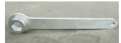
The Park Brake manual release tool (GA4602900) supplied with the Cruiser.
