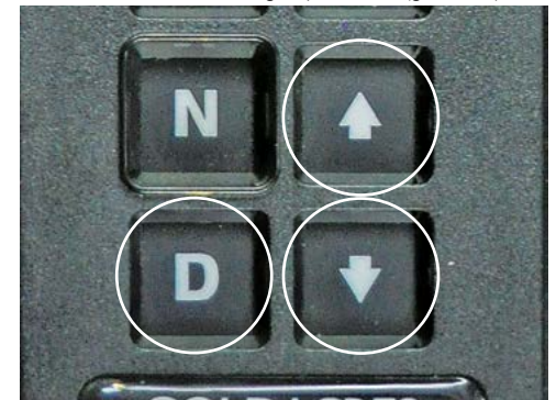
Press the 'D' switch to engage 1st gear. 1-6. Press the Arrow switches to change Up or Down (gears 1-6).
