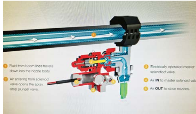
Illustration of the RapidFlow and RapidFire nozzle technologies.
