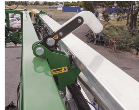
The left hand side Boom Rest lock unfolded - 32 & 36m booms only.
