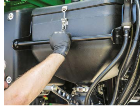
Lift & push the hopper up into its transport position.
