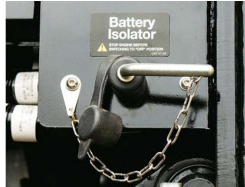
The Battery Isolator located on the right hand side of the engine.
