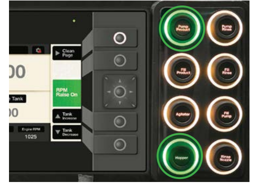
Press the 'Pump Product' push button On & the 'Hopper' push button On.
