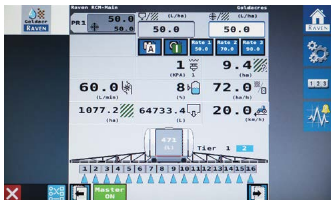
Home screen of the Spray Rate Controller & Raven Control Module (RCM).
