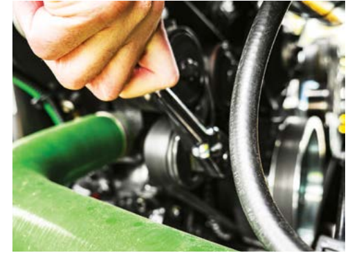
Use a breaker bar with a 1/2" socket to release the engine belt tensioner.
