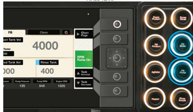
Press the 'Fill Rinse' push button, then 'Fill Product' push button to start filling the Rinse Tank.
