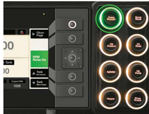
Press the 'Pump Product' push button On to engage suction of the Product Pump from the Product Tank.
