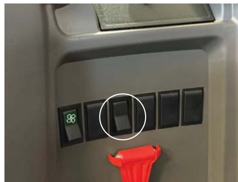
Press & Hold the Adjustable Axle Track In/Out Rocker Switch (on the cabin corner panel) as required while travelling forward at 10kph.
