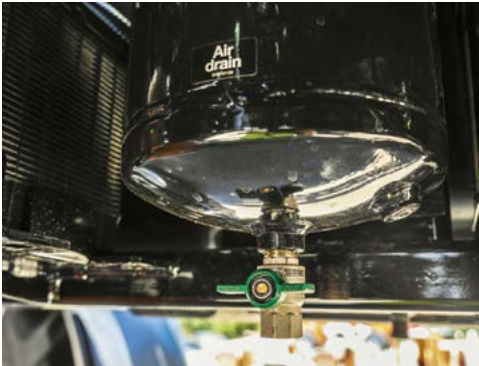
Manual drain tap at the base of the Air Tank.
