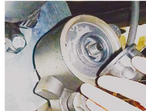
Remove the dust cap from the Park Brake caliper (unscrew counter-clockwise).
