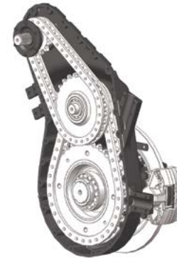
Replace dropleg drive chains when necessary.
