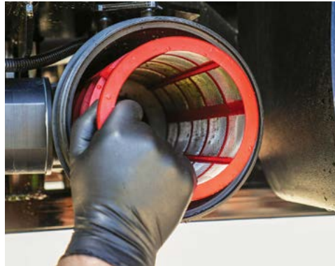
Check the suction filter is clean.
