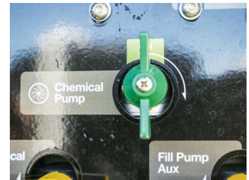
Turn the Chemical Pump valve ON.
