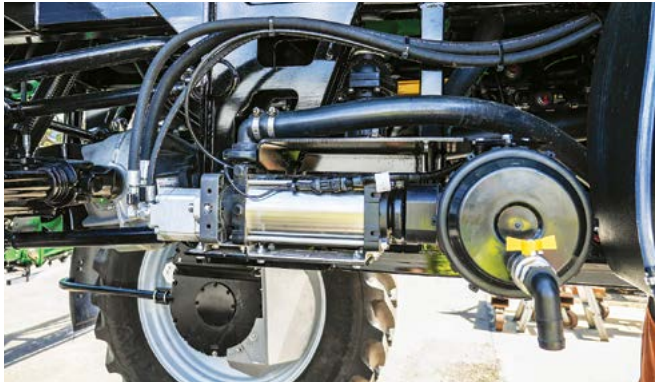
The Suction Filter shown with a centrifugal pump.
