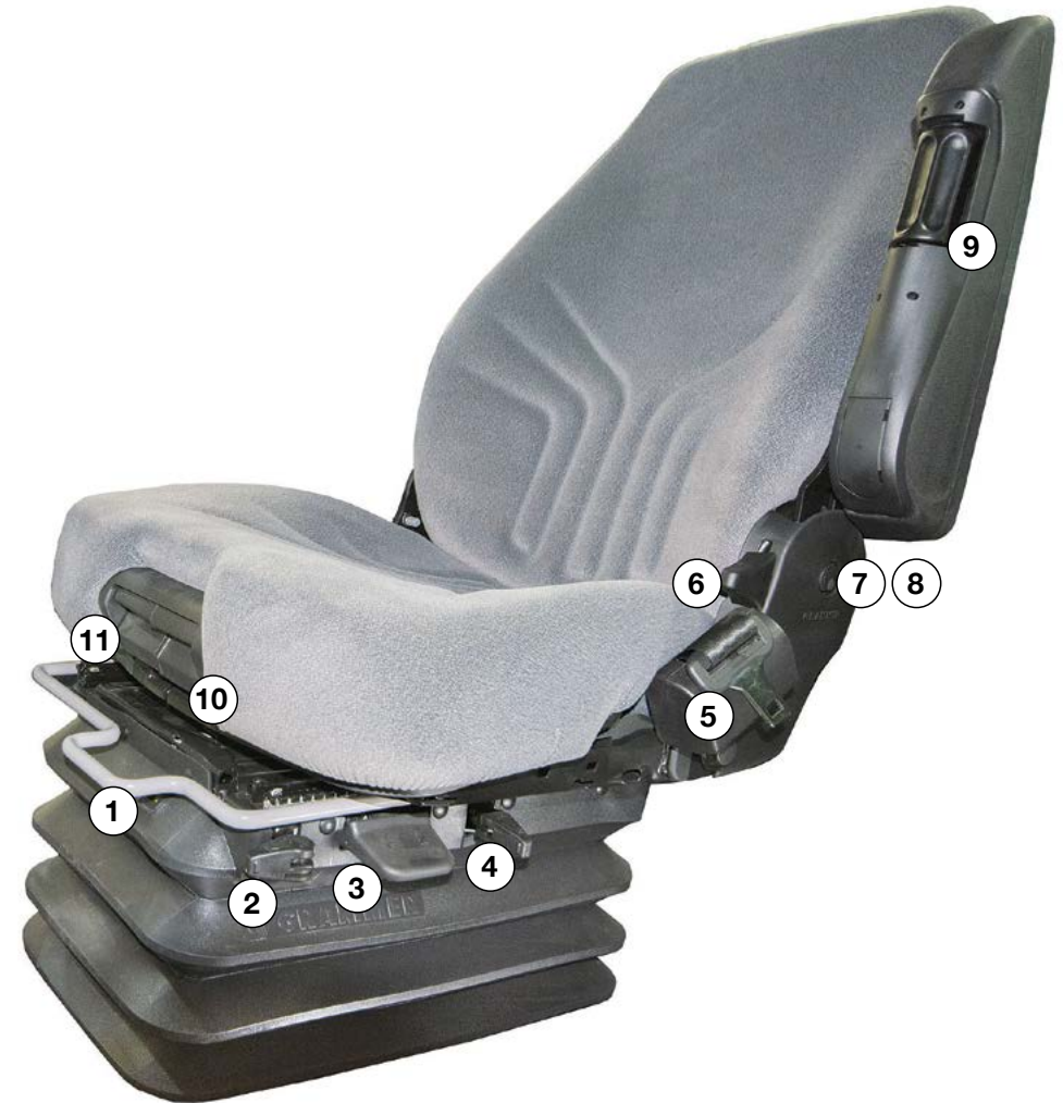
Location of the Operator Seat settings (refer to numbered information & headings on this page for instruction). All position, weight, height & comfort adjustments must be made before driving.
