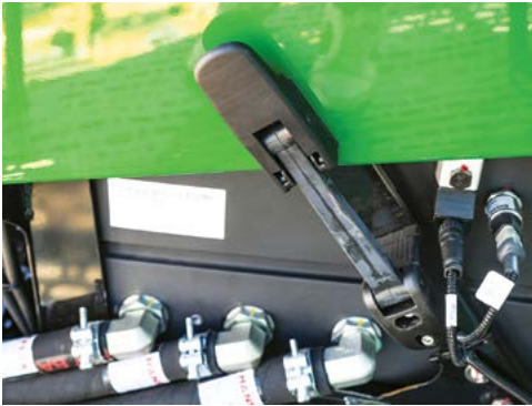
To open the bonnet unclip two latches, located on either side of the bonnet near the cabin.
