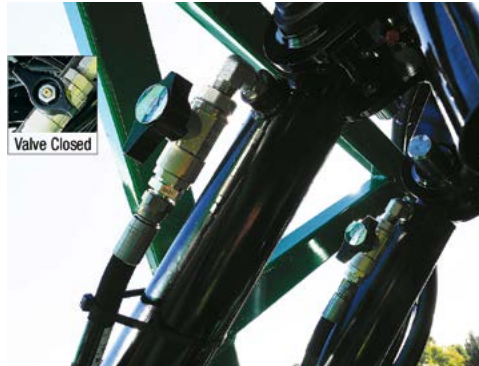
Close the ball valve on each lift cylinder for safety.
