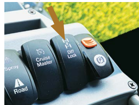
On 4WD models only, press the top of the Diff Lock switch to cycle the differential lock On or Off.
