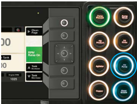
Press the 'Fill Pump' push button On.
