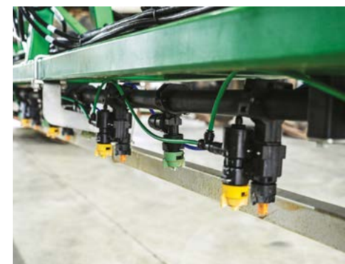
Boom with 3TS Pro with alternating single & double nozzles at 250mm spacing.
