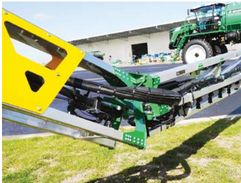
Upwards Tip Breakaway function.
