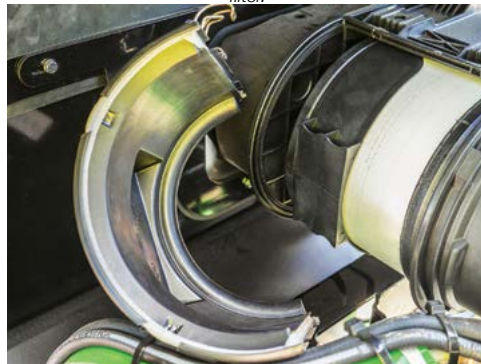
Remove the air cleaner cover, then remove the primary air filter.
