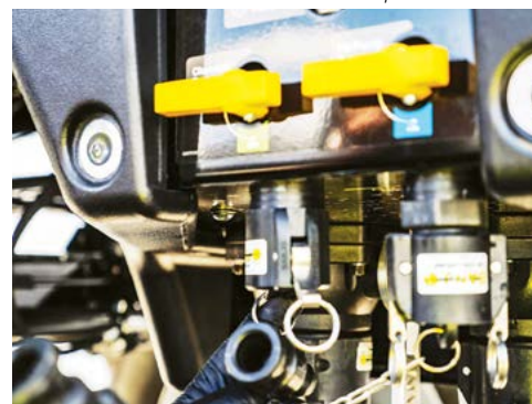
Disconnect the Micromatic hose from the Chemical Probe Inlet & refit the camlock cap.
