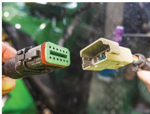
Fit the Starfire adaptor cable & Starfire Receiver cable connectors.
