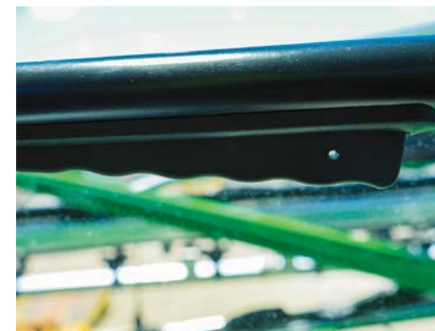
Squeeze the door handle lever to open the cabin door latch, then push the door handle to open the door.
