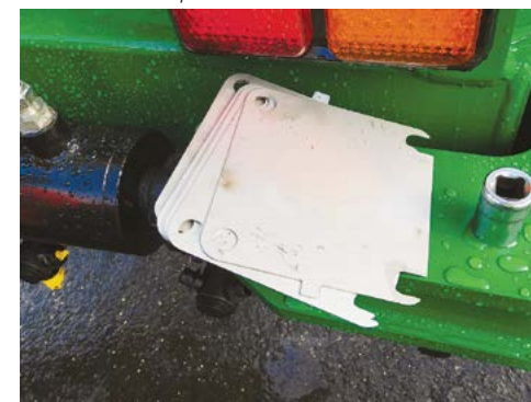
Face the open slot of the shims downwards.
