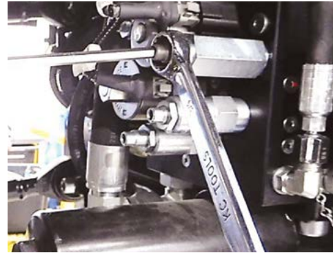
Wind In the adjuster screw on pressure relief valve (RV08) until the gauge reads 200 Bar, then tighten the lock nut.
