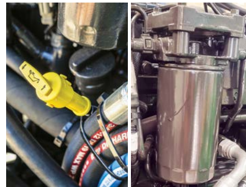
The Secondary fuel filter located on the left hand side above the engine oil dip stick.
