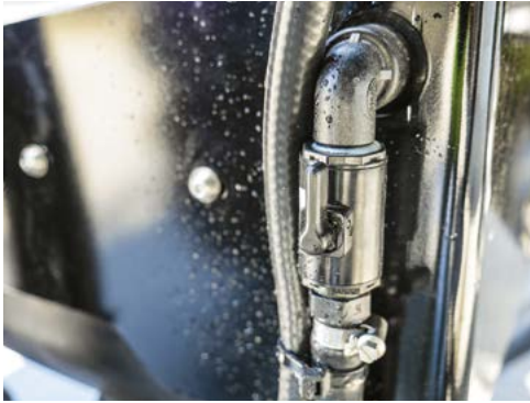
Open the Mixing Jet valve on the RHS of the Hopper.
