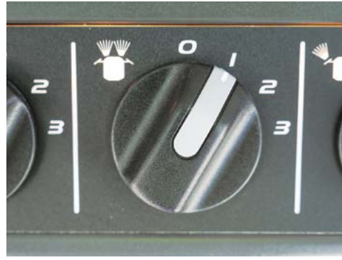
The Inner Front Work Lights Switch.
