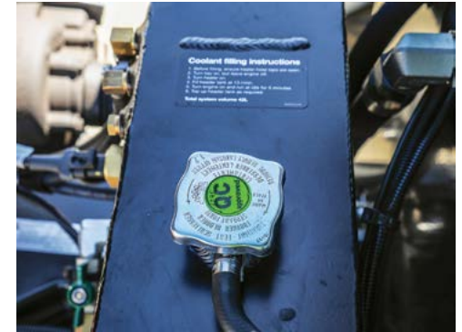
The engine radiator & radiator cap.
