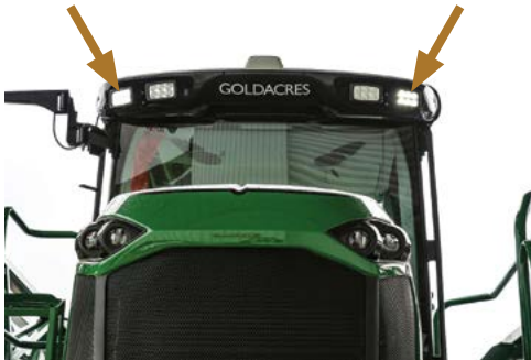
Two Egress lights on the front corners of the cabin provide exit safety in dark conditions.
