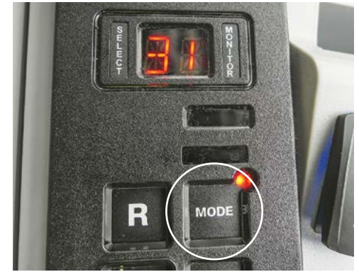
Press the 'Mode' push button to engage the Pre-Select
