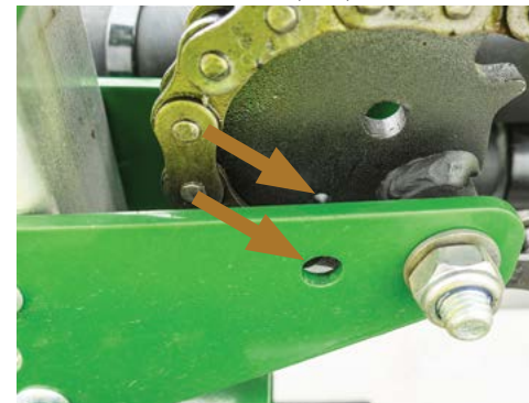
The small hole in the sprocket must align with the hole in the side of the pivot plate.
