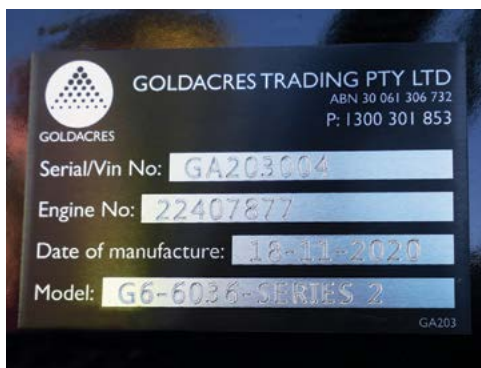
The serial number plate located on the chassis at the front left hand side by the cabin access ladder.
