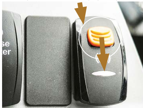
Engage the Park Brake - slide back the orange lock & press the switch forward (On position).
