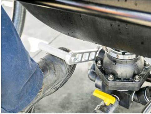
Lift-up to Close the foot operated ball valve at the bottom of the hopper.
