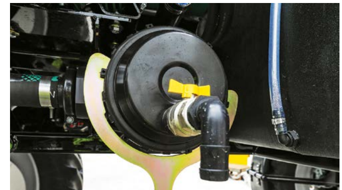
Fully tighten the filter bowl collar & close the drain valve.
