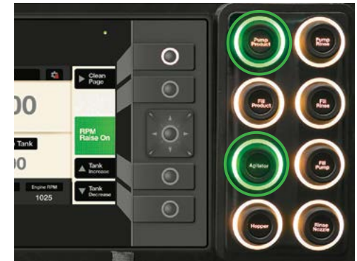
Press the 'Pump Product' push button On, then press the 'Agitator' push button On to keep chemicals mixed.
