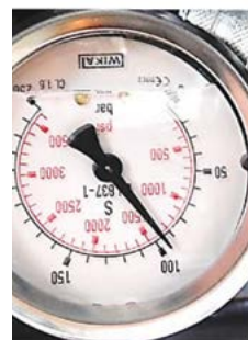
After the adjusting the screw until the gauge reads 200 Bar, pump the brake and the pressure will drop.
