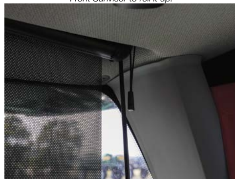
Pull downwards on the cord on the right hand side of the Front Sunvisor to roll it up.
