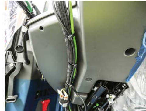
Lift up the Armrest console and release the G-Hub cable harness from underneath.
