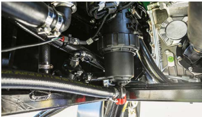
The Pressure Filter showing the red valve (tap) in Open position at the base of the filter.
