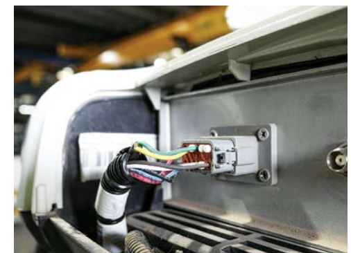
The Starfire adaptor cable fitted to the front connector.
