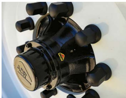
Recommended wheel nut torque tension is 320 ft/lb.
