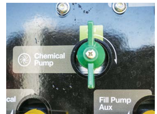
Turn the Chemical Pump valve ON.
