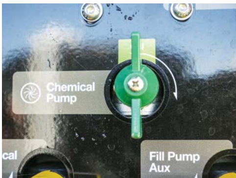
Turn the Chemical Pump valve On.
