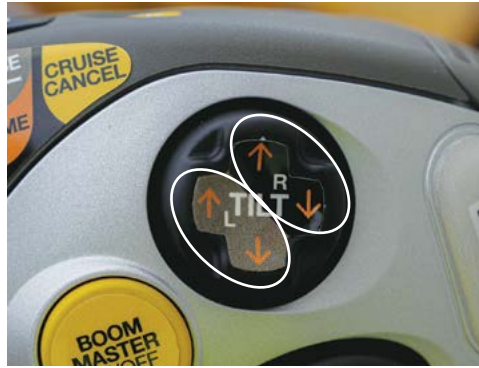
The L & R Arrow Boom Tilt push button used to tilt boom ends up & down.
