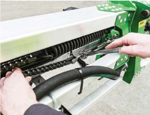
Adjust the turnbuckle to adjust spring tension as required.
