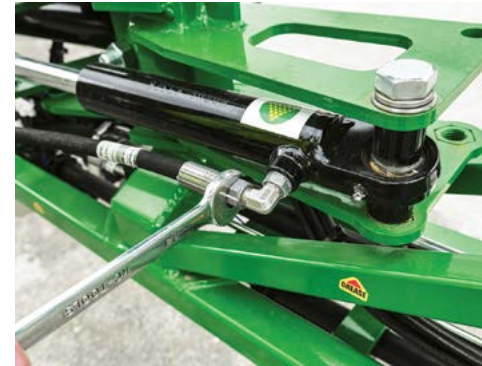
Slightly loosen the hydraulic hose fitting on a breakaway cylinder (approximately one full turn).
