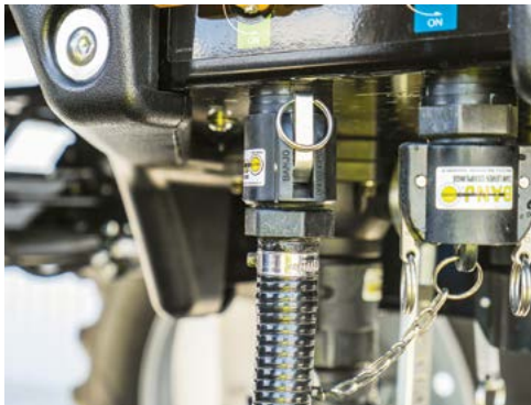
Connect a hose for Micromatic filling to the Chemical Probe Inlet.
