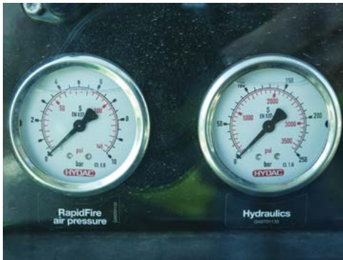
The RapidFire air pressure and Hydraulic Oil pressure gauges in the console in front of the steering column.
