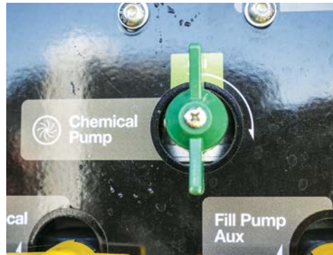
Turn the Chemical Pump valve On.
