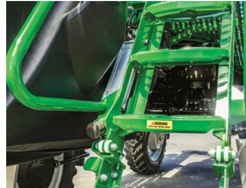
The pneumatic cylinder raises & lowers the Folding Ladder for cabin access.
