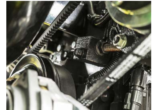
Use the lock nuts on the adjuster to pivot the compressor and tension the belt.
