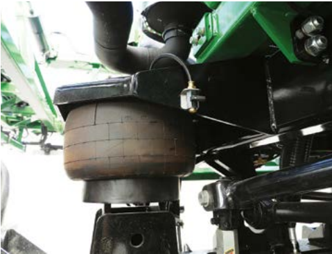
Air bag dump valve closed.
