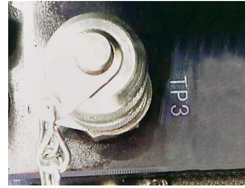
Remove the pressure gauge from test port & replace the dust cap
