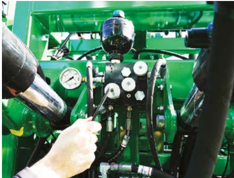
Loosen the locknut and adjust the pressure with the Pressure Reducing Valve (8).
