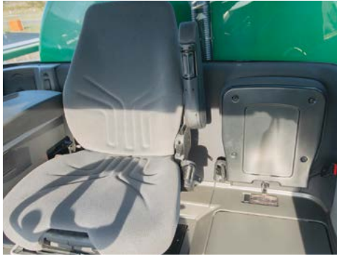
The cabin is equipped with an Operator's seat (left) and a fold-up Training seat (right - folded up).
