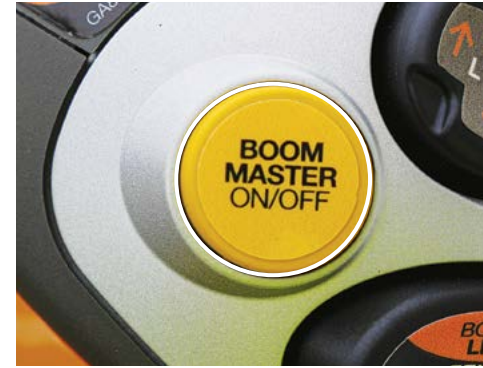
The Boom Master push button used to start & stop the boom spraying.
