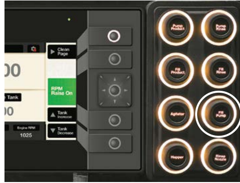
Press the 'Fill Pump' push button Off.
