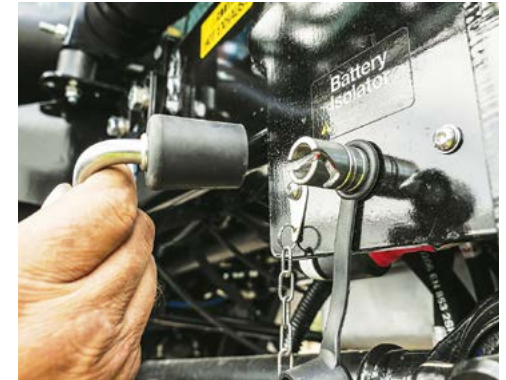
Engage the batter isolator switch to provide power to the Cruiser systems.
