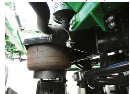
Check airbags are functioning correctly.
