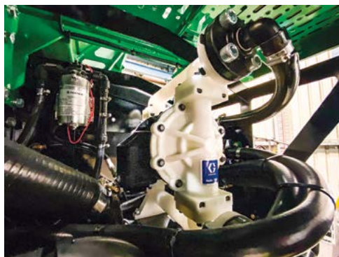
Air driven chemical transfer pump.
