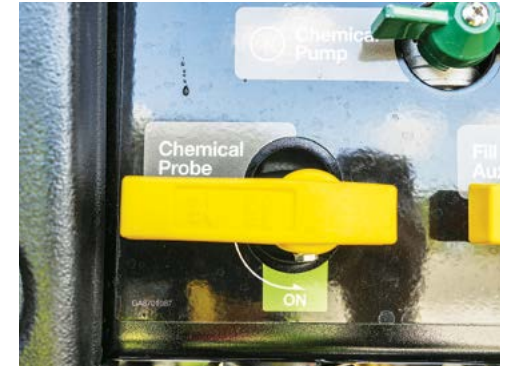
Rotate the Chemical Probe valve to Off position.
