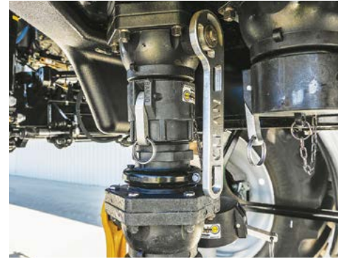
Connect a 3" fill hose to the 'Clean Fill' inlet & Open the 'Clean Fill' ball valves.
