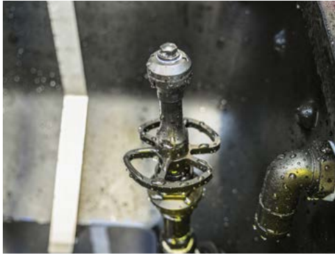
Open the hopper lid to access the Drum Rinse Nozzle.
