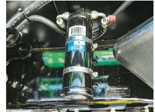
The air conditioner Receiver Dryer.
