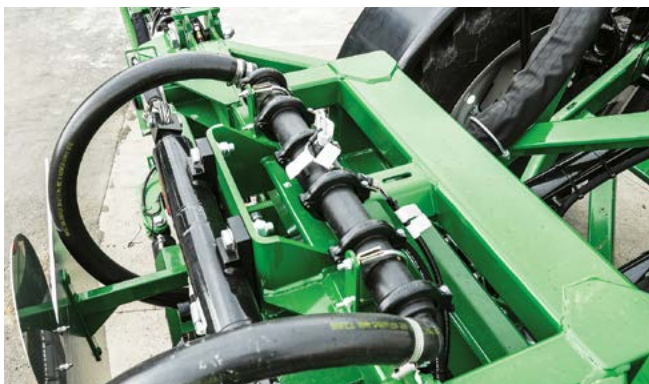
The Flow Meter, located on top of the boom centre section, should regularly be inspected & cleaned.
