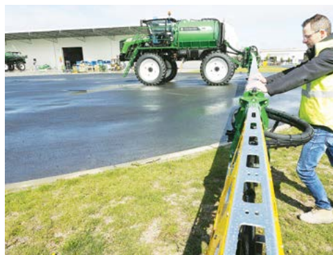
Move the boom fore & aft to purge air from the Yaw hydraulic circuit.
