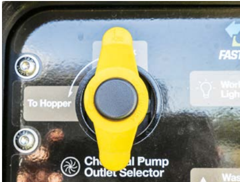
Rotate the Chemical Pump Output to Hopper position.
