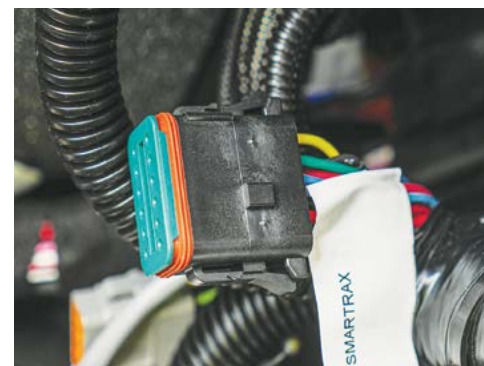
SMARTRAX connector - ISO BUS connection point.
