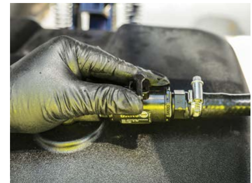
Check the 'Hopper Rinse' valve on the top of the hopper is Closed.
