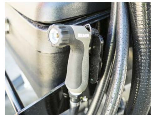
The Wash Down Handgun on the outside of the hopper.
