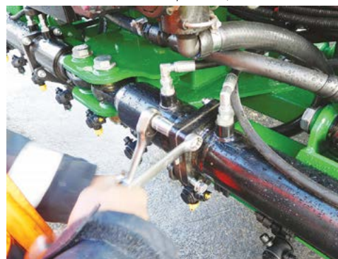
Loosen and remove the top 2 bolts, nuts & washers.
