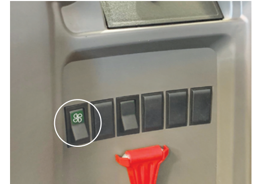
Press the Carbon Filtration Fan Rocker Switch to activate the Carbon Filtration System Fan before spraying.
