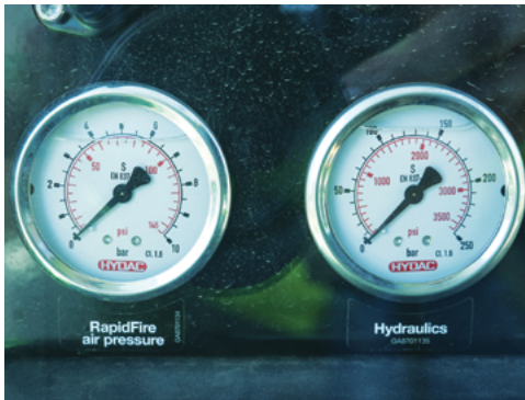
The RapidFire air pressure and Hydraulic Oil pressure gauges in the console in front of the steering column.
