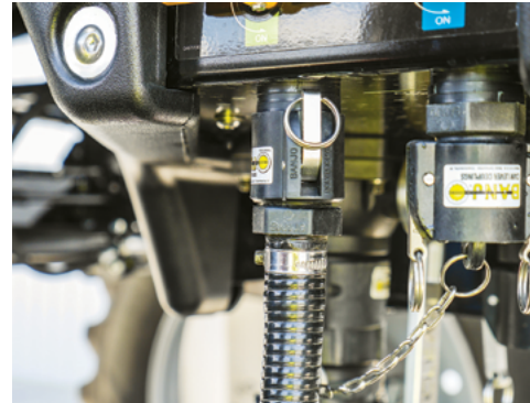
Connect a hose for chemical probe filling to the Chemical Probe Inlet.
