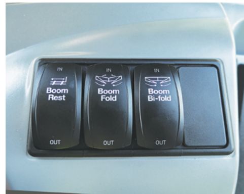
Boom Rest, Boom Fold & Boom Bi-fold rocker switches used for folding & unfolding the boom.
