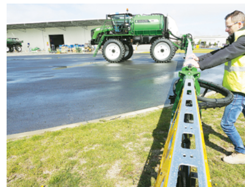
Move the boom by hand to adjust the Yaw Alignment.
