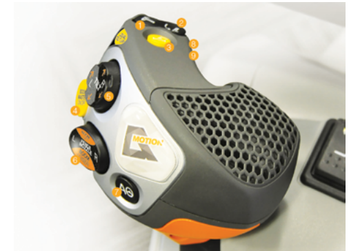
Check all joystick boom switch functions.
