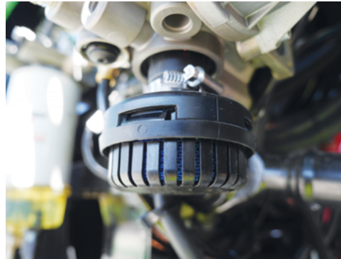
Replace the coalescing air dryer cartridge every one or two years.
