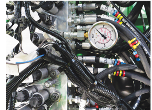
Pressure gauge located on the F3MC Port (48m).
