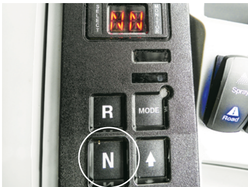
Press the N push button to deactivate all gears.
