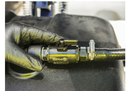
Open the Rinse Valve on top of the hopper lid.
