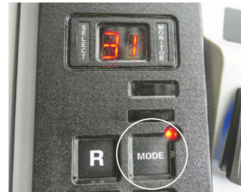
Press the 'Mode' push button to engage the Pre-Select 3rd Gear.
