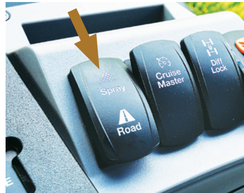
Press the top of the Spray Mode/Road Mode switch to activate Spray Mode
