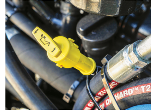
Engine oil dip stick (shown left [yellow]) & engine oil filler cap (shown behind the dipstick).
