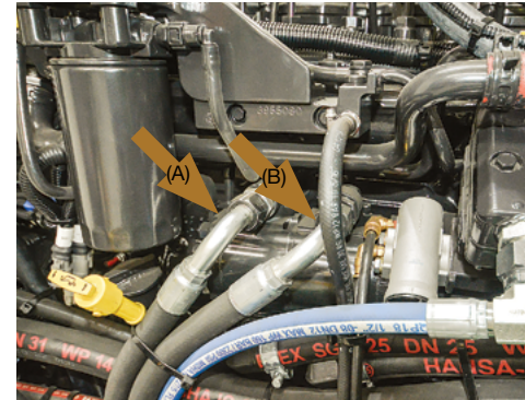
Twin hydraulic gear pumps - 22cc (A) & 32cc (B).
