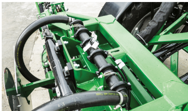
The Flow Meter, located on top of the boom centre section, should regularly be inspected & cleaned.
