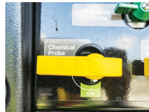
Rotate the Chemical Probe valve to Off position.
