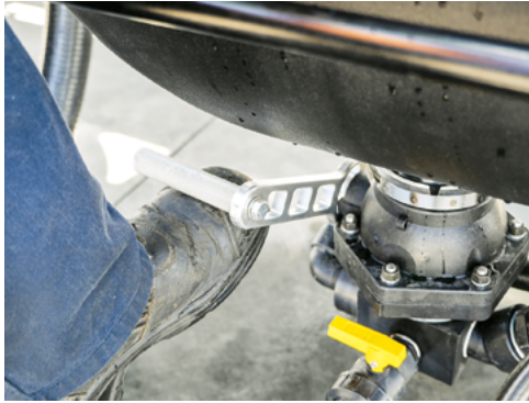
Lift-up to Close the foot operated ball valve at the bottom of the hopper.
