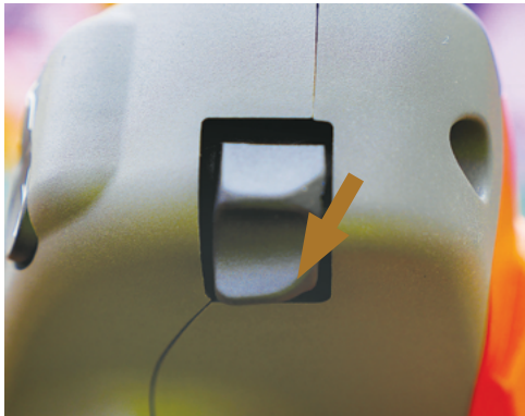
Press & hold Down the lower on the Dual Tilt rocker switch of the Joystick to lower the boom wings ends.
