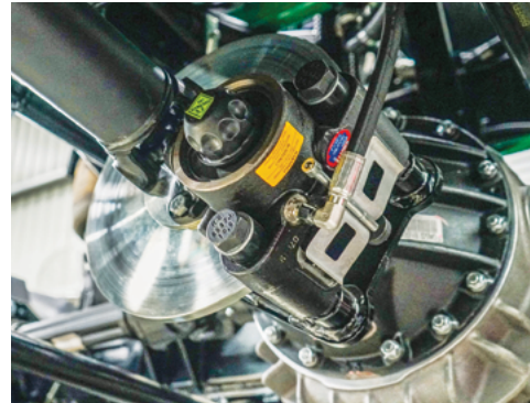
The Park Brake on the rear driveshaft.
