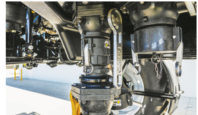
Connect a 3" fill hose to the 'Clean Fill' inlet & Open the 'Clean Fill' ball valves for filling & rinsing water.
