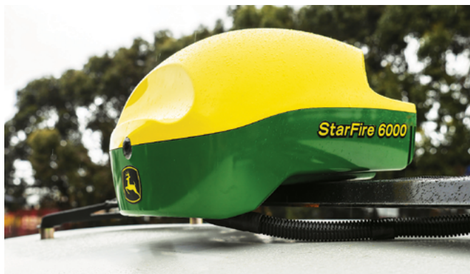
A dealer fitted John Deere Starfire GPS Receiver.
