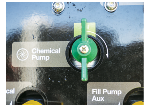
Turn the Chemical Pump valve ON.
