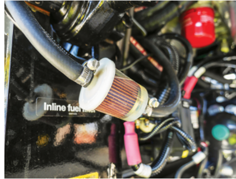
The Inline fuel filter located on the left hand side of the engine.
