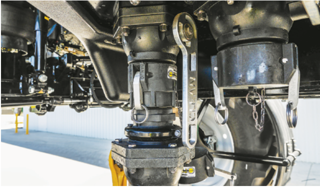
Connect a 3" fill hose to the 'Clean Fill' inlet & Open the 'Clean Fill' ball valves.
