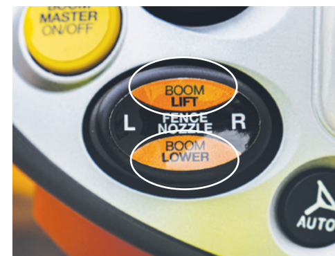
The Boom Lift & Boom Lower push button used to raise & lower the boom height as required.
