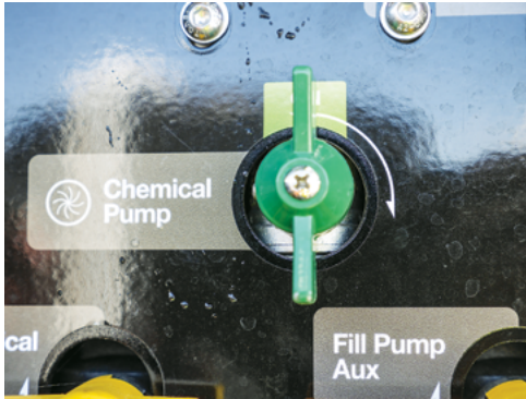
Turn the Chemical Pump valve ON.
