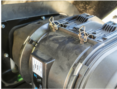
Release the cover clips on top of the air cleaner.
