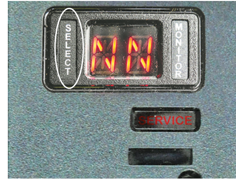
The 'Select' display flashes if restricted transmission shifting occurs. If so, consult a qualified technician.
