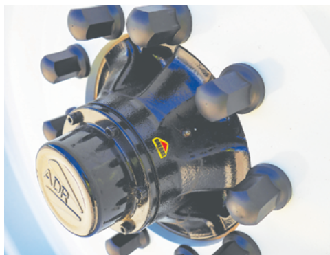
Recommended wheel nut torque tension is 350 ft/lb.
