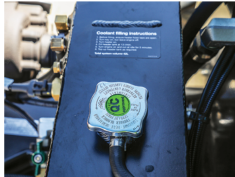
Regularly check the engine coolant level.
