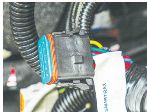
SMARTRAX connector - ISO BUS connection point.
