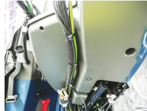
Lift up the Armrest console and release the G-Hub cable harness from underneath.
