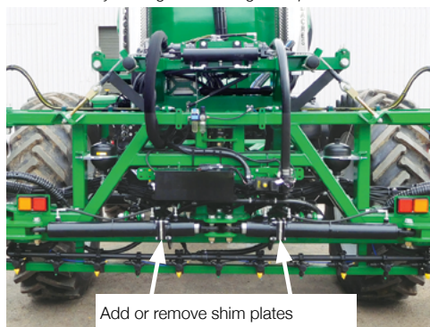
The first wing section 'Smiling Forward' adjustment is made by adding or removing shim plates.
