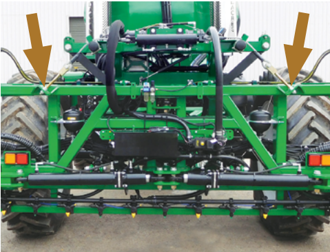
Boom Centre Level cable adjusters (shown on 48m boom).
