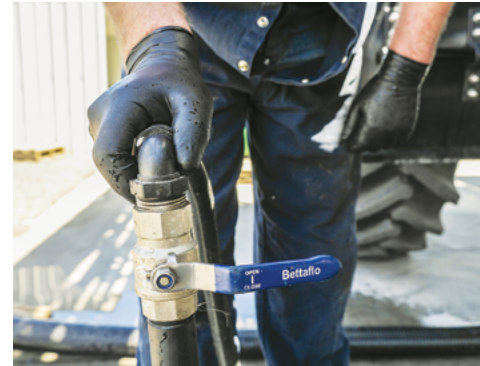
After the required amount of chemical has been transferred to the Hopper, close the Probe Valve.
