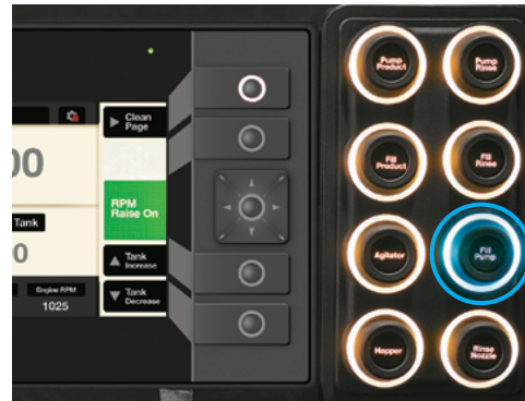
Press the 'Fill Pump' push button to pumping clean water.
