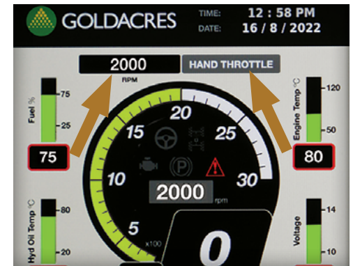
Home screen displaying Hand Throttle inactive & Engine rpm.
