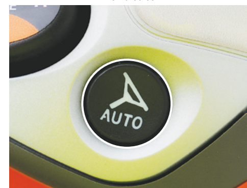
The Autosteer push button is used to engage & disengage the Autosteer.
