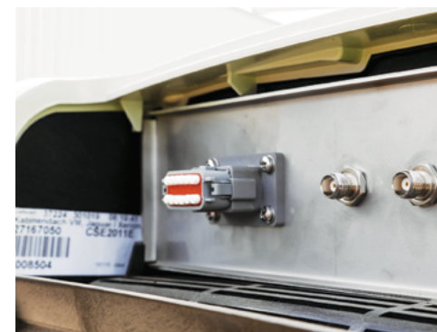
The cover removed showing the antenna connectors.
