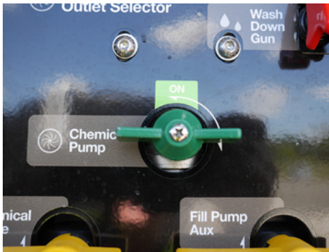
Rotate the Chemical Pump valve to Off position.
