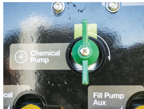
Turn the Chemical Pump valve ON.
