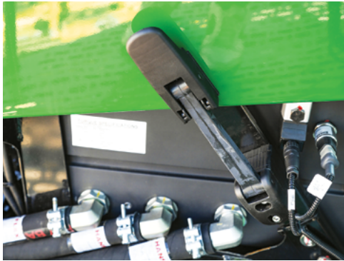
To open the bonnet unclip two latches, located on either side of the bonnet near the cabin.
