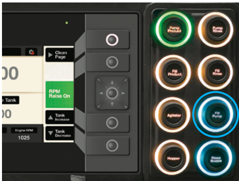
Press the 'Fill Pump' push button On.
