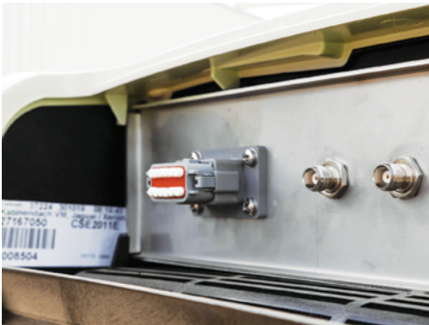
The cover removed showing the antenna connectors.
