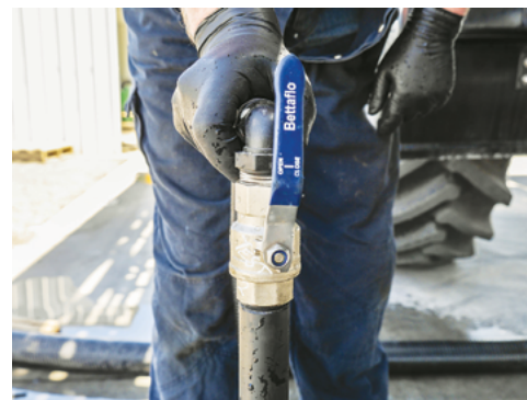
Place the Chemical Probe into the chemical & open the Probe Valve to transfer chemical to the Hopper.
