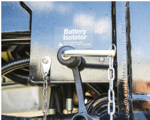
Disengage the Battery Isolator switch.
