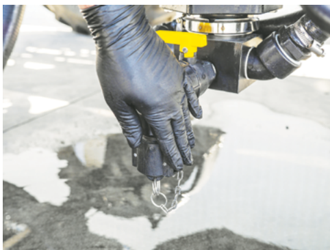
Disconnect the micromatic hose & refit the camlock coupling plug.
