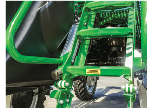
The pneumatic cylinder raises & lowers the Folding Ladder for cabin access.
