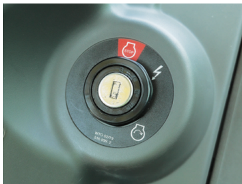
The Ignition Switch has 3 functions: Stop, On/Accessories (lightning symbol) & Engine Start (rotating arrow symbol).
