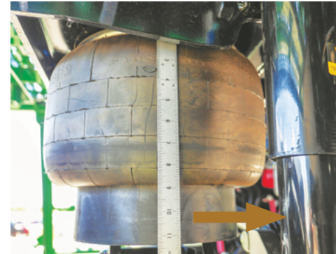
Air bag ride height measurement & shock absorber (right).
