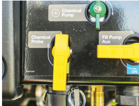
Rotate the Chemical Probe valve to On position.
