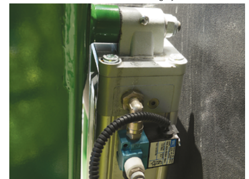
Air inlet of the ladder folding cylinder.
