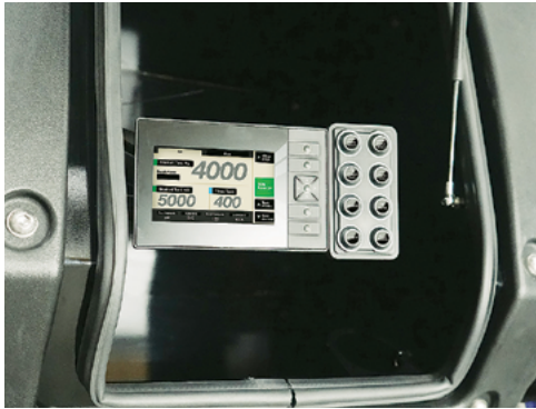
The external G-Hub Controller located in the storage cabinet of the Quick Filling Station.
