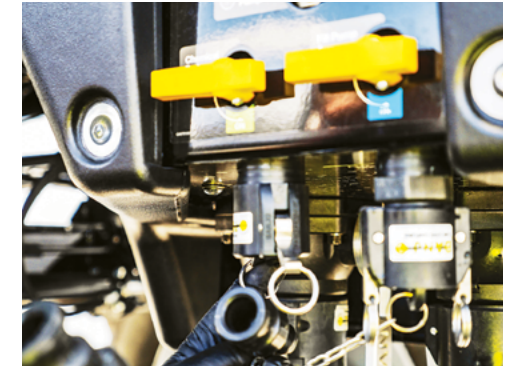
Disconnect the Chemical Probe hose & refit the camlock cap.
