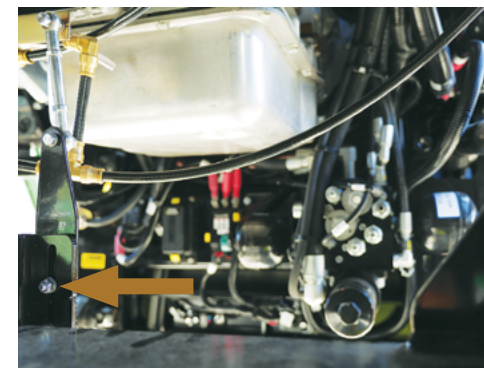
Loosen the bolt holding the adjustor plate & move the plate up or down to adjust the ride height, then retighten the bolt.
