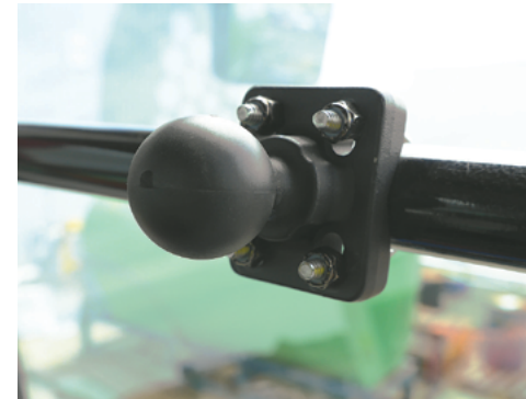
Ball mount fitted on the rail ready for the Autosteer Console.
