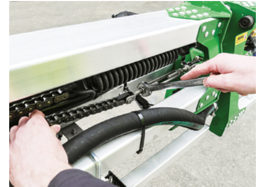
Adjust the turnbuckle to adjust spring tension as required.
