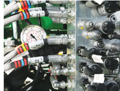
Pressure gauge located on the F2MAC Port (48m).
