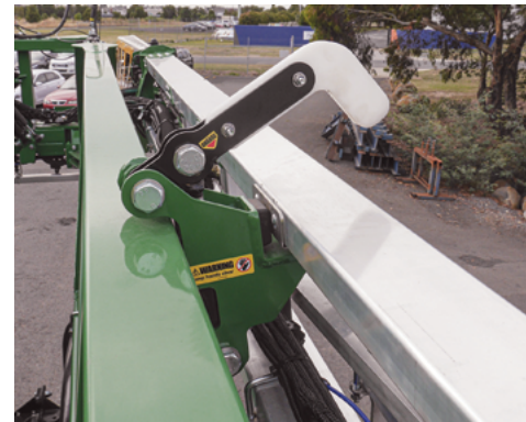
The left hand side Boom Rest lock unfolded - 32 & 36m booms only.
