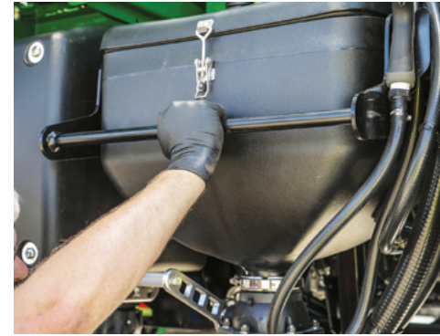
Pull the hopper down into its working position.
