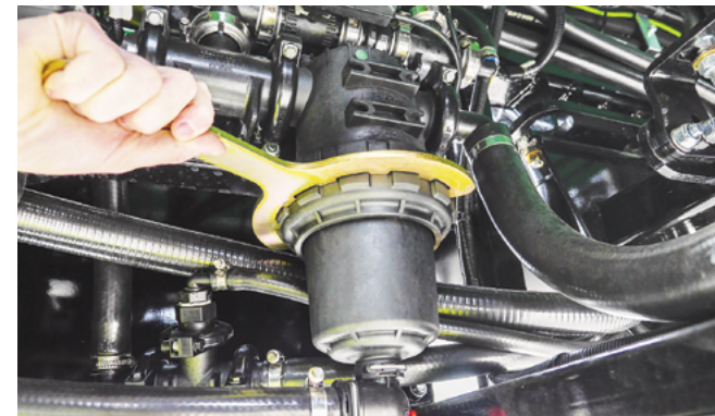
Loosen the pressure filter bowl nut slowly using the filter spanner supplied.
