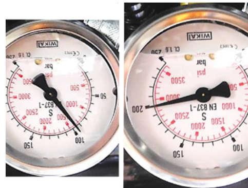
After the adjusting the screw until the gauge reads 200 Bar, pump the brake and the pressure will drop.
