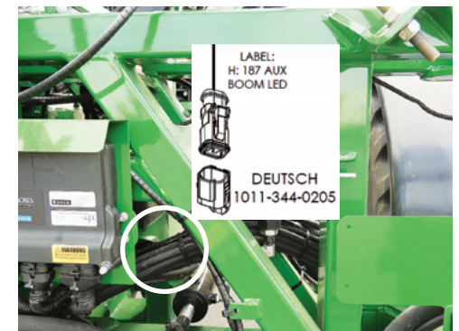
Auxiliary power connector located on a cable on the boom centre section (RHS shown [2 connectors - left & right side]).
