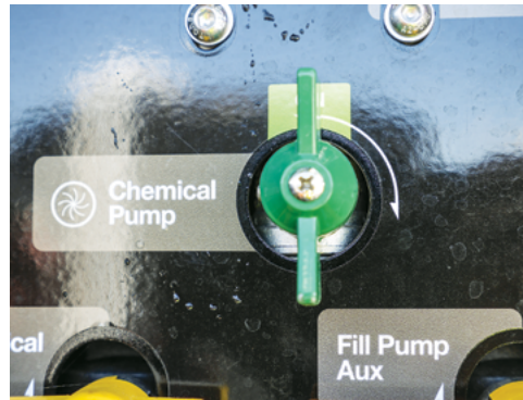
Turn the Chemical Pump valve On.
