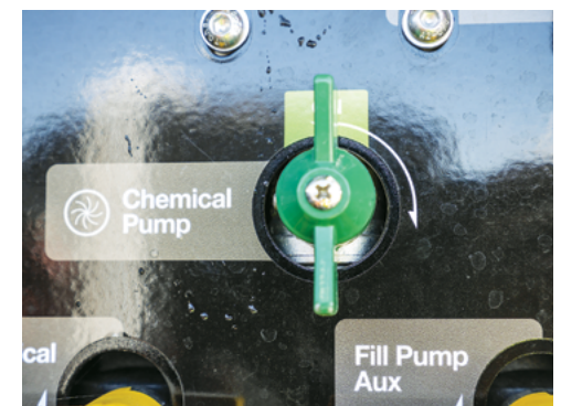
Turn the Chemical Pump valve ON.
