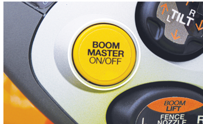
Press the 'Boom Master On/Off' push button on the Joystick to stop spraying.
