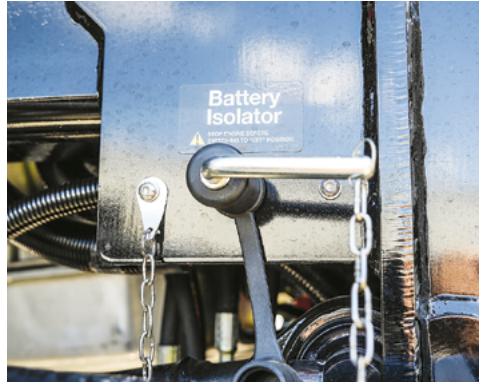
Disengage the Battery Isolator switch.
