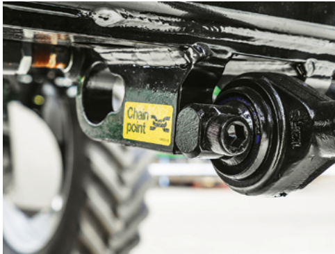
Front left tie-down attachment & towing point.
