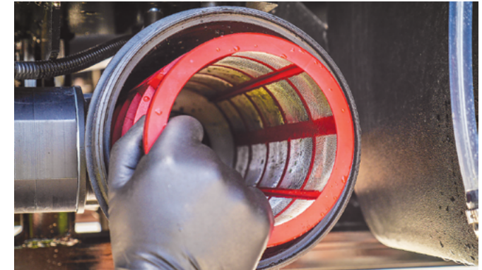
Remove the Suction Filter screen.
