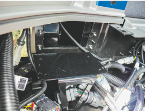
Mounting plate for a Trimble autosteer module at the back of the electrical compartment.
