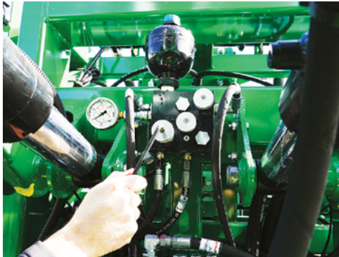
Loosen the locknut and adjust the pressure with the Pressure Reducing Valve (8) (24 to 42m booms).
