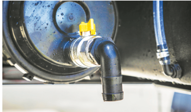
Open the drain valve to drain the Suction Filter.
