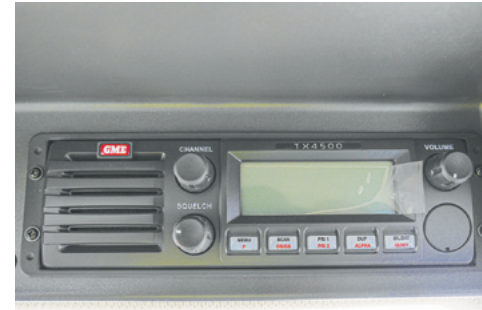
The UHF Two Way Radio located in the Overhead Console above & in front of the operator in the cabin.
