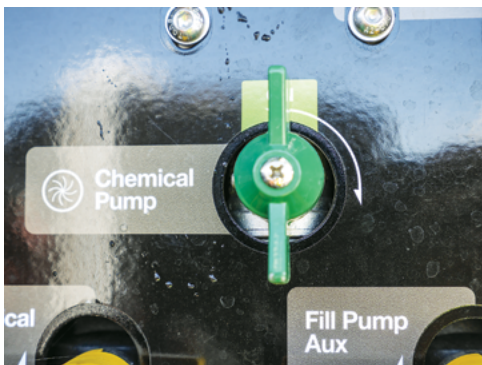
Turn the Chemical Pump valve On.
