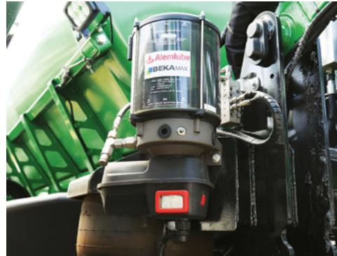
An Alemlube Auto-Greasing System centre (option).
