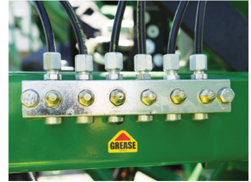
'Remote Grease Bank' with a 'Grease Decal' used to simplify greasing access.
