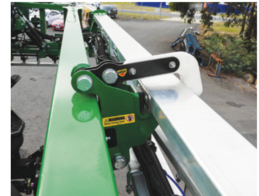
The left hand side Boom Rest lock folded - 32 & 36m booms only..
