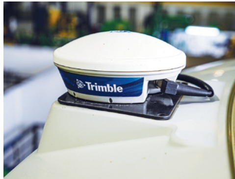
The Trimble antenna on the cabin roof magnetic plate.
