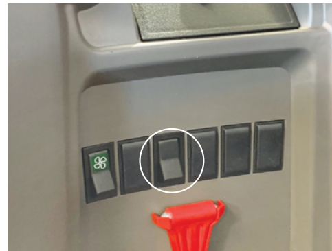
Press & Hold the Adjustable Axle Track In/Out Rocker Switch (on the cabin corner panel) as required while travelling forward at 10kph.
