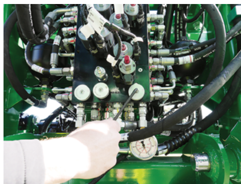
Wind out the Yaw valve B until fully open.
