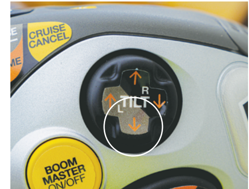
Press & hold the L Arrow Down part of the Boom Tilt push button to tilt down the left hand boom end.
