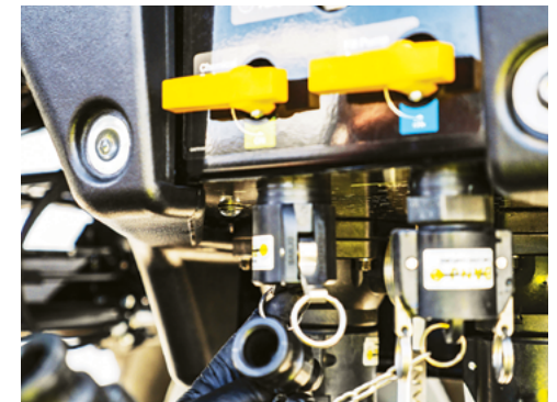
Disconnect the Micromatic hose from the Chemical Probe Inlet & refit the camlock cap.
