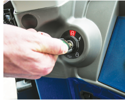
Turn the Ignition key to crank & start the engine.
