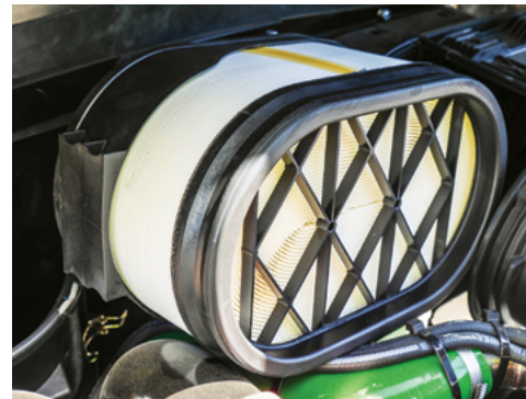
Fit a new primary air filter.
