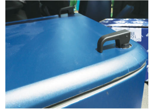
The electrical compartment cover refitted & locked into position.
