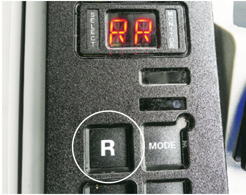
Press the 'R' push button to engage reverse gear for reversing the sprayer.
