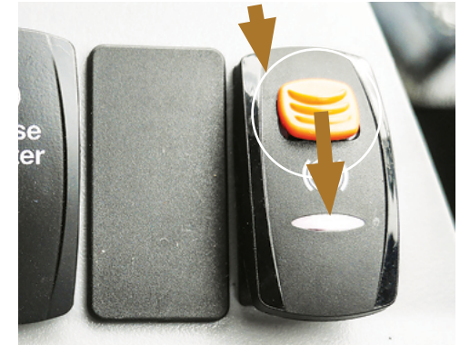
To engage the Park Brake (On), slide the orange lock rearward & press the switch Forward.
