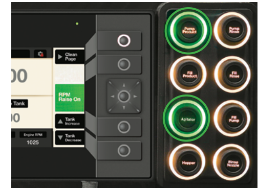
Press the 'Pump Product' push button On, then press the 'Agitator' push button to keep chemicals mixed.
