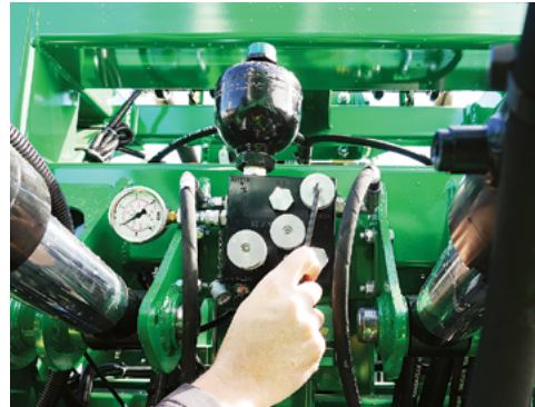
Loosen the locknut and adjust the breakaway return speed with the Breakaway Speed Valve (9).
