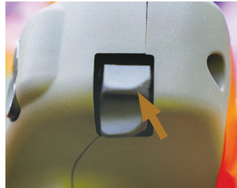
Press & hold Up the lower on the Dual Tilt rocker switch of the Joystick to raise the boom wings ends.
