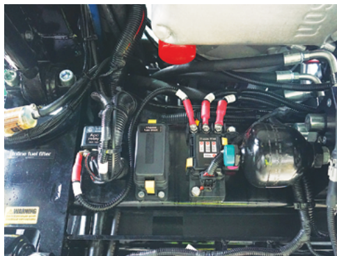
Chassis mounted ACC Relay, Fuse box & Chassis PDM.
