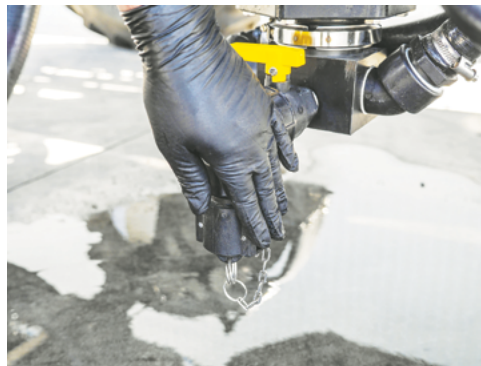
Refit the camlock coupling plug.
