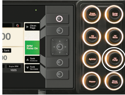
Press the 'Fill Pump' push button Off.
