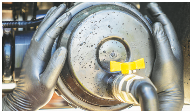
Unscrew the filter bowl collar to remove the filter bowl.
