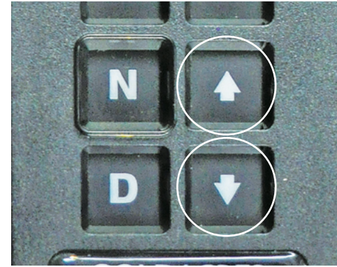
Press the Gear Up (Arrow up) or Gear Down (Arrow down) push button to manually change gears Up or Down.
