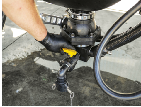
On completion of emptying the hopper, Close the Bottom Drain valve.
