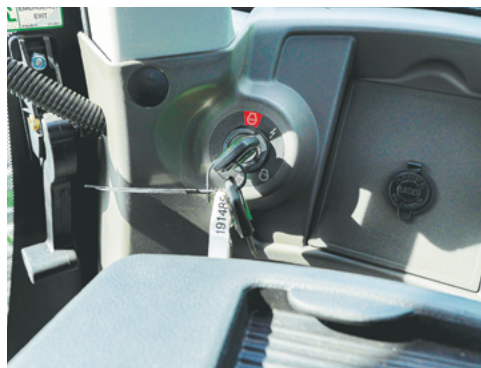
The Ignition Switch is located on the right hand side, rear corner console of the cabin.
