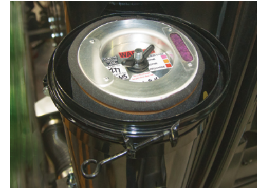
Unscrew the carbon filter retaining nut & remove the filter element from the filter housing.
