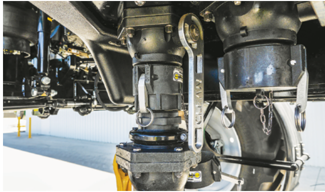
Connect a 3" fill hose to the 'Clean Fill' inlet & Open the 'Clean Fill' ball valves.
