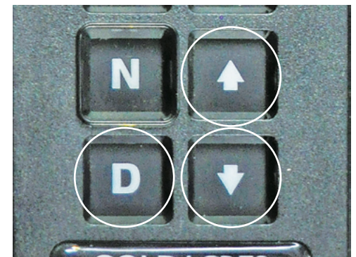
Press the 'D' switch to engage 1st gear. 1-6. Press the Arrow switches to change Up or Down (gears 1-6).
