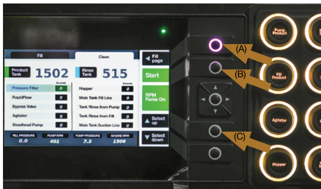
Press the Screen Selector push button (A) to select the 'Clean' screen, press the Select Up push button (C) to select Pressure Filter, then press the Start push button (B).
