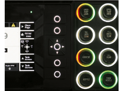
More colour light functions are in the Push Button Pad on the right of the External G-Hub screen
