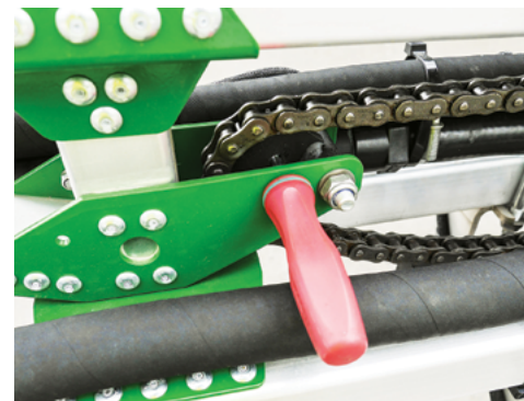
With the boom tip pulled back, place a pin through the holes to hold the sprocket to adjust the turnbuckle.
