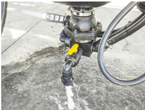
Remove the camlock coupling plug & Open the Bottom Drain valve.
