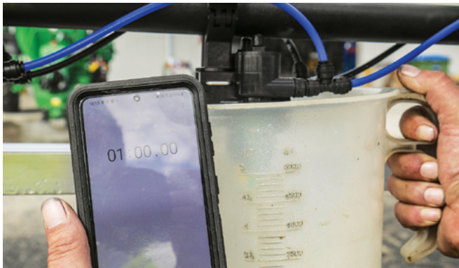
Place the measuring jug under one nozzle to collect nozzle output for exactly 1 minute, then remove it.
