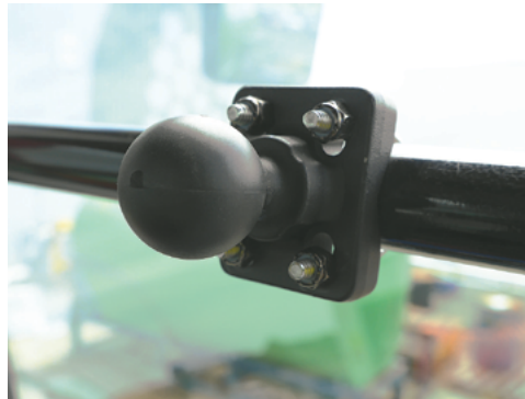
Ball mount fitted on the rail ready for the Autosteer Console.
