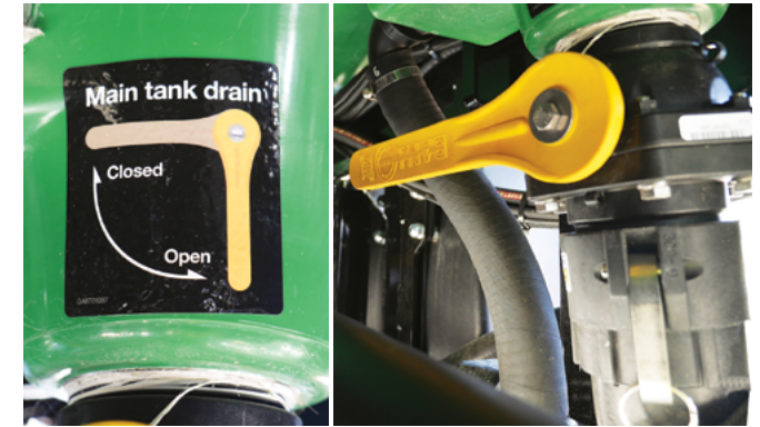
Open the Product Tank drain valve to drain the tank, then close the valve.
