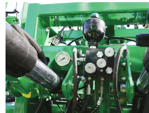
Remove the cap & attach a pressure gauge to the Gauge Test Port (4).
