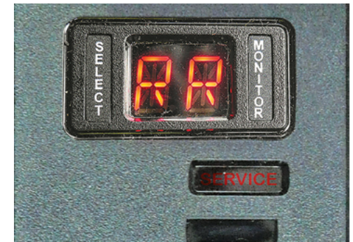
Select & Monitor displays showing Reverse gear.
