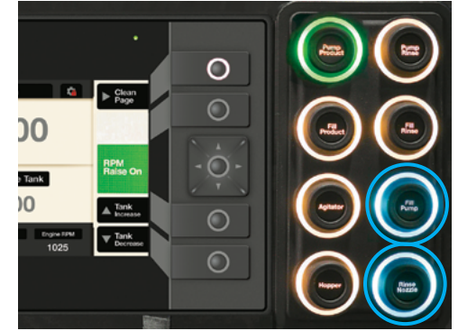
Ensure the 'Pump Product' push button is On, then press the 'Fill Pump' & 'Rinse Nozzle' push buttons On.
