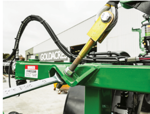
Make adjustment to the Boom Centre Level cable adjusters as required.
