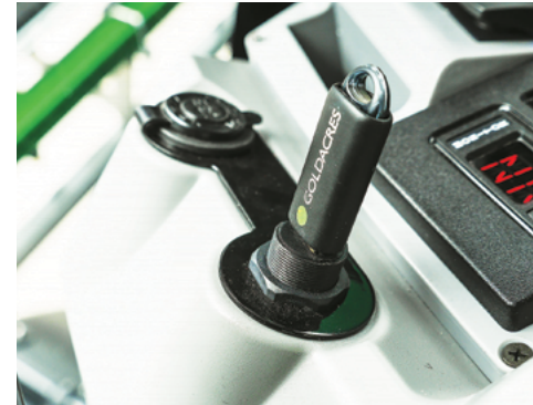
The Back-Up/Restore USB is provided to back-up & restore system settings & data.
