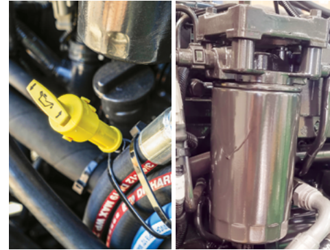
The Secondary fuel filter located on the left hand side above the engine oil dip stick.
