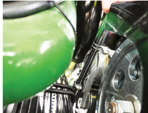
Use a breaker bar with a 1/2" socket to release the hydraulic pump belt tensioner.
