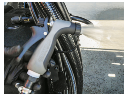
Point the Wash Down Gun & squeeze the trigger to spray.
