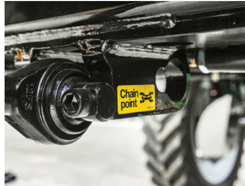
Front right tie-down attachment & towing point.
