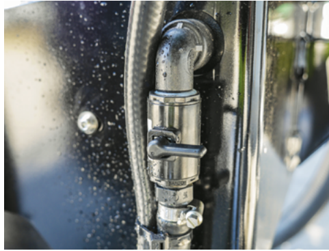
On completion of mixing, Close the Mixing Jet valve.
