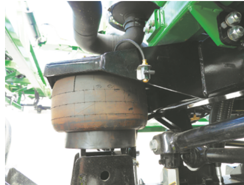
Air bag dump valve closed.
