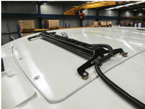
Fasten the Starfire Receiver mount onto the cabin roof.
