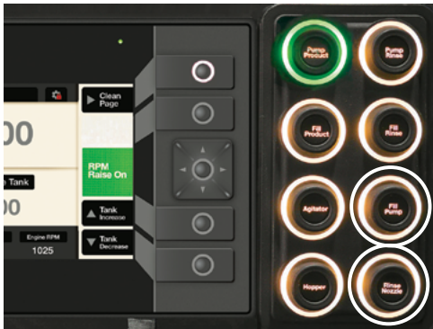
Press the 'Fill Pump' push button Off.
