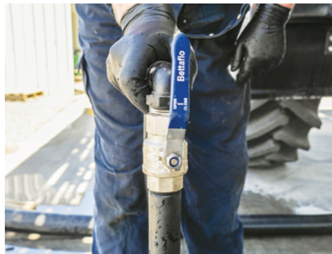
Place the Chemical Probe into the chemical & open the Probe Valve to transfer chemical to the Hopper.
