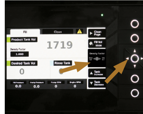
Press the Left or Right arrow touch buttons to Increase or Decrease the Density Factor by 0.001 increments.
