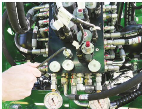
Adjust the Yaw Pressure with the Pressure Reducing Valve (24 to 42m booms).
