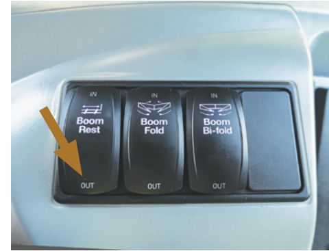
Press & hold down the Boom Rest OUT rocker switch to unlock the LHS boom rest
