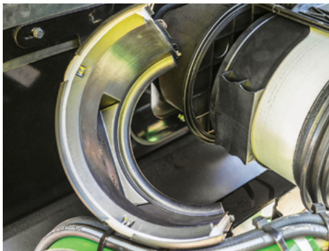
Remove the air cleaner cover, then remove the primary air filter.
