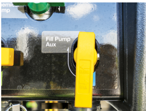
Rotate the 'Fill Pump Aux' valve to On position.
