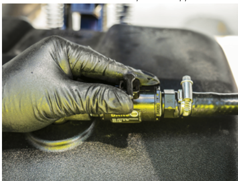
Close the Rinse Valve on top of the hopper lid.
