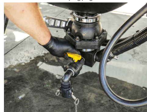
Close the Bottom Drain valve & remove the camlock coupling plug.
