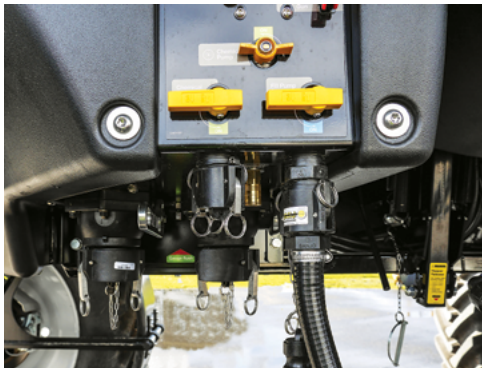
Connect a pressure hose to the 'Fill Pump Aux Valve' 1" camlock fitting.
