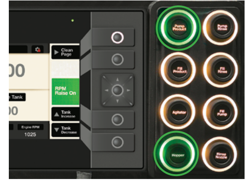
Press the 'Pump Product' push button On & the 'Hopper' push button On.
