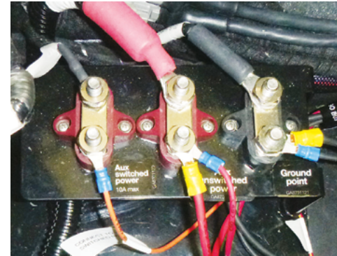
Labelled electrical terminals inside the Electrical Compartment.
