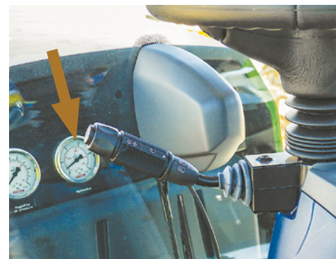
Oil pressure gauge of the closed centre pump.
