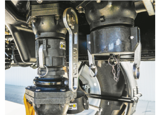
Connect a 3" fill hose to the 'Clean Fill' inlet & Open the 'Clean Fill' ball valves.
