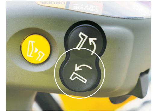
The lower Cruise Set/Decrease push button used to set the current ground speed for Cruise Control.
