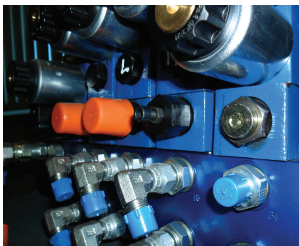
Above: Spool block shown with cap removed from flow control valve.
