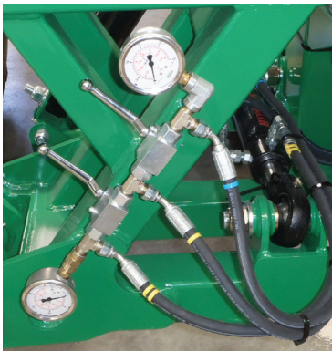
This picture shows the yaw charge ball valves in the "OPEN" position
