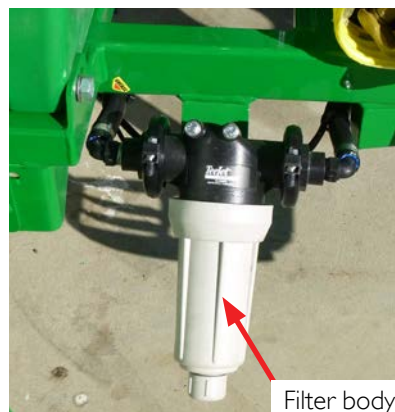
Above: In-line pressure filter located on right hand side chassis rail.
