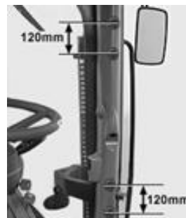
Above: Some tractors may have pre-drilled mounting holes on the pillar which can be used with the bracket GA4522930 to mount the rate control console.
