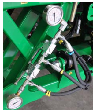
Left: Yaw charge ball valves in the CLOSED position.
