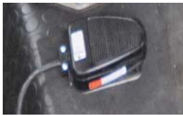
Above: Optional ISOBUS foot controller can be placed anywhere convenient on the cabin floor.
