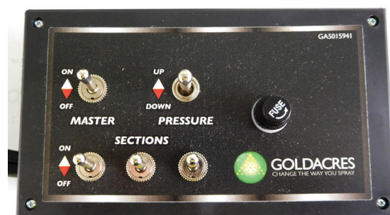
Above: In cab section control and pressure regulation control box and harness.
