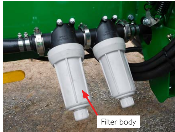
Above: Dual in-line pressure filters located on left hand side chassis rail next to the induction hopper mount.
