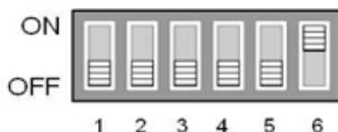
Figure 3: DIP Switch (SW1) setting. Note that all switches are in the OFF position except switch 6.
