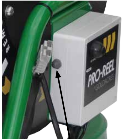
Current overload reset button
