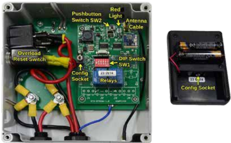
Figure 2: On the left is an inside view of the Pro-Reel® Control Box showing the parts relevant to setup. On the right is a view of the hand-held remote unit underside with the battery cover and battery pack removed, exposing the configuration socket.
