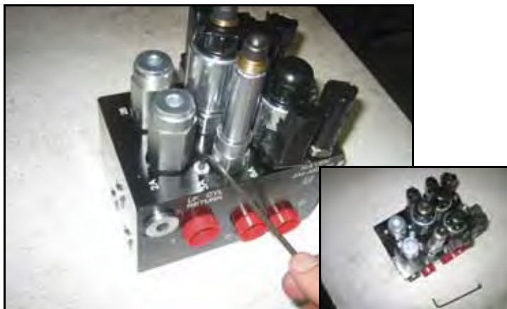
FIGURE 27. Port Plugs Removed from the AutoBoom Valve
