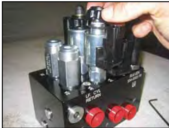
FIGURE 8. Coil Reinstalled on the AutoBoom Valve
