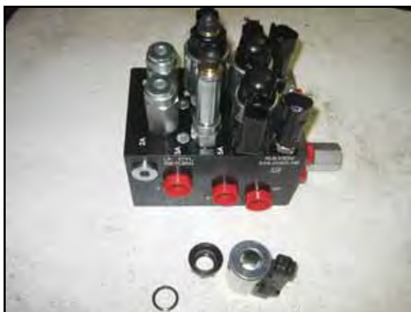
FIGURE 4. Coil Removed from the AutoBoom Valve
