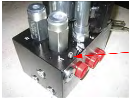
FIGURE 5. Orifice Fitting Removed from the AutoBoom Valve
