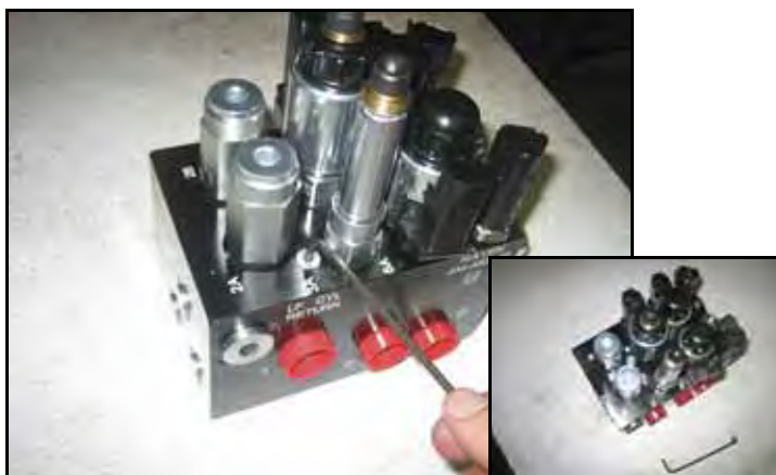
FIGURE 5. Port Plugs Removed from the AutoBoom Valve
