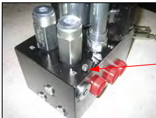
FIGURE 6. Orifice Fitting Removed from the AutoBoom Valve
