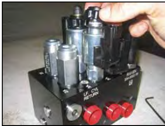
FIGURE 30. Coil Reinstalled on the AutoBoom Valve
