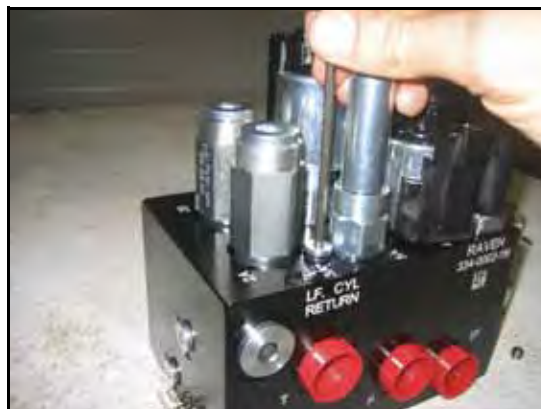
FIGURE 6. Port Plug Reinstalled on the AutoBoom Valve
