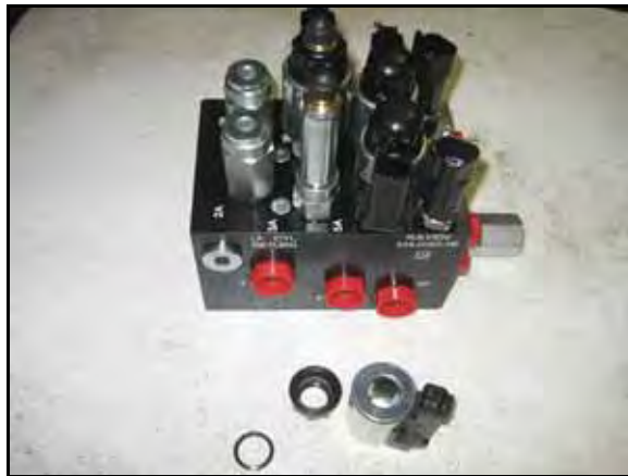
FIGURE 16. Coil Removed from the AutoBoom Valve
