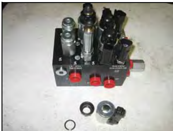
FIGURE 3. Coil Removed from the AutoBoom Valve
