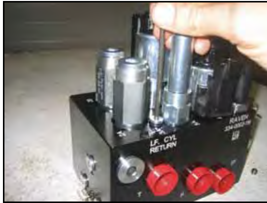
FIGURE 19. Port Plug Reinstalled on the AutoBoom Valve
