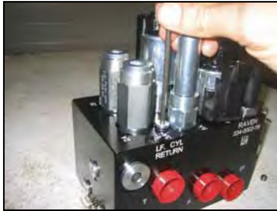
FIGURE 29. Port Plug Reinstalled on the AutoBoom Valve
