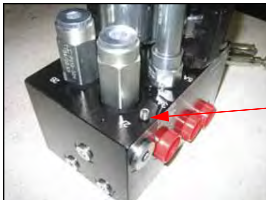
FIGURE 28. Orifice Fitting Removed from the AutoBoom Valve
