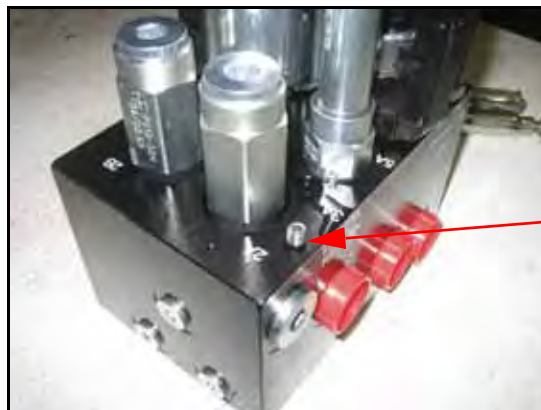
FIGURE 18. Orifice Fitting Removed from the AutoBoom Valve
