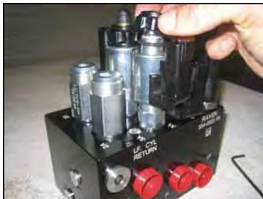
FIGURE 20. Coil Reinstalled on the AutoBoom Valve
