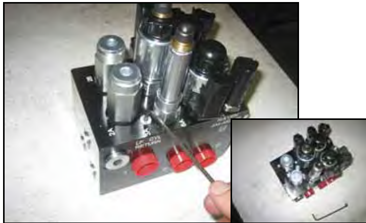
FIGURE 17. Port Plugs Removed from the AutoBoom Valve
