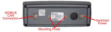
3. Connect the male, 4-pin Deutsch connector on the switch box cable to the 4-pin connector on the back of the switch box.
