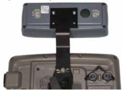
**Note:** The mounting bracket is designed to mount the switch box above the VT display. When looking at the back of the switch box and mounting bracket, the four pin connector and small part number label should be to the left of the mounting bracket flange.
