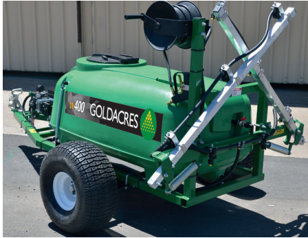
Figure 1: UV400 with 4 metre folding boom closed.
