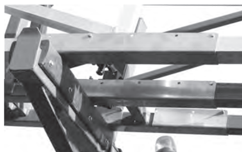
Correctly fitted boom protectors
