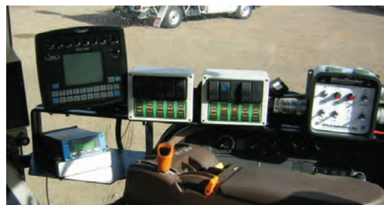
Example of consoles securely mounted in cabin (SCS4400 console and additional consoles shown as example only)
