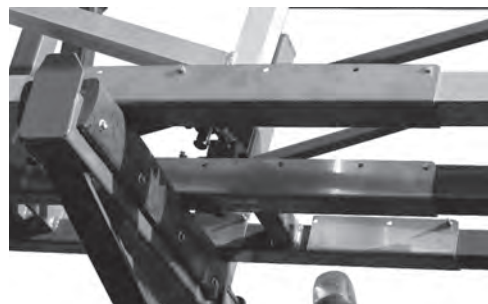
Correctly fitted boom protectors
