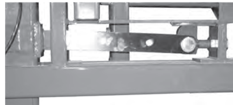
Fixed link in place of hydraulic cylinder
