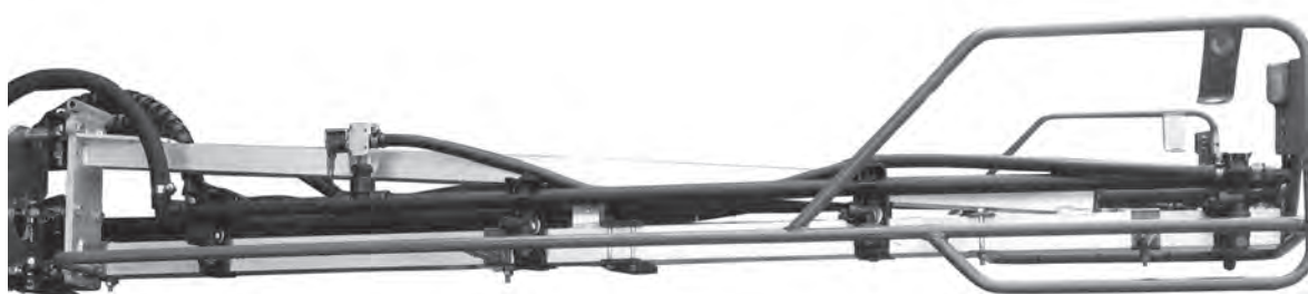
3D breakaway hinge with boom end protector fitted
