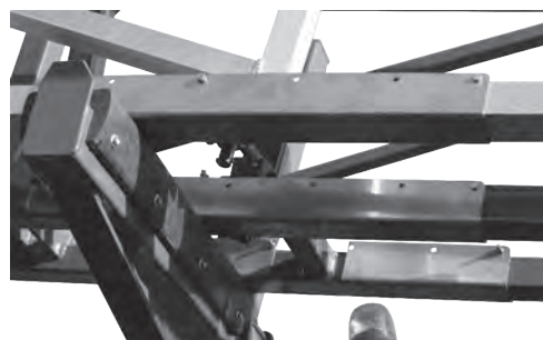
Correctly fitted boom protectors
