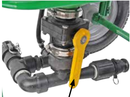
Hopper Ball Valve is shown in the open position, Vertical.
