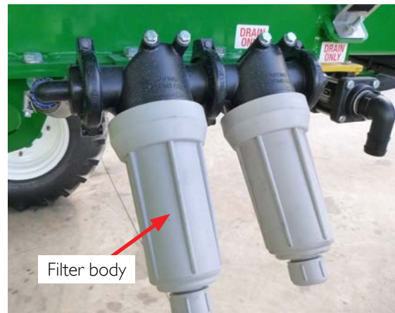
Above: Dual in-line pressure filters located on left hand side chassis rail next to the induction hopper mount.
