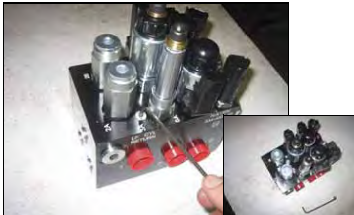
FIGURE 4. Port Plugs Removed from the AutoBoom Valve
